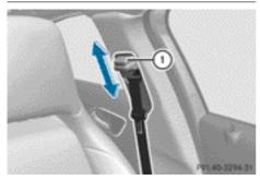
You can adjust the belt height for the front seats. Adjust the belt to a height that allows the upper part of the seat belt to be routed across the centre of your shoulder.
