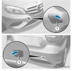
Remove the towing eye from the stowage space.
