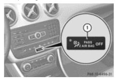
The sensor system for child restraint systems in the front-passenger seat detects whether a special Mercedes-Benz child seat with a transponder for automatic child seat recognition has been fitted. In this case, **Example 1** lights up. The front-passenger front airbag is disabled. If the front-passenger front airbag is disabled by the automatic child seat recognition, the following remain enabled on the front-passenger side:
