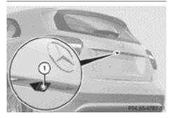
Reversing camera (1) is in the boot lid handle. The reversing camera extends, when it is activated.
