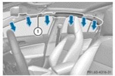
Windowbags ① enhance the level of protection for the head (but not chest or arms), of the vehicle occupants on the side of the vehicle on which the impact occurs.
