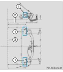
Example: anchorage points for the trailer tow hitch
