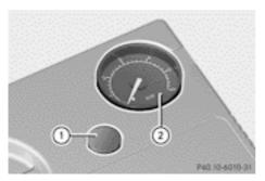
► To reduce the tyre pressure: depress pressure release button (1) next to pressure gauge (2).
