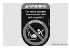
If the front-passenger seat of your vehicle does not have automatic child seat recognition, this is indicated by a special sticker. The sticker is affixed to the side of the dashboard on the front-passenger side. The sticker is visible when you open the front-passenger door.
