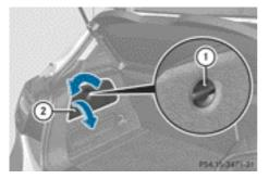
To open the cover: turn handle ① anticlockwise and fold down cover ② and remove it.
