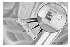
Install the ISOFIX child restraint system. Comply with the manufacturer's instructions when installing the ISOFIX child restraint system.
