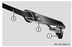
Top Tether provides an additional connection between the ISOFIX child restraint system secured with ISOFIX and the rear seat. It helps reduce the risk of injury even further.
