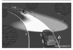
The active light function is a system that moves the headlamps according to the steering movements of the front wheels. In this way, relevant areas remain illuminated while driving. This allows you to recognise pedestrians, cyclists and animals.
