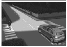
The cornering light function improves the illumination of the road over a wide angle in the direction you are turning, enabling better visibility in tight bends, for example. The cornering light function can only be activated when the dipped-beam headlamps are switched on.
