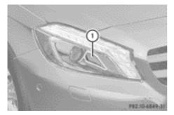
Vehicles with Intelligent Light System ① Cornering lamp: H7 55 W
