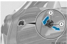
Press the ball coupling in the direction of the arrow until it engages behind the bumper.
