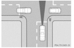
DISTRONIC PLUS may detect vehicles that are crossing your lane by mistake. Activating DISTRONIC PLUS at traffic lights with crossing traffic, for example, could cause your vehicle to pull away unintentionally.
