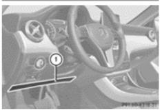
Driver's kneebag ① deploys under the steering column. The driver's kneebag is triggered together with the front airbag. The driver's kneebag is designed to operate together with the front airbag in frontal impacts if certain thresholds are exceeded. The driver's kneebag operates best in conjunction with correctly positioned and fastened seat belts. Driver's kneebag ① increases the driver's protection against:
