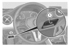
The electric parking brake carries out a function check at regular intervals when the engine is switched off. Noises that occur are normal.
