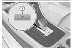
► When the vehicle is stationary, press P button ①.
