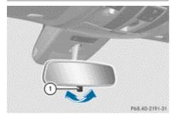
Anti-dazzle mode: pivot anti-dazzle switch ① forwards or back.
