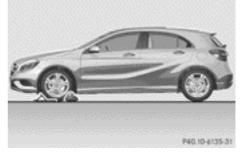
Securing the vehicle on level ground
