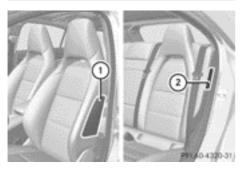
Front sidebags ① and rear sidebags ② deploy next to the outer seat cushions. When deployed, the sidebags offer additional protection of the thorax for occupants on the front seats as well as also of the pelvis for the vehicle occupants on the side of the vehicle on which the impact occurs. However, they do not protect the:
