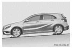
Securing the vehicle on slight downhill gradients
