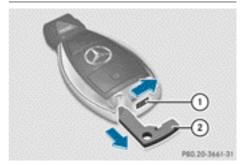
▶ Push release catch ① in the direction of the arrow and at the same time remove mechanical key ② from the SmartKey.
