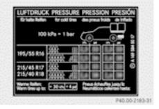
Example: tire pressure table with tire dimensions Some tire pressure tables show only the rim diameters instead of the full tire size, e.g. **R18**. Rim diameter is part of the tire size and can be found on the tire sidewall (⊳ page 313).
