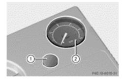
➤ To reduce the tire pressure: depress pressure release button ① next to pressure gauge ②.
