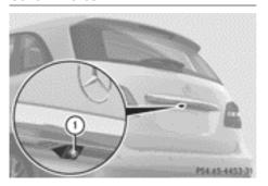
Rear view camera ① is in the trunk lid handle. The rear view camera extends, when it is activated.
