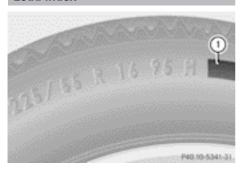
In addition to the load bearing index, load index ① may be imprinted after the letters that identify speed index  $\textcircled{6}(\triangleright \text{ page 313})$  on the sidewall of the tire.
