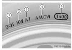
Canadian tire regulations prescribe that every new tire manufacturer or retreader has to imprint a TIN in or on the sidewall of each tire produced. The TIN is a unique identification number. The TIN makes it easier for tire manufacturers or retreaders to notify customers of recalls or other safety-related matters. It makes it possible for the purchaser to easily identify the affected tires.
