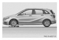
Securing the vehicle on level ground
