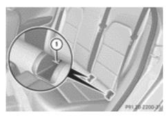
► Install the LATCH-type (ISOFIX) child restraint system. Comply with the manufacturer's instructions when installing the LATCH-type (ISOFIX) child restraint system.
