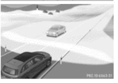
The extended range fog lamps reduce the glare experienced by the driver and improve the illumination of the edge of the road.
