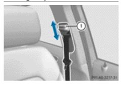
You can adjust the seat belt height on the front seats. Adjust the belt to a height that allows the upper part of the seat belt to be routed across the center of your shoulder.
