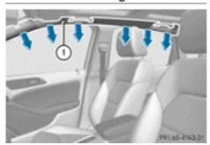
Window curtain air bags (1) enhance the level of protection for the head, but not chest or arms, of the vehicle occupants on the side of the vehicle on which the impact occurs.
