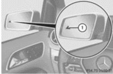
① Yellow indicator lamp/red warning lamp When Blind Spot Assist is activated, indicator lamp ① in the exterior mirrors lights up yellow at speeds of up to 20 mph (30 km/h).
