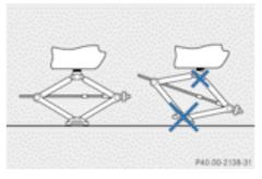
► Make sure the foot of the jack is directly beneath the jacking point.
