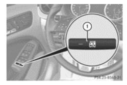
► To activate/deactivate: press button ①. If indicator lamp is lit, operation of the rear side windows is disabled. Operation is only possible using the switches in the driver's door. If the indicator lamp is off, operation is possible using the switches in the rear compartment.
