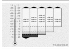
Viscosity describes the flow characteristics of a fluid. If an engine oil has a high viscosity, this means that it is thick; a low viscosity means that it is thin.
