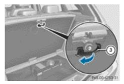
► Fold out hook ③ on the underside of the cargo compartment floor.
