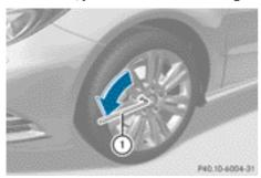
► Using lug wrench ①, loosen the bolts on the wheel you wish to change by about one full turn. Do not unscrew the bolts completely.
