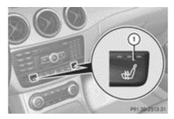
The three red indicator lamps in the button indicate the heating level you have selected. The system automatically switches down from level 3 to level 2 after approximately
