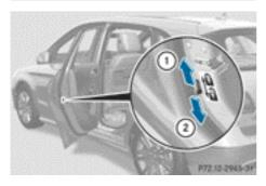
You can secure each door individually with the child-proof locks on the rear doors. A door secured with a child-proof lock cannot be opened from inside the vehicle. When the vehicle is unlocked, the door can be opened from the outside.
