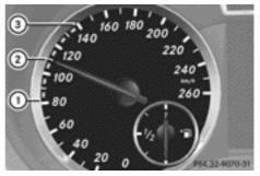
DISTRONIC PLUS displays in the speedometer
