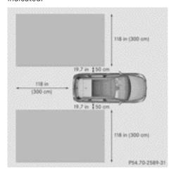
Blind Spot Assist monitors the area up to 10 ft (3.0 m) behind your vehicle and directly next to your vehicle, as shown in the diagram.
