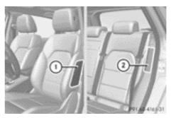
Front side impact air bags (1) and rear side impact air bags (2) deploy next to the outer seat cushions.
