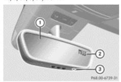
To receive a correct display in rear-view mirror ①, the compass must be calibrated and the magnetic field zone set.
