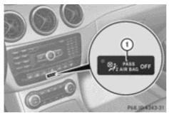
The sensor system for the air bag deactivation system detects whether a special Mercedes-Benz child seat with a transponder for the air bag deactivation system has been installed. In this case, [2] [2005] indicator lamp 1 lights up. The front-passenger front air bag is deactivated:
