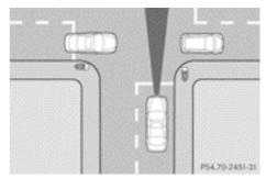
DISTRONIC PLUS may detect vehicles that are crossing your lane by mistake. Activating DISTRONIC PLUS at traffic lights with crossing traffic, for example, could cause your vehicle to pull away unintentionally.
