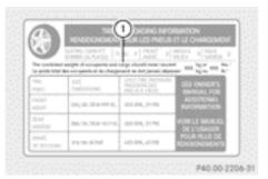
► Specification for maximum gross vehicle weight ① is listed in the Tire and Loading Information placard: "The combined weight of occupants and cargo should never exceed XXX kilograms or XXX lbs."
