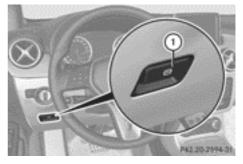
The electric parking brake performs a function test at regular intervals while the engine is switched off. The sounds that can be heard while this is occurring are normal.
