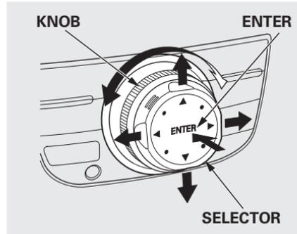
The knob turns left and right. Use it to make selections or adjustments to a list or menu on the screen.
