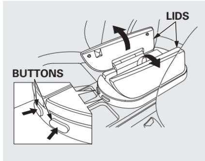
Your vehicle is equipped with a front seat armrest pad that is also a console compartment. To open the console compartment fully, push both buttons at the front of the compartment.
