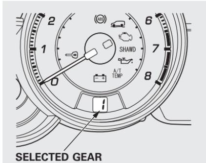
With the shift lever in “D” position, you can select the Sequential SportShift mode to shift gears much like a manual transmission, but without a clutch pedal.
