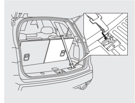
3. Route the tether strap over the head restraint, then attach the tether strap hook to the anchor, making sure the strap is not twisted.
