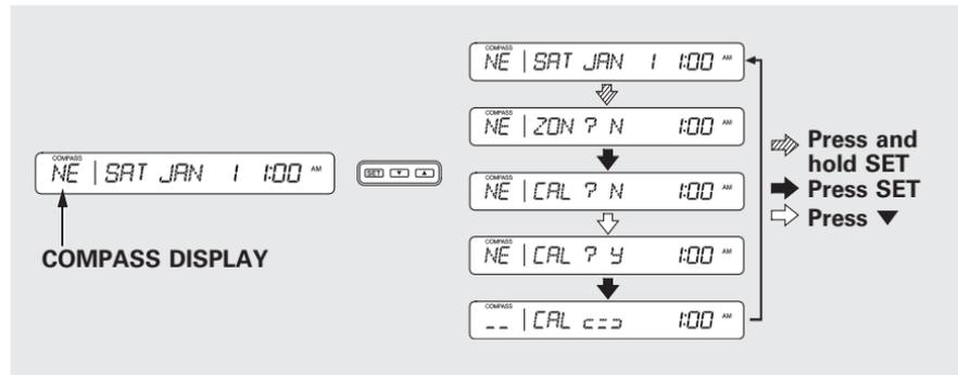
1. Press and hold the SET button for five seconds until the clock display changes to “ZON ? N.” (Clock adjustment mode will be started after the first two seconds.)
