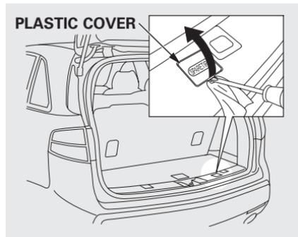
7. The spare tire is stored underneath the rear cargo area. Remove the plastic cover on the cargo area lining to access the shaft for the spare tire hoist.
