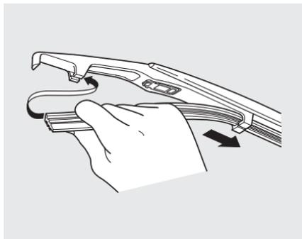
4. Slide the new blade into the wiper arm. Make sure it is engaged in the slot along its full length.
