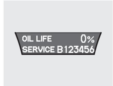
Press the SEL/RESET button on the steering wheel repeatedly to select the engine oil life. The message “SERVICE”, along with “0%”, and the maintenance item code are displayed on the lower part of the multi-information display when the calculated engine oil life is 0 – 1%.
