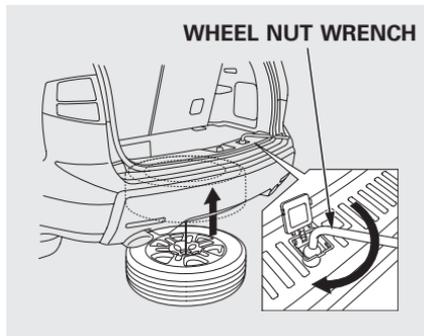
22. Slowly turn the wheel nut wrench clockwise to take up the slack of the hoist cable. Make sure the bracket is seated in the center hole of the flat tire.
