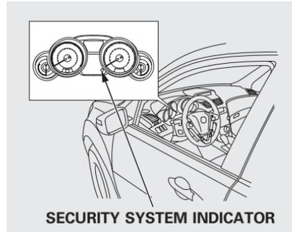
Once the security system is set, opening any door, the tailgate, or the hood without using the key or the remote transmitter, will cause it to alarm. It also alarms if the radio is removed from the dashboard or the wiring is cut.
