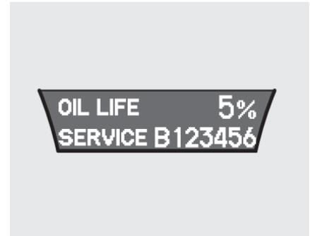
Press the SEL/RESET button on the steering wheel repeatedly to select the engine oil life. The message “SERVICE”, along with “5%”, and the maintenance item code are displayed on the lower part of the multi-information display when the calculated engine oil life is 1 – 5 percent (see page 383).
