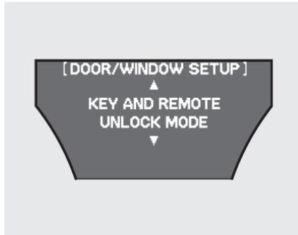
To select whether the driver's door unlocks or all the doors unlock when you unlock the doors with the remote transmitter, follow these instructions.
