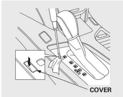
3. Put a cloth on the edge of the shift lock release slot cover. Use a small flat-tipped screwdriver or metal fingernail file to carefully pry up the edge of the cover and remove it from the slot.
