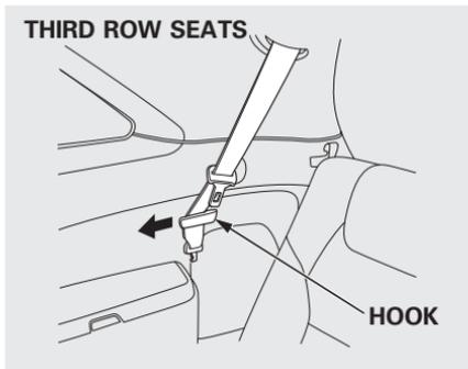
Pull out the outer shoulder belts from the hook. Both of the third-row hooks should only be used when the seat belt is detached.
