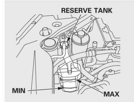
Look at the coolant level in the radiator reserve tank. Make sure it is between the MAX and MIN lines. If it is below the MIN line, see **Adding Engine Coolant** on page [396](#) for information on adding the proper coolant.
