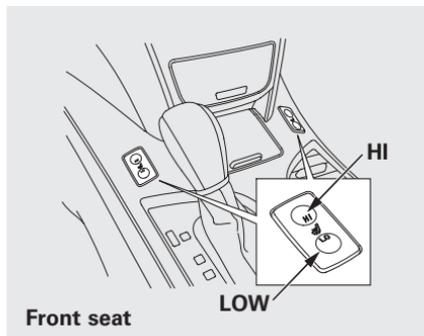
Push the front of the switch, HI, to rapidly heat up the seat. After the seat reaches a comfortable temperature, select LO by pushing the back of the switch. This will keep the seat warm.
