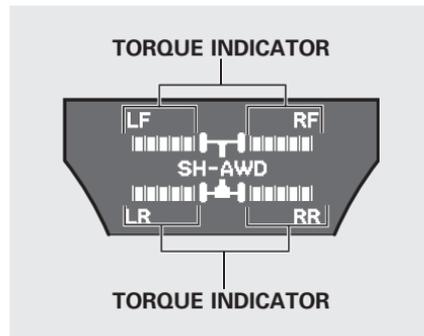
The SH-AWD torque distribution monitor on the multi-information display shows you the amount of torque being sent to the wheels. Each wheel: right front (RF), left front (LF), right rear (RR), and left rear (LR), has its own torque indicator.
