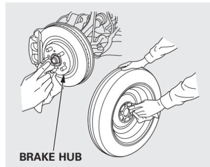
15. Before mounting the spare tire, wipe any dirt off the mounting surface of the wheel and hub with a clean cloth. Wipe the hub carefully; it may be hot from driving.
