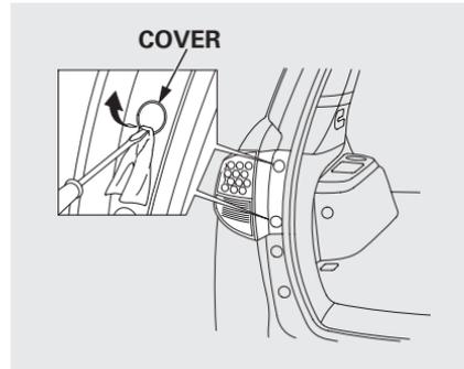
1. Open the tailgate. Use a flat-tip screwdriver protected with a cloth to pry open the two covers.
