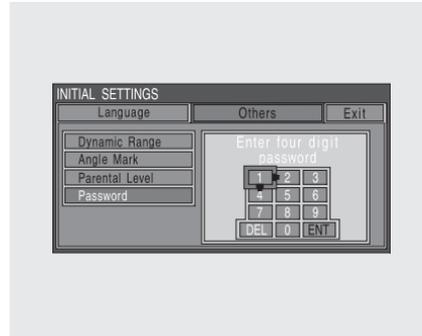
Select the first digit by pressing the ▼, ▲, ►, or ◀ button, and enter it by pressing the ENT button. Repeat this until all four digits are entered. When you enter the fourth number, the cursor automatically moves to “ENT” on the display. Press the ENT button on the control panel.
