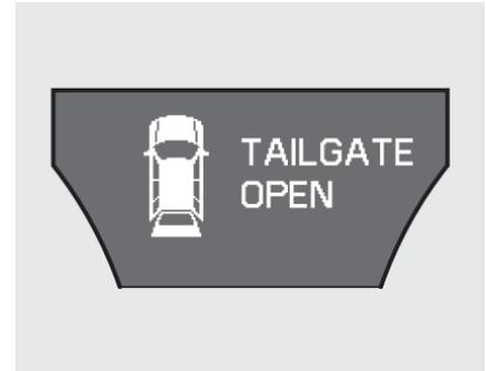
When the tailgate is not tightly closed, the “TAILGATE OPEN” message will come on.
