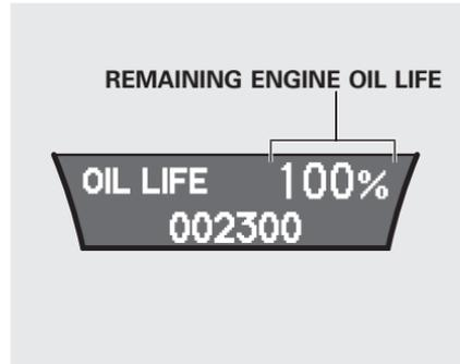
To see the remaining engine oil life displayed on the multi-information display as a percentage, turn the ignition switch to the ON (II) position. Make sure the display shows blank, SH-AWD and tire pressure, and then press the SEL/RESET button on the steering wheel repeatedly until the engine oil life appears (see page 73).
