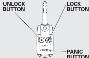
**LOCK** – Press this button once to lock all doors and the tailgate. Some exterior lights will flash. When you push **LOCK** twice within 5 seconds, you will hear a beep to verify that the doors and tailgate are locked and the security system has set. This button does not work if any door or tailgate is not fully closed.
