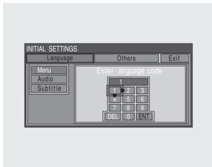
If you select “Yes,” the display changes to the language code input mode. Select the first digit using the ▼, ▲, ►, or ◀ button, and press the ENT button to enter it. Repeat this until all four digits are filled. When the fourth digit is entered, the cursor automatically moves to “ENT” on the display. Press the ENT button on the control panel to enter the new language code.
