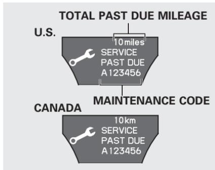
If the indicated required service is not done and the remaining engine oil life becomes 0%, the multi-information display will show a “SERVICE PAST DUE” message, the total mileage after the remaining oil life became 0%, and the maintenance item code(s).
