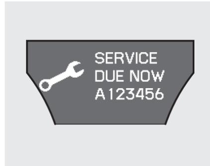
When the remaining oil life is 1 to 5 percent, the multi-information display shows a “SERVICE DUE NOW” message with the same maintenance items “SERVICE DUE SOON” was displayed with. When you see this message have the indicated maintenance performed as soon as possible.
