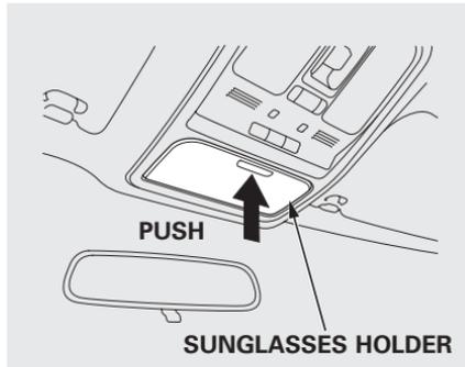
To open the sunglasses holder, push then release the raised detent. It will unlatch and swing down. To close it, push it until it latches. Make sure the holder is closed while you are driving.
