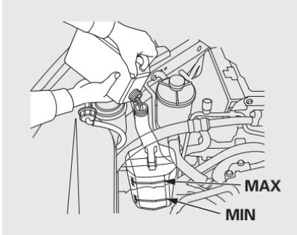
If the coolant level in the reserve tank is at or below the MIN line, add coolant to bring it up to the MAX line. Inspect the cooling system for leaks.
