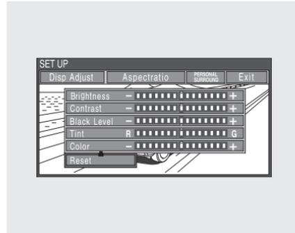
If you want to set the display to the default setting, select “Reset” by pressing the ▲ or ▼ button, and, then pressing the ENT button.
