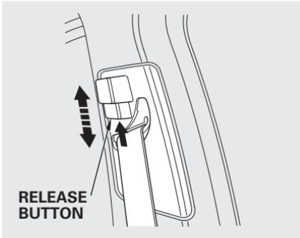
The front seats have adjustable seat belt anchors. To adjust the height of an anchor, squeeze the release button and slide the anchor up or down as needed (it has four positions).
