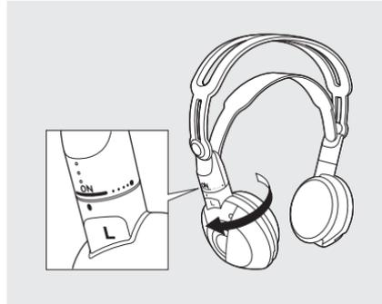
The audio for the rear entertainment system is sent to the wireless headphones that come with the system. When using the headphones, make sure you wear them correctly: L (left) and R (right) are marked on the sides of the frame. Wearing the headphones backwards may affect audio reception, limiting the sound quality and range.
