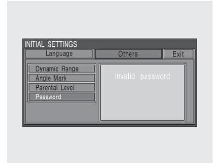
If the system does not recognize the password you entered, you will see the above display. Repeat the password setting steps until you enter the correct password.
