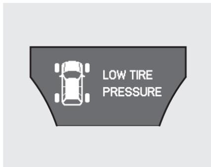
If any of the tires has low pressure, the tire pressure monitor also shows the above message to warn you about the low tire pressure when you select the display by pressing the INFO button several times. Following this display, press the SEL/RESET button to see each tire pressure. When you continue driving after installing the spare tire, you will also see this message on the multi-information display.
