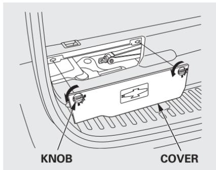
5. The tools and jack are under the cargo area behind a cover on the driver's side. Remove the cover by turning the knobs counterclockwise, then pulling out the cover.
