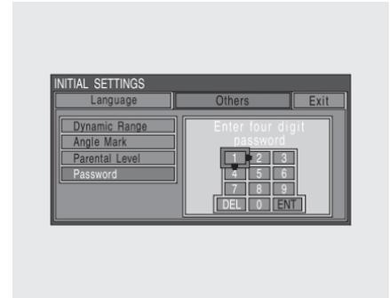
When you select and enter “Yes,” the display changes as shown above. To change the level, you need to enter your four digit password. Select the number for the first digit by pressing the ▼, ▲, ►, or ◀ button, and enter it by pressing the ENT button. Repeat this until all four digits are filled. When you enter the fourth number, the cursor automatically moves to “ENT” on the display. Press the ENT button on the control panel.
