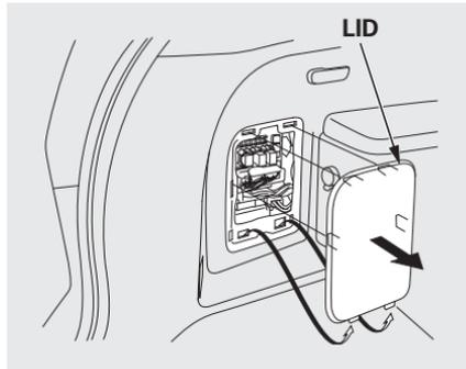
If the fuel fill door release button does not work, use the release lever inside the rear fuse box lid in the cargo area.
