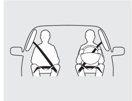
In addition, your vehicle has side curtain airbags to help protect the heads of the driver, front passenger, and passengers in the outer rear seating positions during a moderate to severe side impact or rollover (see page 32 for more information on how your side curtain airbags work).
