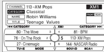
To listen to XM satellite radio, turn the ignition switch to the ACCESSORY (I) or ON (II) position. Push the power/volume knob to turn on the audio system, and press the «>» button. The last channel you listened to will show in the display. Adjust the volume by turning the power/volume knob.
