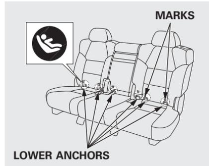
When you install a child seat in rear seating position, use the lower anchors as shown in the illustration. You can install up to three child seats at a time with LATCH.
