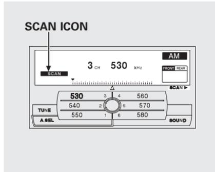
**SCAN** – The SCAN function samples all stations with strong signals on the selected band. To activate it, press the SCAN button, then release it.
