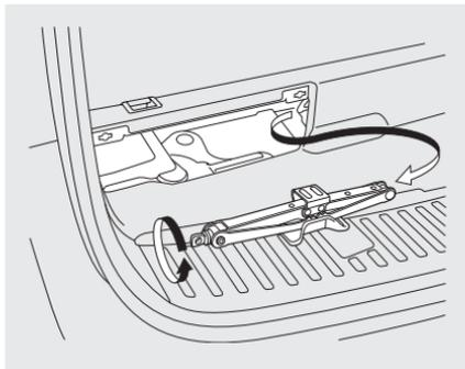
6. Turn the jack's end bracket counterclockwise to loosen it, then remove the jack.
