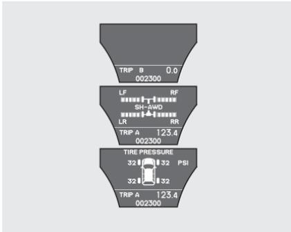
When the main menu is blank, SH-AWD or TIRE PRESSURE, pressing the SEL/RESET button changes the display to “trip meter/odometer” “outside temperature/odometer” and “engine oil life/odometer”.
