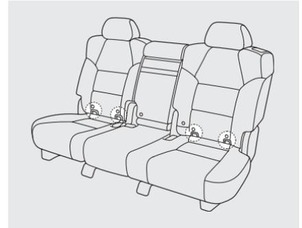
To install a LATCH-compatible child seat in either outer second row seat:
