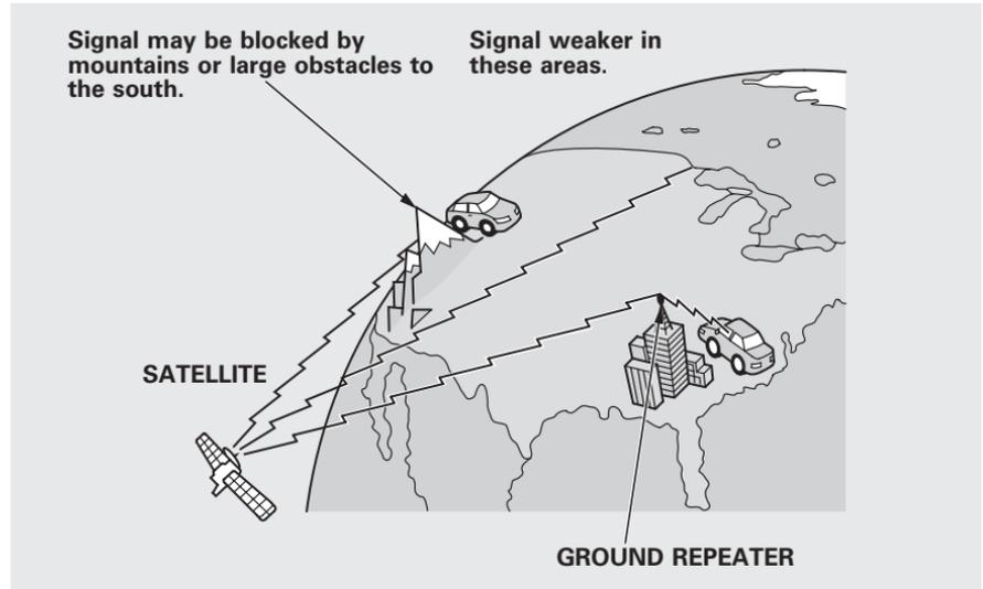
The XM satellites are in orbit over the equator; therefore, objects south of the vehicle may cause satellite reception interruptions. To help compensate for this, ground-based repeaters are placed in major metropolitan areas.
