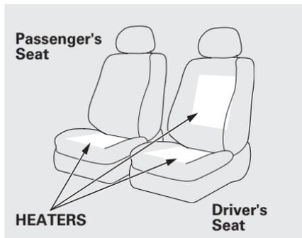
Both front seats are equipped with seat heaters. Because of the sensors for the side airbag cutoff system, there is no heater in the passenger's seat-back. The ignition switch must be in the ON (II) position to use the heaters.
