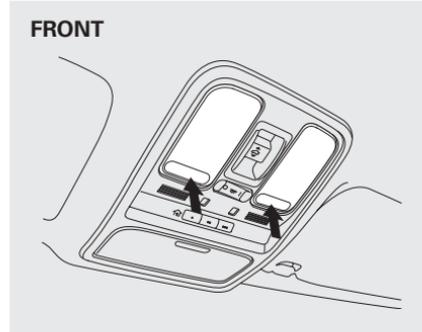
Turn on the front row individual map lights by pushing the lens. Push the lens again to turn it off. With the light control switch in the door activated position, the second row map lights can be turned on by pushing the lens. Push the lens again to turn it off.
