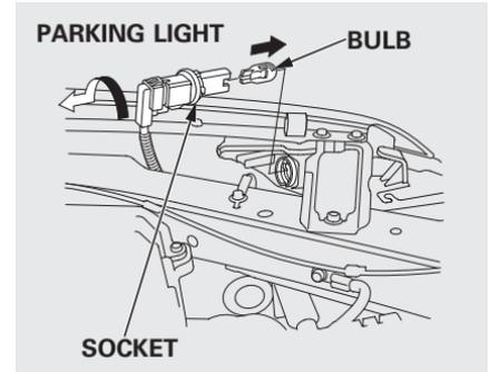
5. Push the new bulb straight into the socket until it bottoms.
