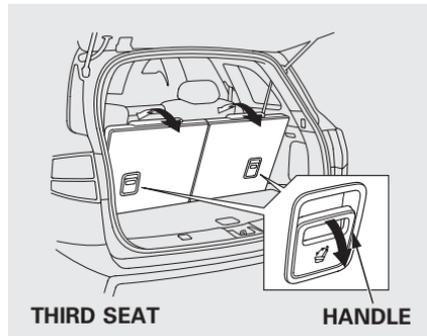
3. Unlock the seat-back by pulling the handle. Push the seat-back forward.
