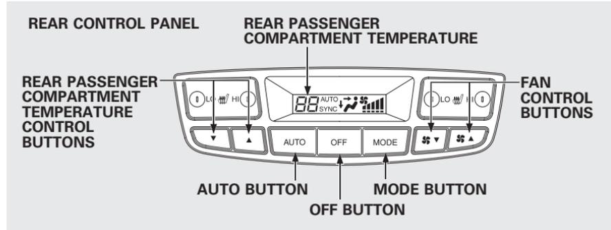
You can use the rear control panel when the indicator in the REAR button on the front control panel is on. Pressing any control button on the rear control panel turns on the rear button indicator on the front control panel.
