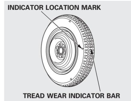
Replace the tire when you can see the tread wear indicator bars. The replacement should be the same size and design tire, mounted on the same wheel. The spare tire is not designed to be mounted on a regular wheel, and the spare wheel is not designed for mounting a regular tire.
