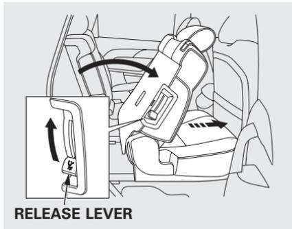
To get into the third row seats, pull up the lever on the side of the passenger's side second row seat-back. The seat-back will tilt forward, and then can be slid forward.
