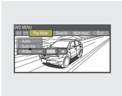
To change the view angle, highlight “Angle” from the play mode menu with the ▼ or ▲ button and press the ENT button. You can see the available angle options with the ► or ◀ button. Press the ENT button when your desired subtitle is highlighted.
