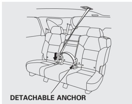
The lap/shoulder belts in the center seat of the second row and both of the third row seats are equipped with a detachable anchor that has two parts: a small latch plate and a buckle.
