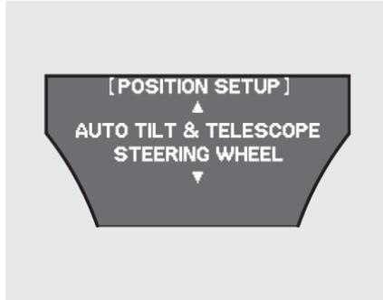
When “AUTO TILT & TELESCOPE STEERING WHEEL” is set to “ON,” the steering wheel automatically moves fully in and up when you turn the ignition switch to the LOCK (0) position and remove the key.
