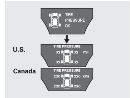
When the tire pressure monitor is shown on the multi-information display, press the SEL/RESET button. The display changes as shown.
