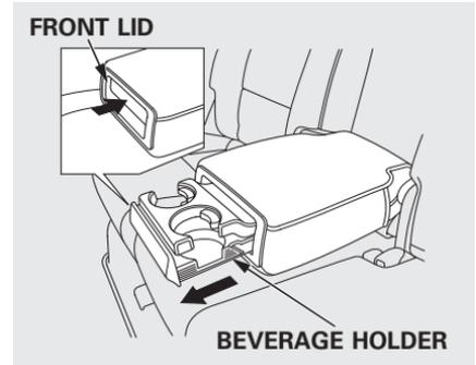
To open the beverage holder, press and release the front lid. To close, press the lid again until it latches. When you put back the armrest in the center seat-back, make sure the lid is closed properly.
