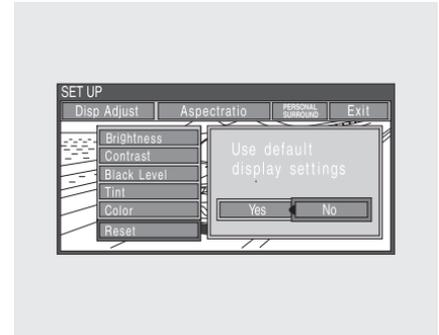
The display changes as shown above. Select “Yes,” and press the ENT button. You will see the message “Default display settings applied” on the display for 5 seconds.
