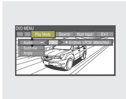
To change the Audio setting, highlight “Audio” from the play mode menu with the ▼ or ▲ button and press the ENT button. A submenu of the dubbed language appears. You can select another language by pressing the ► or ◀ button. The sound characteristics (Dolby Digital, LPCM, MPEG Audio, dts) recorded with the selected language is also displayed next to the language.
