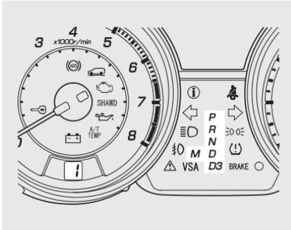
These indicators on the instrument panel show which position the shift lever is in. In the Sequential SportShift Mode, the “M” indicator next to the “D” indicator comes on, and the illuminated number under the charging system indicator shows you the gear you have selected.
