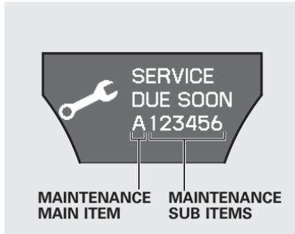
When the remaining engine oil life is 15 to 6 percent, the multi-information display shows a “SERVICE DUE SOON” message along with the maintenance schedule code indicating the main and sub items required at the time of the oil change. Refer to page 390 for a complete list of the maintenance main items and sub items.
