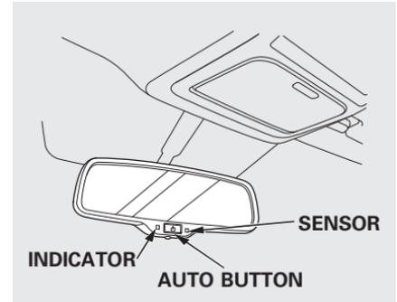
The inside mirror can automatically darken to reduce glare. To turn on this feature, press the button on the bottom of the mirror. The AUTO indicator comes on as a reminder. When it is on, the mirror darkens when it senses the headlights of a vehicle behind you, then returns to normal visibility when the lights are gone. Press the button again to turn off this feature.
