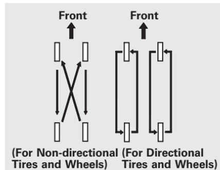
To help increase tire life and distribute wear more evenly, rotate the tires according to the maintenance messages displayed on the multi-information display. Move the tires to the positions shown in the illustration each time they are rotated. If you purchase directional tires, rotate only front-to-back.
