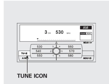
**TUNE** – Use the TUNE knob to tune the radio to a desired frequency. Turn the knob right to tune to a higher frequency, or left to tune to a lower frequency. To tune with the interface dial, push the selector down, and turn the knob to TUNE. Then press ENTER on the selector, and turn the knob to the desired frequency. To exit the TUNE mode, press ENTER on the selector.
