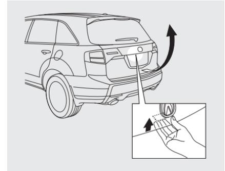
To open the tailgate, push up inside the handle, then lift up. To close the tailgate, use the inner handle to pull it down, then press down on the back edge.
