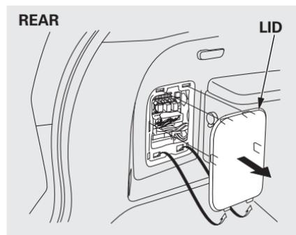
The rear fuse box is located at the left side of cargo area.
