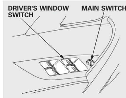
Turn the ignition switch to the ON (II) position to raise or lower any window. To open a window, push the switch down and hold it. Release the switch when you want the window to stop. Pull back on the switch and hold it to close the window.
