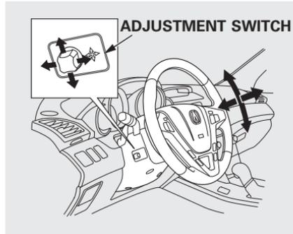
Move the steering wheel in, out, up, or down by pushing and holding the adjustment switch in that direction.
