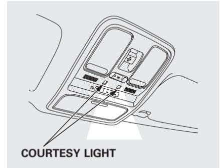
The courtesy light between the map lights comes on when you turn the parking lights on. To adjust its brightness, press either of the instrument panel brightness control buttons (+ or -).
