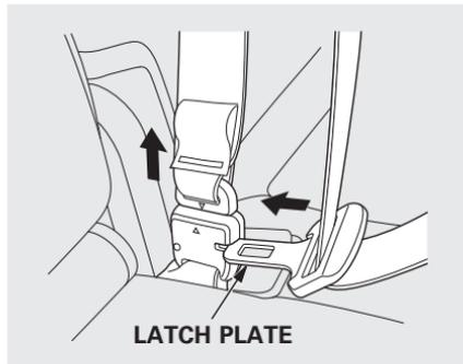
The seat belts in the second row center seat and the third row seats are equipped with detachable anchors.
