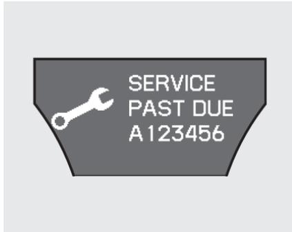
If the indicated maintenance service is not done and the remaining engine oil life reaches 0%, the multi-information display will show the message “SERVICE PAST DUE” and the maintenance item code(s). This message is displayed when the total mileage is less than 10 miles (for U.S. models) or 10 km (for Canadian models) after the engine oil life became 0%.
