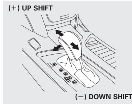
To enter the Sequential SportShift mode, move the shift lever further to the driver's side. To return to “D,” move the shift lever to the passenger's side.
