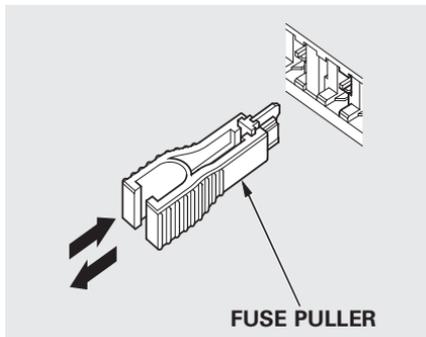
4. Check the smaller fuses in the under-hood fuse boxes and rear fuse box, and all the fuses in the interior and rear fuse boxes by pulling out each one with the fuse puller provided in the primary under-hood fuse box.
