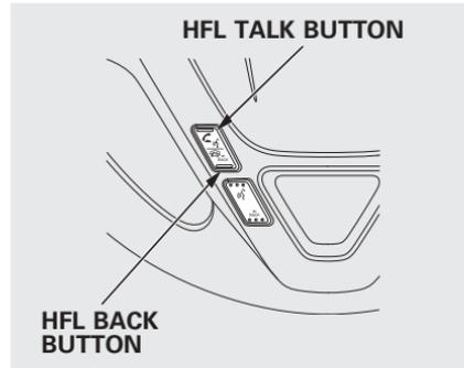
To operate the HFL, use the HFL Talk and Back buttons on the left side of the steering wheel.
