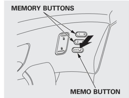
3. Press and release the MEMO button on the control panel. You will hear a beep. Immediately press and hold one of the memory buttons (1 or 2) until you hear two beeps. The indicator in the memory button will come on. The current positions of the driver's seat, steering wheel, and outside mirrors are now stored.
