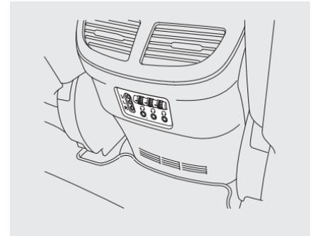
Auxiliary input jacks and headphone connectors for the rear entertainment system are on the back of the center console compartment.
