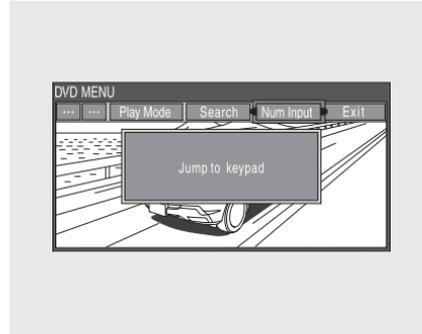
A numerical command can be issued to a DVD by inputting a two digit number, and a button number can be selected on the screen.
