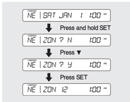
1. Press and hold the SET button for five seconds until the clock display changes to “ZON ? N.” (Clock adjustment mode will be started after the first two seconds.)
