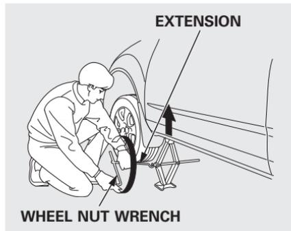
13. Use the extension and the wheel nut wrench as shown to raise the vehicle until the flat tire is off the ground.
