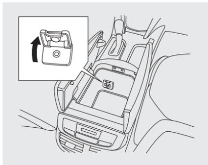
The auxiliary input jack is inside the front console compartment. The system will accept auxiliary input from standard audio accessories.
