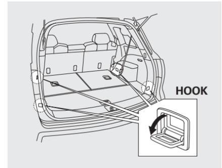
The hooks on the floor of the cargo area enable you to tie down items stored in the back. Make sure all stored items are secured before driving.
