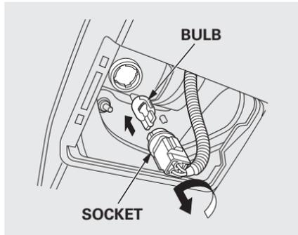
2. Remove the socket by turning it one-quarter turn counterclockwise.
