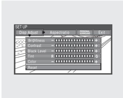
Select the quality you want to adjust by pressing the ▼ or ▲ button. Adjust the setting by pressing the ◀ or ▶ button. When you are finished with your adjustment, cursor back to the top of the setup menu, or press the RETURN button to exit.
