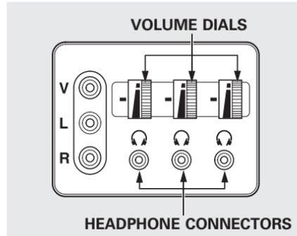
There are three headphone connectors for the third seat passengers. Each connector has its own volume control.
