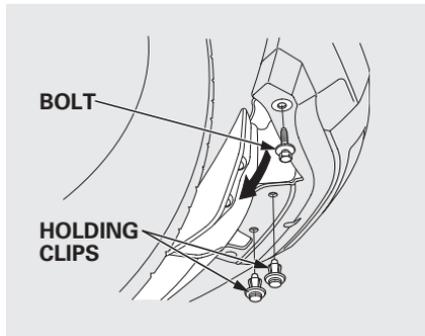
1. Remove the bolt and use the flat-tip screwdriver to remove the holding clips located under the front bumper.
