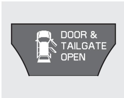
When both tailgate and one or more doors are not tightly closed, the “DOOR & TAILGATE OPEN” message will come on.
