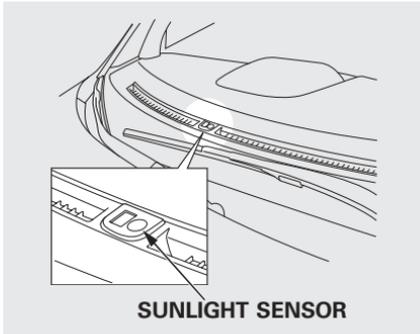
To regulate the interior temperature and humidity, the climate control system has two sensors. A sunlight sensor is located in the top of the dashboard and a temperature/humidity sensor is next to the steering column. Do not cover the sensors or spill any liquid on them.
