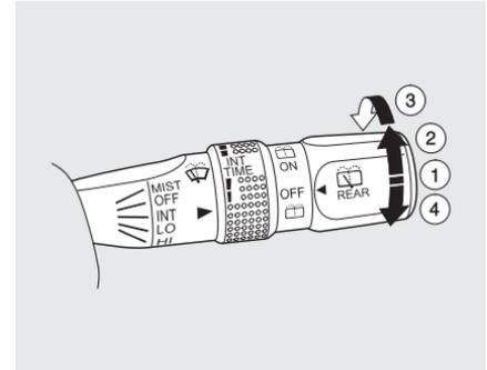
1. Rotate the switch clockwise to turn the rear window wiper ON.
