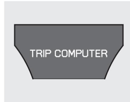
When the main menu displays "TRIP COMPUTER", pressing the SEL/RESET button changes the display to "AVERAGE FUEL A/RANGE" to "AVERAGE FUEL B/RANGE" and to "AVERAGE SPEED/ELAPSED TIME".
