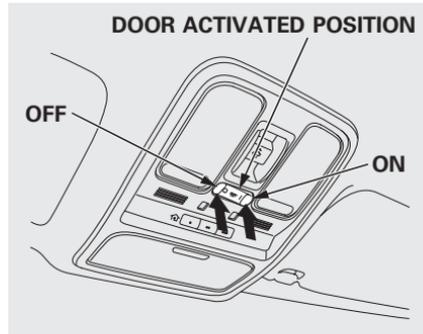
The light control switch has three positions: OFF, Door Activated, and ON.
