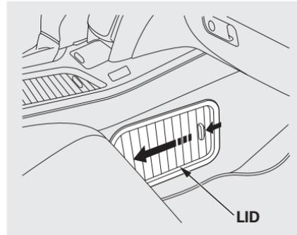
The storage compartment with a sliding lid is at the left-side foot of the front passenger seat.
