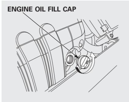
Unscrew and remove the engine oil fill cap on top of the valve cover. Pour in the oil slowly and carefully so you do not spill. Clean up any spills immediately. Spilled oil could damage components in the engine compartment.
