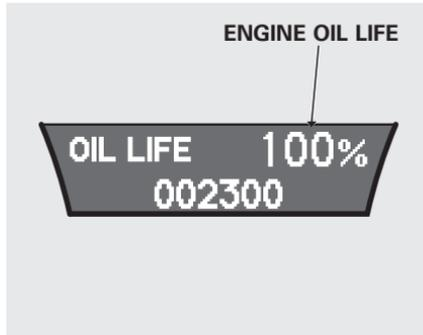
This shows the remaining life of the engine oil. It shows 100% after the engine oil is replaced and the display is reset. The engine oil life is calculated based on engine operating conditions and accumulated engine revolutions. For more information, see page [383](#).
