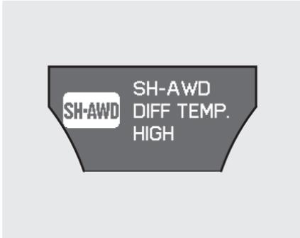
If the SH-AWD indicator blinks while driving, it indicates the differential temperature is too high. You will also see an “SH-AWD DIFF TEMP. HIGH” message on the multi-information display. If this happens, pull to the side of the road when it is safe, shift to Park, and let the engine idle until the indicator goes out. If the indicator does not go out, take your vehicle to a dealer to have it checked.
