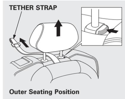
1. After properly securing the child seat (see page 50), lift the head restraint, then route the tether strap over the seat-back and through the head restraint legs.
