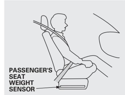
The passenger's advanced front airbag system has weight sensors under the seat. Although Acura does not encourage carrying an infant or small child in front, if the sensors detect the weight of an infant or small child (up to about 65 lbs or 29 kg), the system will automatically turn the passenger's front airbag off.
