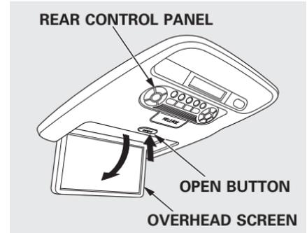
Open the overhead screen by pushing the OPEN button. The screen will swing down part-way. Pivot the screen the rest of the way. If you pivot the screen too far forward, past the second detent, the display will turn off. Pivot the screen back to the second or first detent to turn the display back on. To close the screen, pivot it up until it latches.
