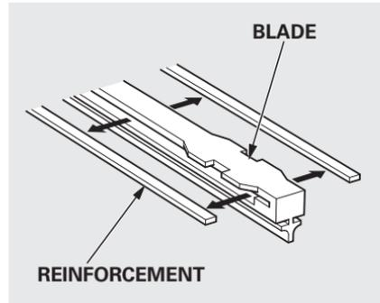
4. Examine the new wiper blades. If they have no plastic or metal reinforcement along the back edge, remove the metal reinforcement strips from the old wiper blade, and install them in the slots along the edge of the new blade.
