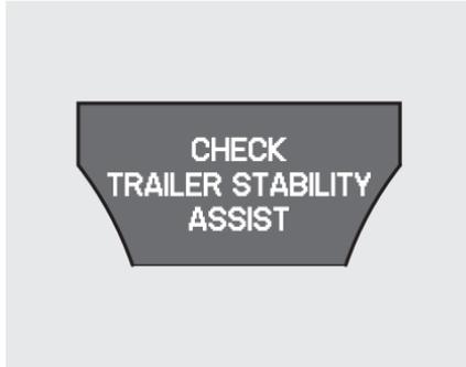
The control unit monitors the VSA circuitry and the braking system. If there is a problem with the brake lighting system, the trailer stability assist function shuts down and the “CHECK TRAILER STABILITY ASSIST” message appears on the multi-information display.
