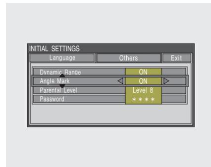
Select “Angle Mark” by pressing the ▼ or ▲ button. The above submenu appears. If you want the angle mark to be displayed, select “ON” with the ► or ◀ button.
