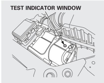
Check the condition of the battery monthly by looking at the test indicator window:
