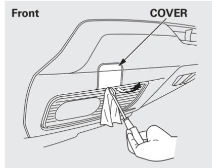
1. Remove the cover, put cloth on the edge of the cover and carefully pry with a small flat-tip screwdriver or a metal fingernail file.
