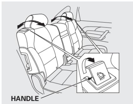
To change the seat-back angle of the seats in the second row, pull up on the handle on the outside of the seat-back, and push the seat-back.
