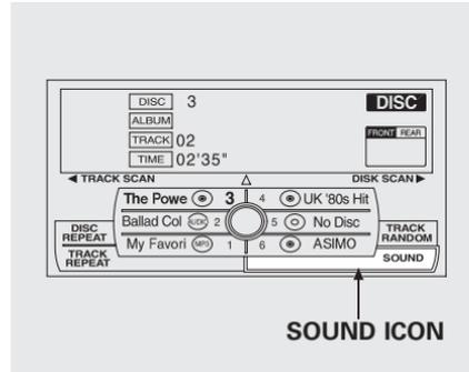
To adjust them, press the AUDIO button, push the interface selector down, and turn the interface knob to SOUND. Then press ENTER on the selector.
