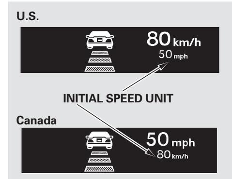
If you change the speed unit measurement from the factory default setting, the initial speed unit measurement is shown under the current unit.
