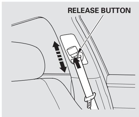
The front seats have adjustable seat belt anchors. To adjust the height of an anchor, press and hold the release button and slide the anchor up or down as needed (it has four positions).
