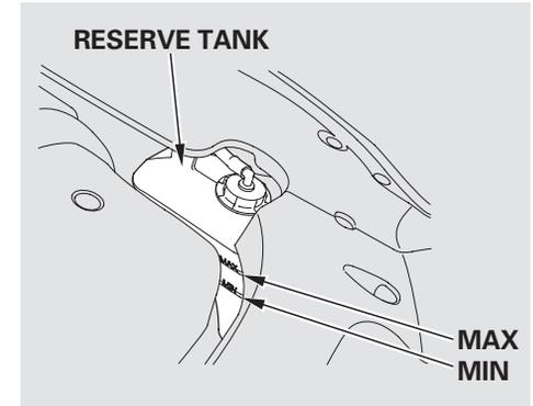
Look at the coolant level in the radiator reserve tank. Make sure it is between the MAX and MIN lines. If it is below the MIN line, see **Adding Engine Coolant** on page 461 for information on adding the proper coolant.
