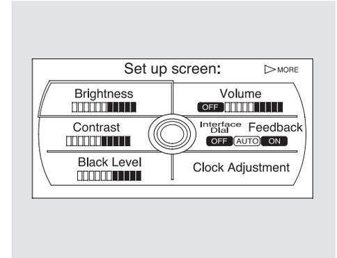
The first setup screen allows you to change the system’s brightness, contrast, black level, volume, interface dial feedback, and clock adjustment. To select a setup item, turn the interface knob until it is highlighted, then press ENTER to select it.
