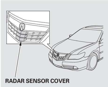
The radar sensor is located under the Acura emblem in the front grille. If the radar sensor cover is covered with mud, dirt, dead leaves, wet snow, etc., or if you put a sticker on it, the CMBS will automatically shut off, and the CMBS indicator on the instrument panel will come on. You will also see a "CHECK CMBS RADAR SENSOR" message on the multi-information display for about 5 seconds.
