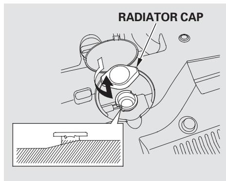
2. When the radiator and engine are cool, relieve any pressure in the cooling system by turning the radiator cap counterclockwise, without pressing down.
