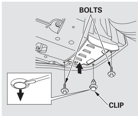
1. Use a Phillips-head screwdriver to remove the two undercover bolts, and remove the holding clip with a flat-tip screwdriver.
