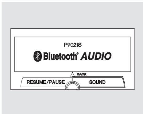
Press the AUDIO button, then push down the selector to display the audio menu. Turn the knob to switch the setting between the resume/pause mode and the sound mode. Select SOUND, then press ENTER to set your selection.
