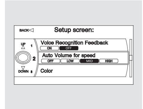
The second setup screen allows you to change the system's voice recognition feedback, auto volume for speed, and clock settings. To select a setup item, turn the interface knob until it is highlighted, then press ENTER to select it.
