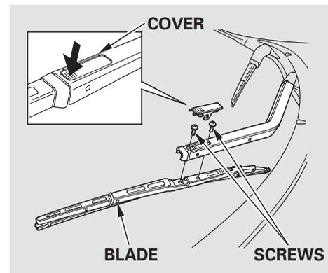
2. Push the end of the cover on the blade assembly until the other end is pivoted out, and remove the cover.
