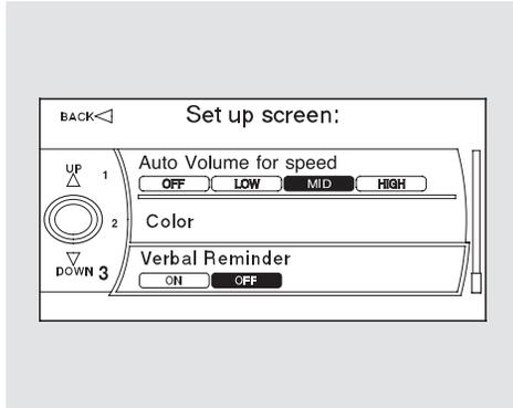
The third setup screen allows you to change the verbal reminder. To select a setup item, turn the interface knob until it is highlighted, then press ENTER to select it.
