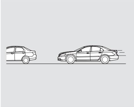
If the system senses a likely collision with a vehicle or object ahead of you, it alerts you with a visual alert or a combination of a visual alert and an audible alert.
