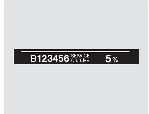
Press the SEL/RESET button on the steering wheel repeatedly to select the engine oil life. The message “SERVICE OIL LIFE”, along with “5%”, and the maintenance item code(s) are displayed on the lower part of the multi-information display when the calculated engine oil life is 1 to 5 percent (see page 445).
