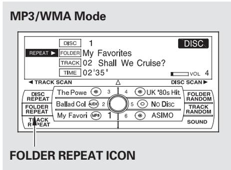
This feature, when activated, replays all files in the selected folder. To activate folder repeat mode, select FOLDER REPEAT by using the interface knob, and press ENTER on the interface selector. You will see REPEAT next to FOLDER on the screen. To turn this feature off, highlight FOLDER REPEAT (if not already highlighted), and press ENTER on the interface selector again.
