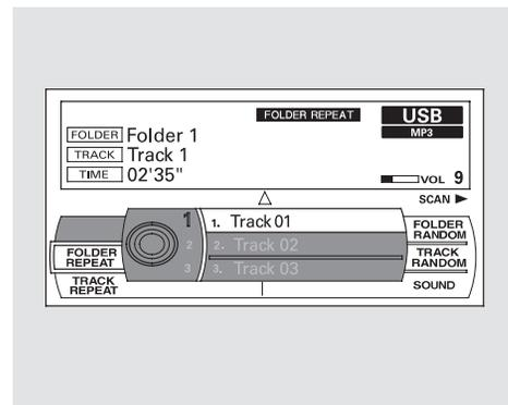
You can also select a folder or file from the list by using the interface dial. Press the AUDIO button to show the audio control display.
