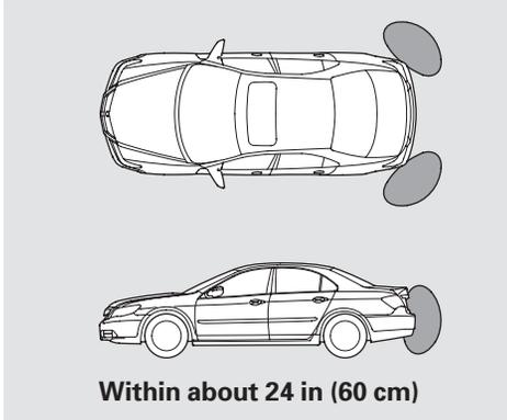
The range of the corner sensors and the rear center sensors are limited. Each corner sensor is capable of sensing an obstacle within about 24 in (60 cm).
