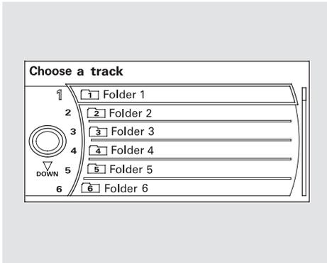
Push up the selector on the interface dial to switch the display to the folder list, then turn the knob on the interface dial to select a folder.
