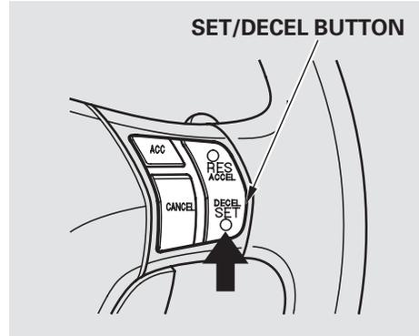
3. Press and release the SET/DECEL button on the steering wheel, then release the accelerator pedal.
