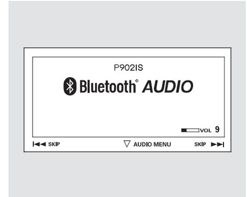
You can also operate the skip function with the interface dial on the audio control display. Push the AUDIO button. Each time you push the selector to the right, the system skips forward to the beginning of the next file. Push it to the left to skip backward to the beginning to the current file. Push the selector to the left again to skip to the previous file.
