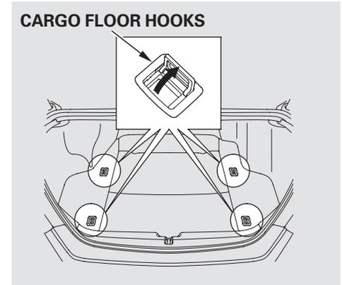
The cargo floor hooks can also be used to tie down and secure items on the floor.
