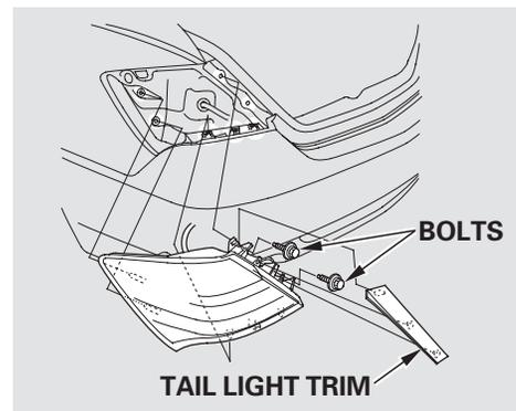
3. Carefully pry in the top or bottom edge of the trim with a small flat-tip screwdriver, and pull the trim straight back.
