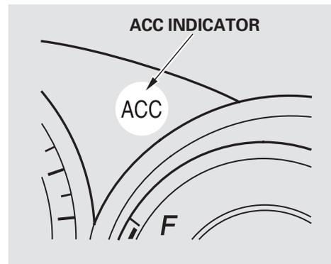
This indicator normally comes on for a few seconds when you turn the ignition switch to the ON (II) position. If it comes on at any other time, there is a problem in the ACC system. If this happens, take the vehicle to your dealer to have it checked.
