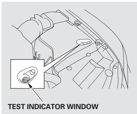
Check the condition of the battery monthly by looking at the test indicator window. The label on the battery explains the test indicator's colors. To see the label, remove the battery cover (see page 492).
