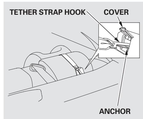
7. Route the tether strap over the head restraint, then attach the tether strap hook to the anchor, making sure the strap is not twisted.
