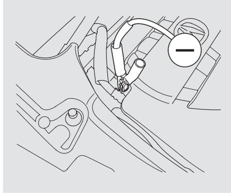
5. Connect the second jumper cable to the negative (–) terminal on the booster battery. Connect the other end to the engine hanger as shown. Do not connect this jumper cable to any other part of the engine.
