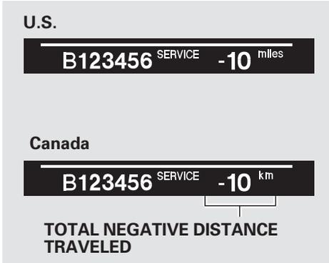
When you press the SEL/RESET button to select the engine oil life minder, the message “SERVICE”, along with the maintenance item code and the total negative distance traveled after the oil life became 0 percent, will be displayed on the lower part of the multi-information display.
