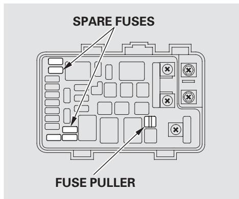
If you cannot drive the vehicle without fixing the problem, and you do not have a spare fuse, take a fuse of the same rating or a lower rating from one of the other circuits. Make sure you can do without that circuit temporarily (such as the accessory power socket).
