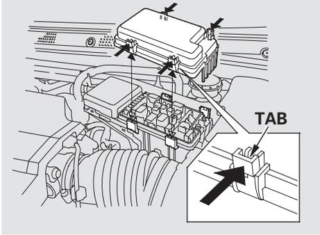
The primary under-hood fuse box is in the engine compartment on the driver's side. To open it, push the tabs as shown.
