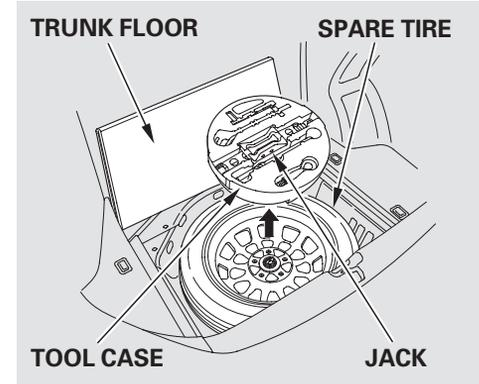
3. Open the trunk, and fold the trunk floor forward.
