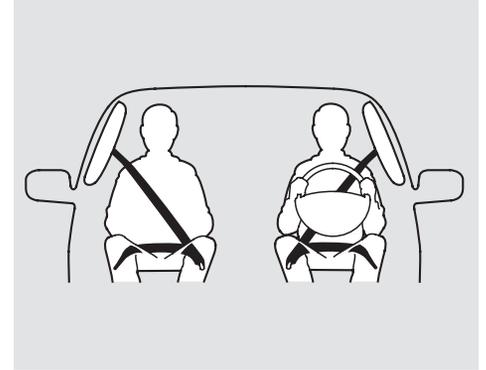
In addition, your vehicle has side curtain airbags to help protect the heads of the driver, front passenger, and passengers in the outer rear seating positions during a moderate to severe side impact (see page 33 for more information on how your side curtain airbags work).
