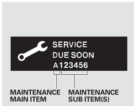
When the remaining engine oil life is 15 to 6 percent, the multi-information display shows a “SERVICE DUE SOON” message along with the maintenance schedule code(s) indicating the main and sub items required at the time of the oil change. Refer to pages 453 and 454 for a complete list of the maintenance main items and sub items.
