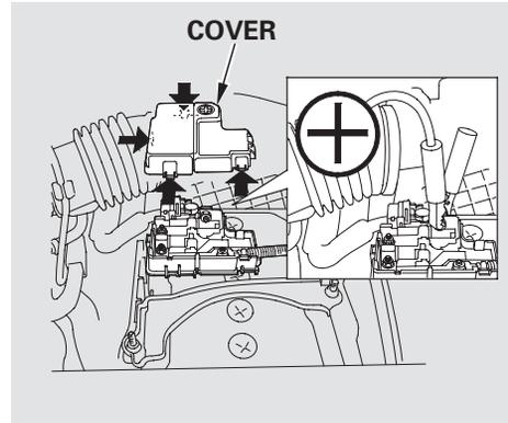
3. Remove the battery cover (see page 492), then remove the secondary under-hood fuse box cover from the positive (+) terminal on the battery.
