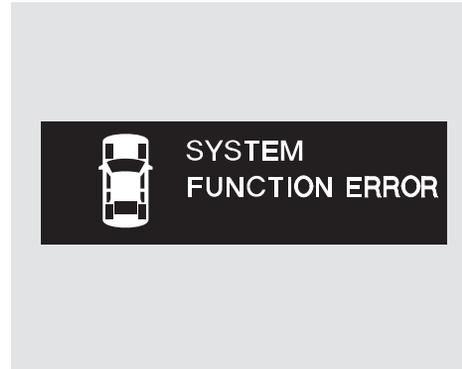
If there is a system error with the TPMS, the multi-information display shows a “SYSTEM FUNCTION ERROR” message (see page 433 ), and the tire pressure readings will not be displayed. You will also see a “CHECK TPMS SYSTEM” message on the multi-information display (see page 433 ).
