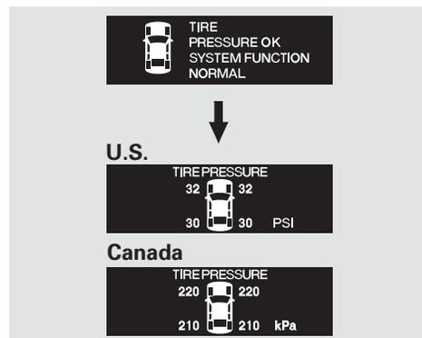
When the tire pressure monitor is shown on the multi-information display, press the SEL/RESET button. The display changes as shown.
