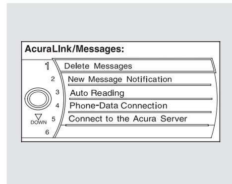
To access the following functions, press the SETUP button, push the interface selector to the right to select Other, then rotate the interface knob to select AcuraLink/ Messages.
