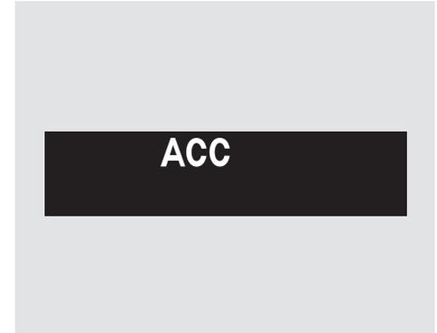
When your speed reaches 25 mph (40 km/h), ACC goes into wait mode, and "ACC" is shown on the multi-information display.
