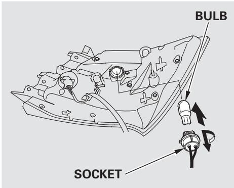
6. Remove the socket by turning it one-quarter turn counterclockwise.
