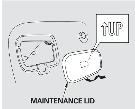
If the fuel fill door release button does not work, use the release lever inside the left maintenance lid in the trunk.
