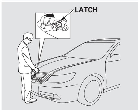
2. Reach between the hood and the front bumper with your finger. Slide the latch handle up.
