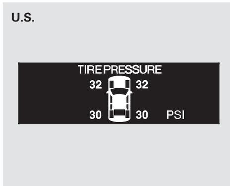
When the TPMS is functioning normally, you can see the tire pressure readings of each tire in psi (U.S. models) or kPa (Canadian models) by pressing the SEL/RESET button while the multi-information display shows the tire pressure monitor.
