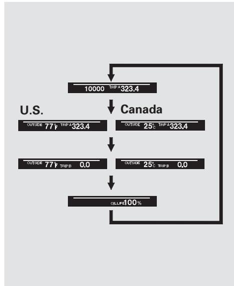
With the ignition switch in the ON (II) position, the lower part of the multi-information display changes as shown in the illustration, each time you press the SEL/RESET button.
