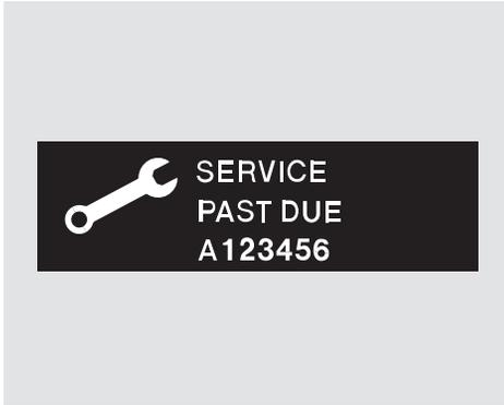
If the indicated maintenance service is not done and the remaining engine oil life reaches 0%, the multi-information display will show the message “SERVICE PAST DUE” and the maintenance item code(s). This message is displayed when the total distance traveled is less than 10 miles (for U.S. models) or 10 km (for Canadian models) after the engine oil life became 0%.
