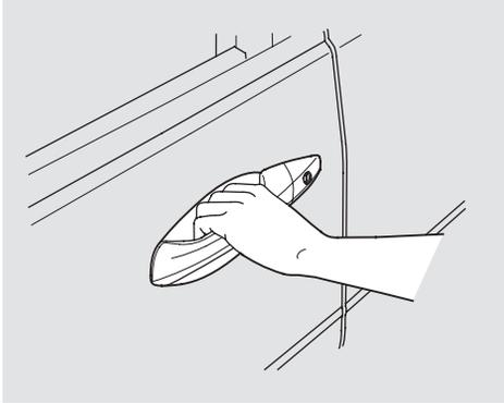
The handle of each front door has a sensor. That sensor works with the remote so you can automatically unlock/lock the door(s).
