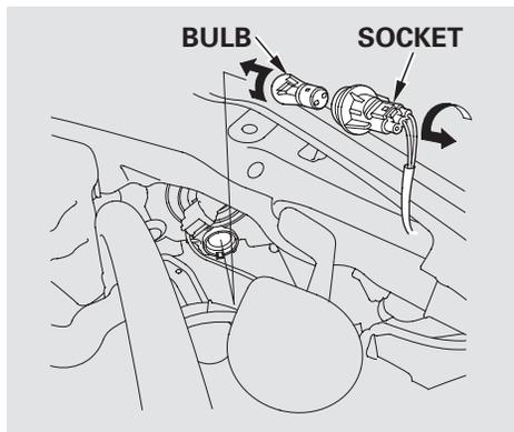
3. Remove the socket from the headlight assembly by turning it one-quarter turn counterclockwise.
