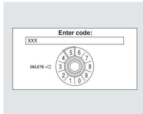
If the battery goes dead or is disconnected for any reason, you will have to enter a security code into both the audio system and the compass system before you can use it again.
