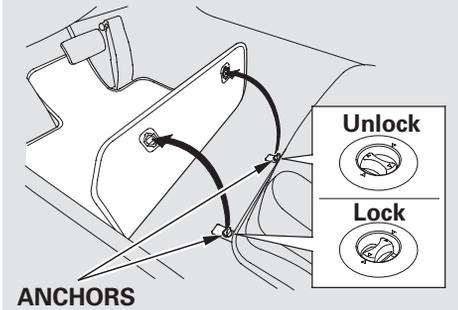
The floor mats that came with your vehicle hook over the floor mat anchors. This keeps the floor mats from sliding forward (possibly interfering with the pedals), or backwards (making the front passenger's weight sensors ineffective).
