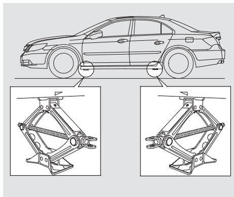
7. Place the jack under the jacking point nearest the tire you need to change. It is pointed to by a  $\triangle$  mark molded into the underside of the body. Turn the end bracket clockwise until the top of the jack contacts the jacking point. Make sure the jacking point tab is resting in the jack notch.
