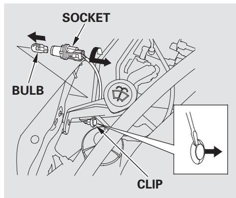
4. Remove the socket from the headlight assembly by turning it one-quarter turn counterclockwise.
