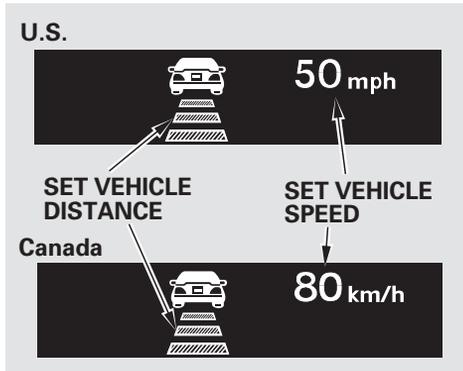
When the speed is set, it is shown along with a vehicle icon and distance bars on the multi-information display. Refer to page 328 for how to set and change the set distance between your vehicle and the vehicle ahead of you.
