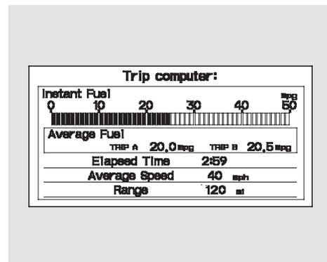
The **Trip computer** screens display the trip information from the multi-information display in the gauge assembly.
