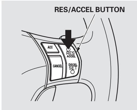
The set speed can be increased by using the RES/ACCEL button or the accelerator pedal.
