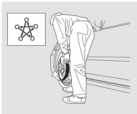
13. Tighten the wheel nuts securely in the same crisscross pattern. Have the wheel nut torque checked at the nearest automotive service facility. Tighten the wheel nuts to: 94 lbf·ft (127 N·m , 13 kgf·m)
