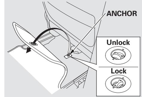
Make sure the rear floor mats are properly hooked to the floor mat anchors. Your vehicle is equipped with front passenger's seat weight sensors. If the rear passenger's floor mat is on the seat rail of the front passenger's seat, the sensors will detect the decreased weight on the seat, and they may not work properly.
