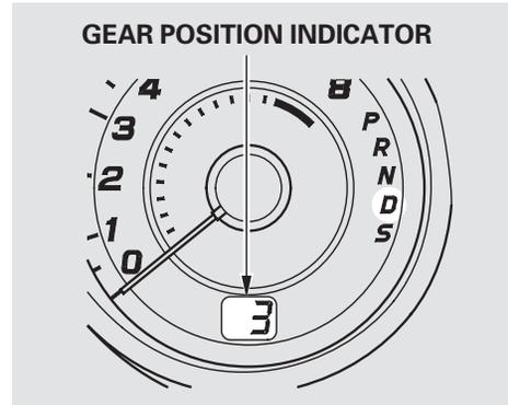
When you pull either paddle shifter, the gear position indicator shows you the selected gear number.
