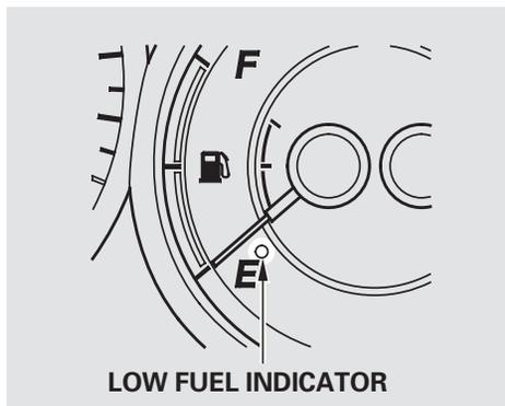
This indicator is in the fuel gauge. It comes on as a reminder that you must refuel soon. You will also see a “FUEL LOW” message on the multi-information display. When the indicator comes on, there are about 2.69 U.S. gal (10.2 ℓ) of fuel remaining in the tank. When the needle reaches E, there is a very small amount of fuel in the tank.
