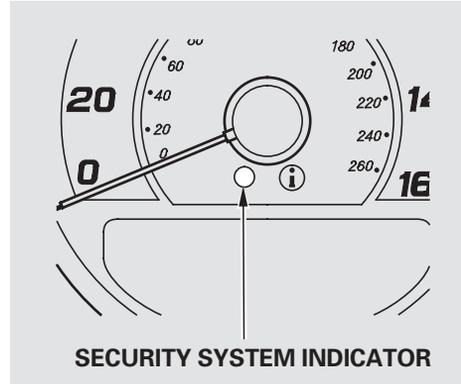
Once the security system sets, opening any door, the trunk, or hood without using the built-in key or the keyless access remote, will cause the alarm to activate. It also activates if the ignition switch is turned to the ON (II) position, the audio unit is removed from the dashboard, or the wiring is cut.
