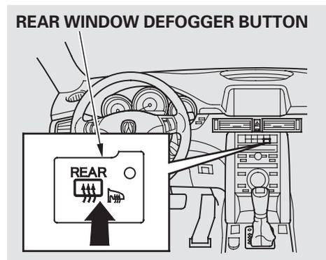
The rear window defogger clears fog, frost, and thin ice from the window. Push the defogger button to turn it on and off. Pushing this button also turns the mirror heaters on and off. The indicator in the button comes on to show the defogger is on. If you do not turn it off, the defogger will shut itself off after 5 to 40 minutes (depending on the ambient temperature). It also shuts off when you turn off the ignition switch. You
