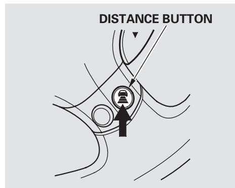
With ACC on, the distance between your vehicle and the vehicle ahead of you is controlled and maintained. You can change this distance to one of three ranges: long, middle, or short.
