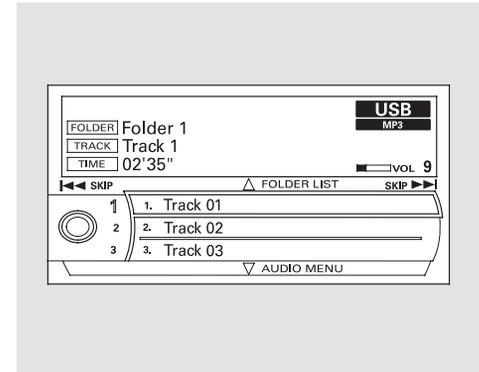
You can select any type of repeat, random and scan modes on the audio menu screen. Press the AUDIO button to show the audio control display. Push down the selector to display the audio menu items.
