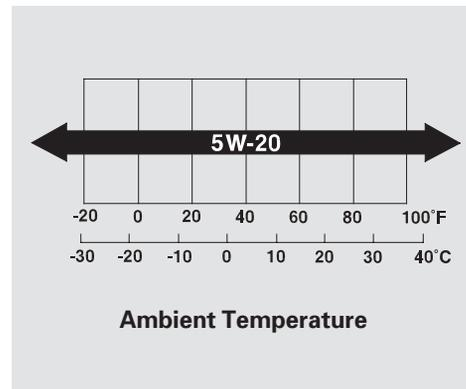
Acura Motor Oil is the preferred 5W-20 lubricant for your vehicle. It is highly recommended that you use Acura Motor Oil in your vehicle for optimum engine protection. Make sure the API Certification Seal says "For Gasoline Engines."
