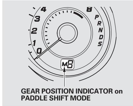
Using a paddle shift mode, the gear position indicator shows you the selected gear number (see page 407).
