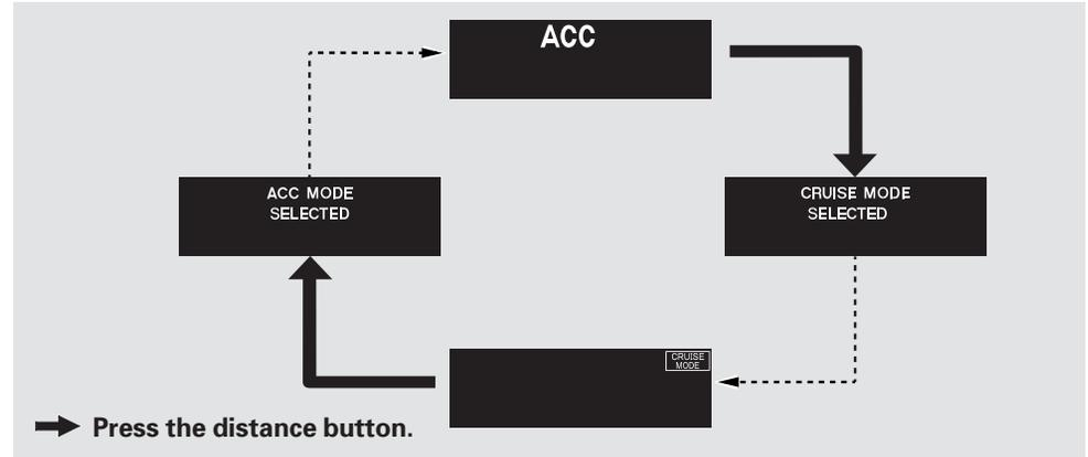
When you press the button, you will see CRUISE MODE SELECTED on the multi-information display for 2 seconds. To switch back to ACC, press and hold the distance button again for 1 second.
