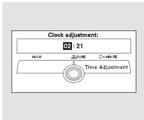
To adjust the hour, turn the interface knob, then press ENTER.
