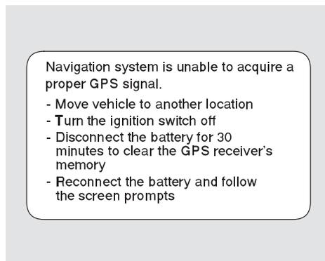
If within ten minutes the system fails to locate a sufficient number of satellites to locate your position, the screen above appears. Follow the instructions on the screen.
