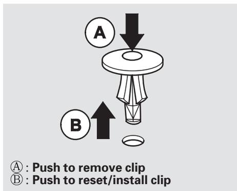
2. Remove the holding clips by pushing on the center of each fastener head.
