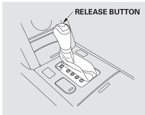
To shift from Park to any position, press firmly on the brake pedal, and press the release button on the top of the shift lever, then move the lever. You cannot shift out of Park when the ignition switch is in the LOCK (0) or ACCESSORY (I) position.
