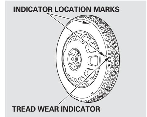
Replace the tire when you can see the tread wear indicator bars. The replacement tire should be the same size and design, mounted on the same wheel. The spare tire is not designed to be mounted on a regular wheel, and the spare wheel is not designed for mounting a regular tire.
