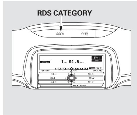
You can also select an RDS category with the TUNE bar. Press either side ( <<< or >>> ) of the TUNE bar to display an RDS category in the display. Select a category by pressing either side of the bar.
