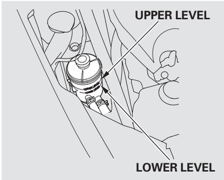
After removing the right engine compartment cover (see page 457), check the level on the side of the reservoir when the engine is cold. The fluid should be between the UPPER LEVEL and LOWER LEVEL. If not, add power steering fluid to the UPPER LEVEL mark.
