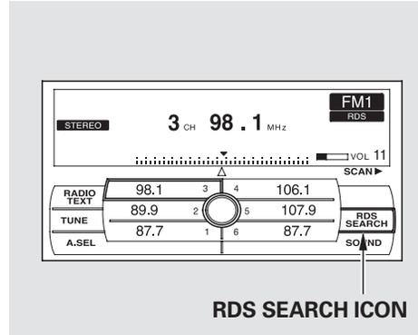
With the FM band selected, you can select the program type provided by the RDS. Press the AUDIO button to display the radio information on the screen. Push down the selector on the interface dial, then turn the knob to select RDS SEARCH icon. Press ENTER to set your selection. The principal RDS categories are shown as follows:
