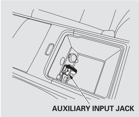
The auxiliary input jack is inside the console compartment. The system will accept auxiliary input from standard audio accessories using a 1/8 inch (3.5 mm) stereo miniplug.
