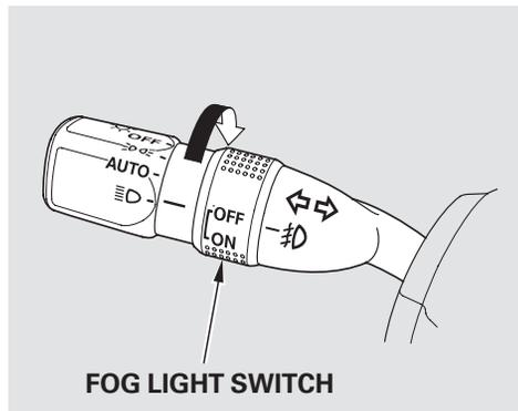
Turn the fog lights on and off by turning the switch next to the headlight switch.
