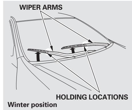
Adjust the wiper arms to the winter position by holding both arms as shown in the illustration at the same time. Pull on the arm, parallel to the windshield, until it locks in the higher position.
