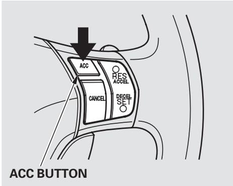
1. Push the ACC button on the steering wheel. The ACC indicator on the instrument panel comes on, and "ACC" is shown on the multi-information display.
