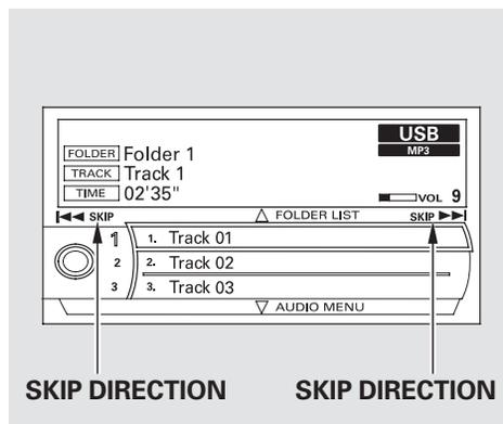
You can also change files with the interface dial. Press the AUDIO button to show the audio control display. Push the selector to the right side to skip to the beginning of the next file, and to the left side to skip to the beginning of the current file. Pushing it to the left again skips to the beginning of the previous file.
