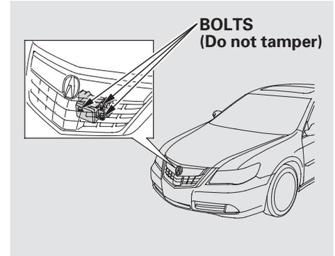
There are three bolts on the sides of the radar sensor. Do not tamper with these bolts, or you may cause the system to malfunction.
