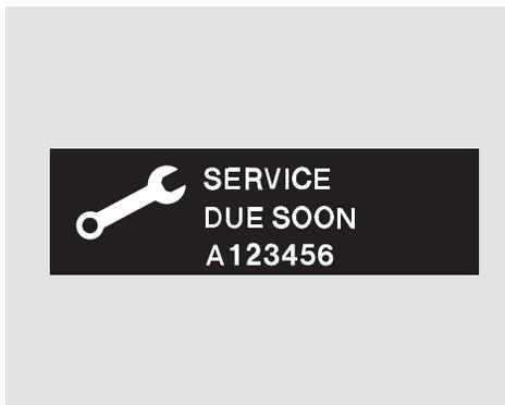
When the engine oil life reaches 15%, the display shows “SERVICE DUE SOON” and the code for the maintenance items to be performed.
