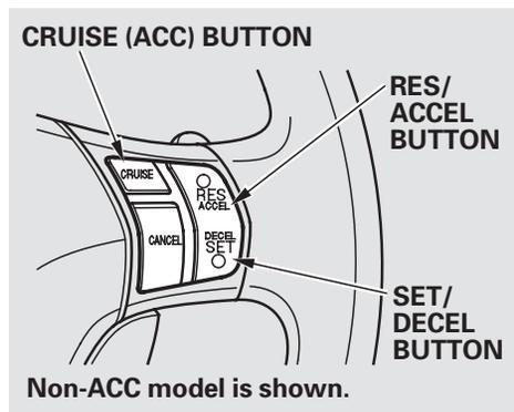
1. Push in the CRUISE button or the ACC button (models with adaptive cruise control) on the steering wheel. The CRUISE MAIN or green ACC indicator (models with ACC) indicator on the instrument panel comes on.
