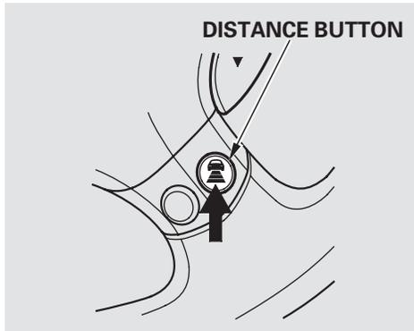
To switch from ACC to cruise control, press the distance button on the steering wheel, and hold it for 1 second.
