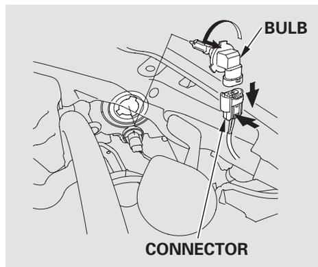
3. Remove the electrical connector from the bulb by pushing on the tab and pulling the connector down.
