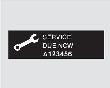
When the remaining engine oil life is 1 to 5 percent, the multi-information display shows a “SERVICE DUE NOW” message with the maintenance items. When you see this message have the indicated maintenance performed as soon as possible.
