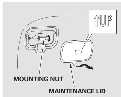
1. Open the trunk lid, and remove the left or right maintenance lid.
