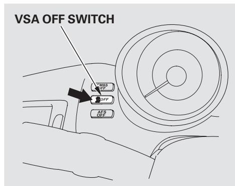
This switch is at the right side of the left vent. To turn the VSA system on and off, press and hold it until you hear a beep.
