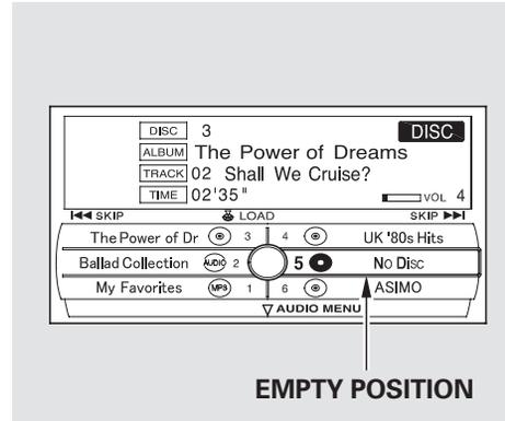
You can load a disc into an empty position while a disc is playing. Press the AUDIO button to view the audio control display. Select the empty position (“No Disc” is shown on the audio control display) by rotating the interface dial. Then press ENTER on the selector to enter your selection. The current disc stops playing and starts the loading sequence. The disc just loaded will play.
