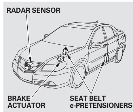
The CMBS consists of a radar sensor in the front grille, a brake actuator in the engine compartment, an indicator on the instrument panel, seat belt e-pretensioners on the front seats, and an on/off button on the dashboard.
