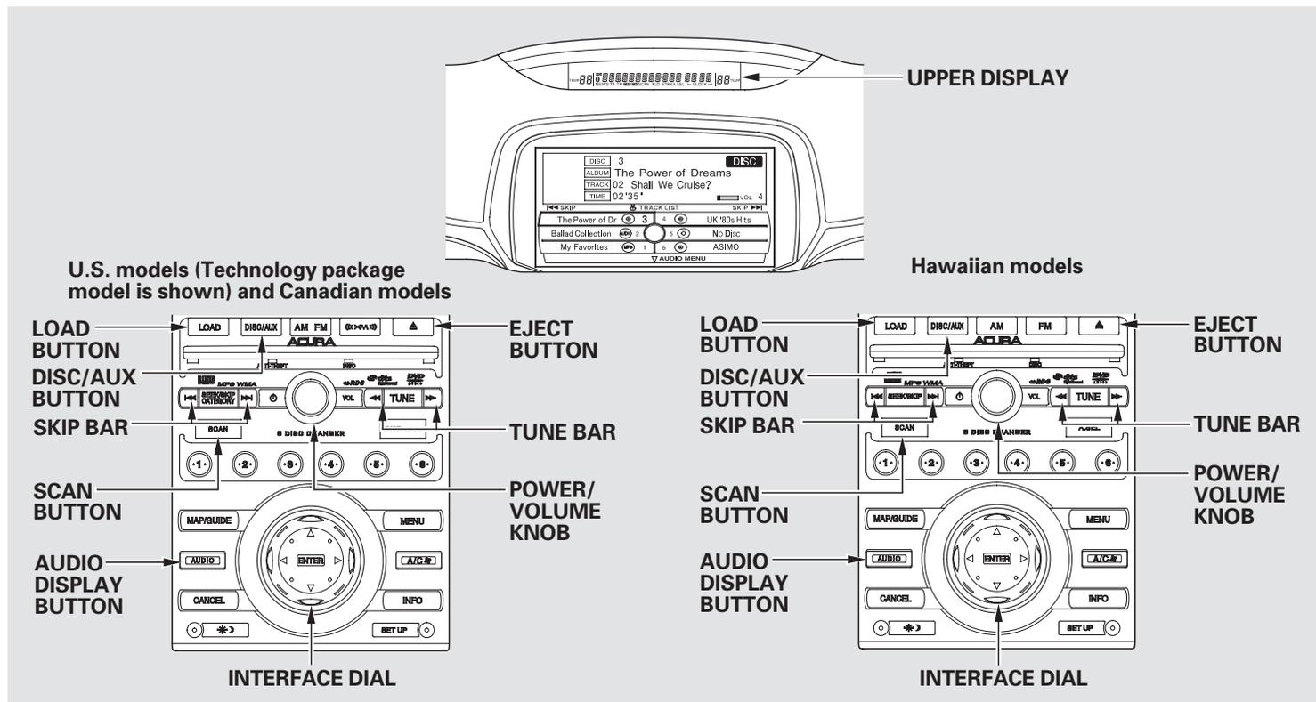
Your vehicle's audio system has an in-dash disc changer with the same controls used for the radio. To operate the disc changer, the ignition switch must be in the ACCESSORY (I) or the ON (II) position.
