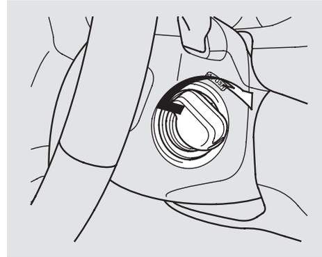
When you push the ignition switch, the remote and the vehicle recognize each other. After the recognition, the remote indicator flashes, and a beeper sounds once. After the beep, turn the ignition switch.
