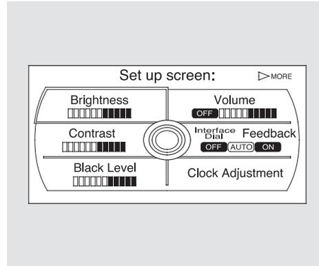
Select the **Clock Adjustment** by turning the interface knob, then press ENTER.
