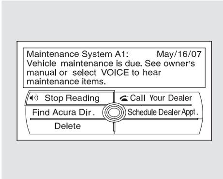
These messages provide detailed information about the service needed for your vehicle. When a maintenance message appears on the multi-information display, a list of needed maintenance items is provided through an AcuraLink message. These messages tell you the exact maintenance needed, helping you to avoid unnecessary maintenance costs.
