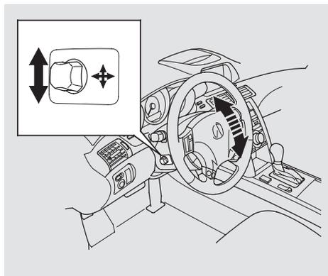
Move the steering wheel in, out, up, or down by pushing and holding the adjustment switch in that direction.
