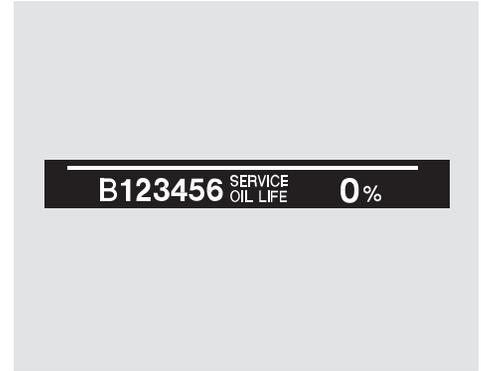
Press the SEL/RESET button on the steering wheel repeatedly to select the engine oil life minder. The message “SERVICE OIL LIFE”, along with “0%”, and the maintenance item code are displayed on the lower part of the multi-information display when the calculated engine oil life is 0 percent.
