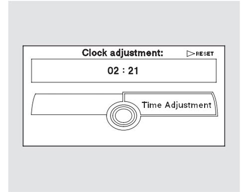
Select the **Time Adjustment**, then press ENTER. The display changes to the **Time Adjustment** screen for HOUR.
