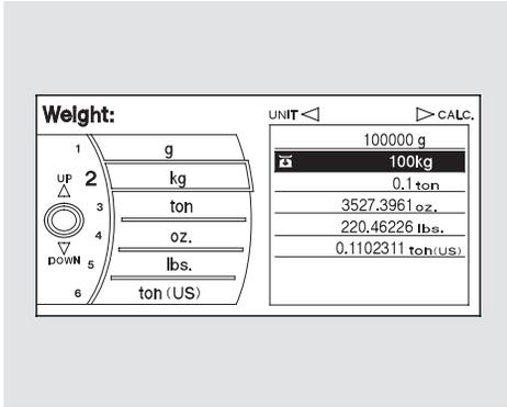
4. Turn the interface knob until the unit you want to convert from is highlighted (kilogram, for example), then press ENTER to select it as it the example above.
