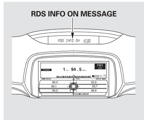
To switch the function between on and off, press and hold the DISP button. With the system on, you will see the “RDS INFO ON” message on the upper display. If the station you are listening to is an RDS station, the displayed frequency switches to the station name.
