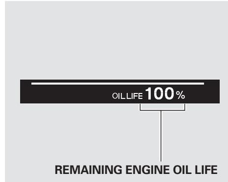
To see the remaining engine oil life displayed on the lower right corner on the multi-information display as a percentage, turn the ignition switch to the ON (II) position, and press the SEL/RESET button on the steering wheel repeatedly until the engine oil life appears (see page 73 ).
