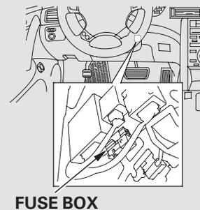
To open the secondary fuse box lid, push the tab in the direction as shown in the illustration.
