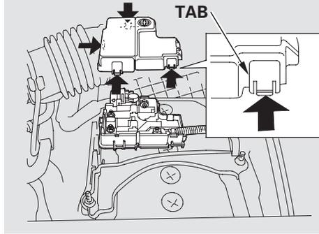
The secondary under-hood fuse box is on the battery. To open it, push the tabs as shown.
