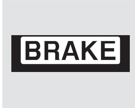
The visual alert is an amber colored BRAKE message that flashes on the multi-information display, the audible alert is a constant beeping sound. If one or more of the alerts come on, take the appropriate means to prevent a collision (apply the brakes, change lanes, etc.).
