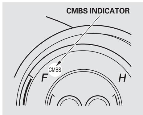
This indicator comes on for several seconds when you turn the ignition switch to the ON (II) position. It also comes on and stays on when you turn the CMBS off by pressing the CMBS OFF button.
