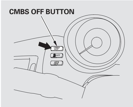
To switch the CMBS off, press the CMBS OFF button on the dashboard for about 1 second. When you do this, a beeper sounds, a CMBS indicator on the instrument panel comes on, and a CMBS OFF message appears on the multi-information display. To switch the system back on, press the button again for about 1 second.
