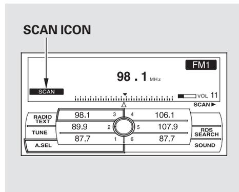
**SCAN** – The scan function samples all stations with strong signals on the selected band. To activate it, press
