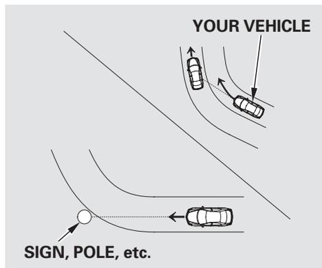
Because of the road condition (curved, winding, etc.) or the state of your vehicle (turning angle, lane position, etc.), CMBS can sometimes mistake a stationary object (light pole, traffic sign, guard rail, etc.) as a vehicle ahead of you and temporarily operate. This is normal.
