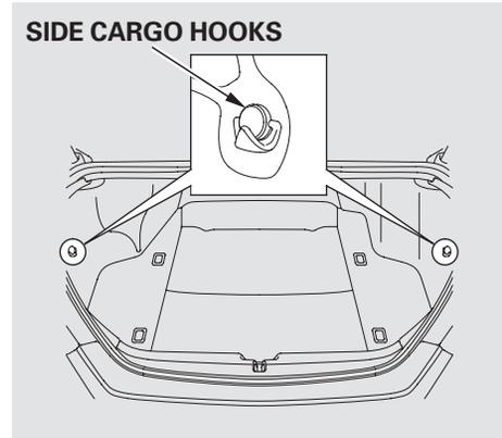
There are hooks on the floor and both sides of the trunk. They can be used to install the cargo net for securing items. The side cargo hooks are designed to hold light items (maximum load: 6 lbs or 3 kgs for each hook). Heavy objects may damage the side hooks.
