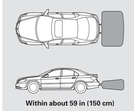
The rear center sensors sense an obstacle within about 59 in (150 cm).
