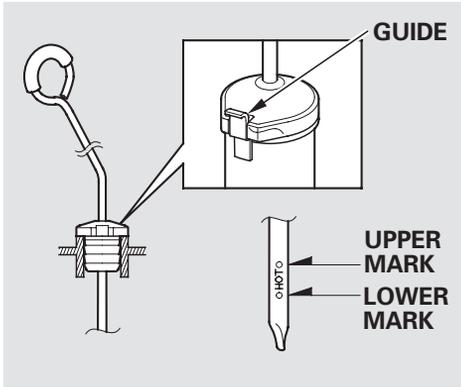
3. Insert the dipstick all the way into the transmission as shown.
