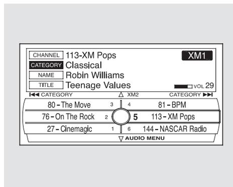
To listen to XM Radio, turn the ignition switch to the ACCESSORY (I) or ON (II) position, and press the « XM » button. The last channel you listened to will show in the display. Adjust the volume by turning the power/volume knob.
