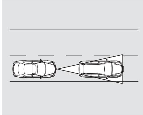
*When a vehicle ahead is within ACC range and going at a steady speed*
