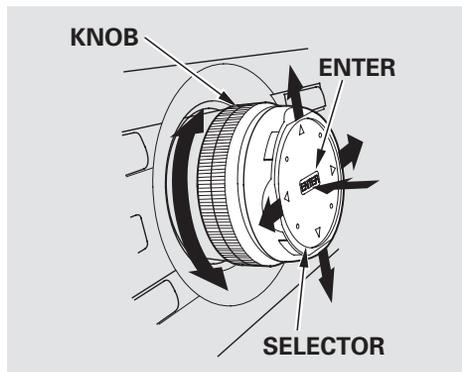
Most functions of the compass system can be accessed with the interface dial. The interface dial has two parts: a knob and a selector.
