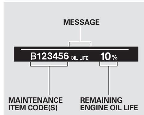
Press the SEL/RESET button on the steering wheel repeatedly to select the engine oil life. The message “OIL LIFE” along with the percentage of oil life remaining and the maintenance item code(s), appear on the lower part of the multi-information display.
