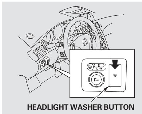
The headlight washers can be operated at any time by pressing the headlight washer button located next to the steering wheel column. The headlights must be turned on to use this button. In addition, the headlight washer operates without pressing the button at the first time you turn on the windshield washers after you turn the ignition switch to the ON (II) position.
