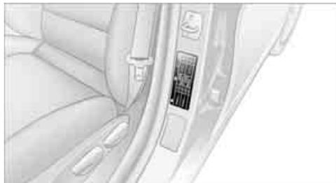
The inflation pressures for your factory-installed tires at ambient temperature can be found on the door post when you open the driver's door.
