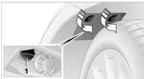
2. Apply gentle pressure to the bulb while turning it to the left for removal and replacement.
