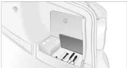
The onboard tool kit is stored in a compartment on the right-hand side of the luggage compartment. Remove the cover.
