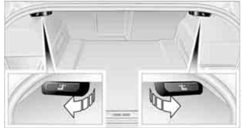
5. The unlocked rear seat back moves forward slightly. Fold the seat back forward by the head restraint.
