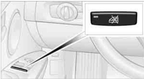
With the safety switch, you can prevent the rear windows from being opened or closed via the switches in the rear passenger area, by children, for example. When the safety function is switched on, the indicator lamp comes on.
