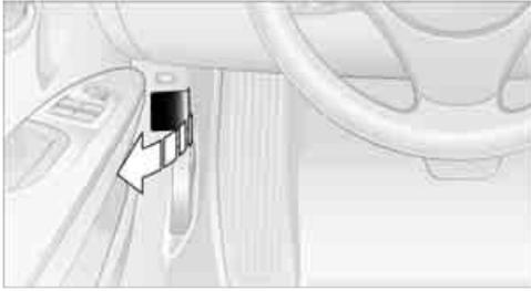
The Onboard Diagnostics OBD interface socket is located on the left of the driver's side under the instrument panel and under a cover.
