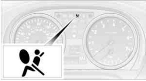
When the remote control is inserted into the ignition lock or the car is radio-ready, refer to page 49, the warning lamp comes on briefly to indicate that the entire airbag system and the belt tensioners are operational.
