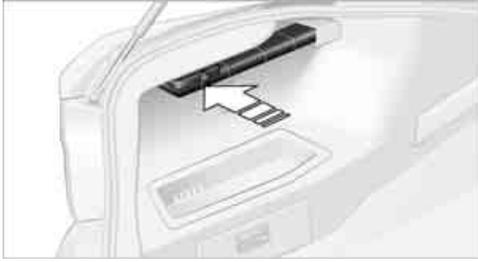
The warning triangle is on the left-hand side of the luggage compartment. Press the tab to take it out.
