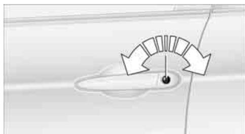
One turn of the key in the driver's door lock unlocks the driver's door only. Turning the key a second time unlocks all of the remaining doors, the luggage compartment lid and the fuel filler door.
