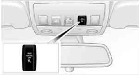
The indicator lamp located above the rearview mirror indicates whether the front passenger airbag system is active or not active/OFF.
