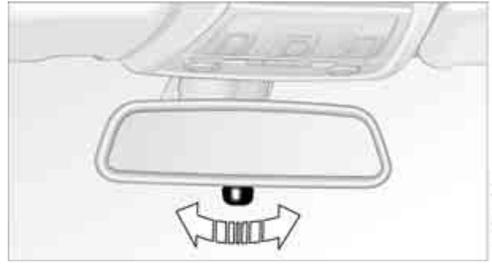
Turn the knob underneath the mirror to reduce glare from the headlamps of cars behind you when driving at night.
