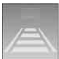
Distance 4 This distance is always set when the system is used for the first time after starting the engine.
