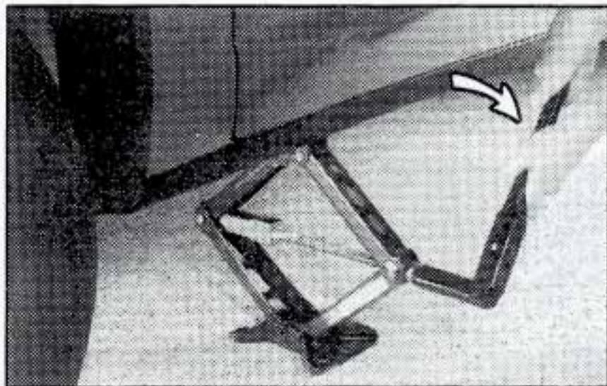
5. Raise the vehicle by rotating the wheel wrench to the right in the jack. Raise the vehicle far enough off the ground so there is enough room for the spare tire to fit.
