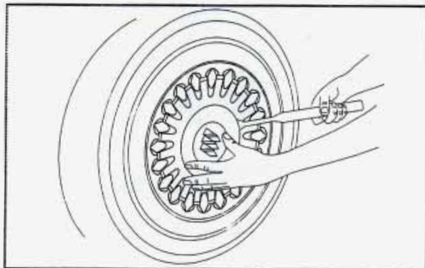
1. Insert the flat end of the wheel wrench in the notch and pry off the center cover. Do not drop the cover or lay it face down, as it could be scratched or damaged.
