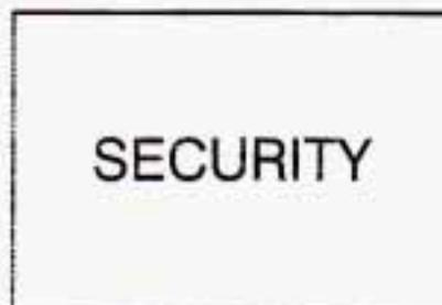
Your vehicle is equipped with a Content Theft-Deterrent alarm system. With this system, the SECURITY light will flash as you open the door (if your ignition is off).
