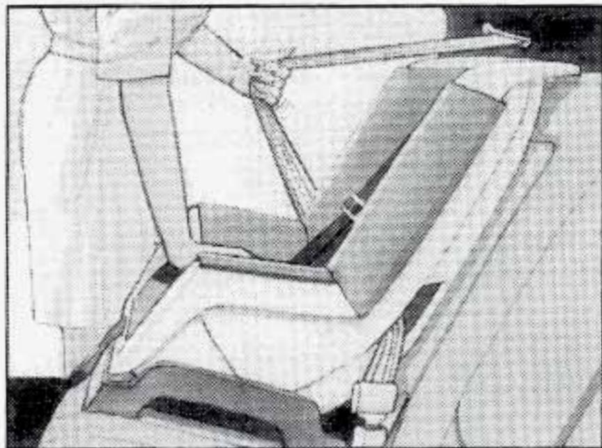
5. To tighten the belt, pull up on the shoulder belt while you push down on the child restraint. If you're using a forward-facing child restraint, you may find it helpful to use your knee to push down on the child restraint as you tighten the belt.
