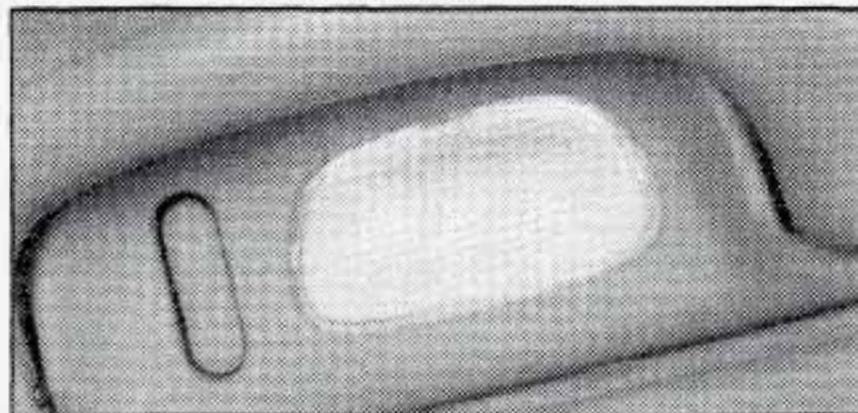
To turn on a rear seat reading lamp, press the switch above that rear door. To turn off the reading lamp, press the switch again.
