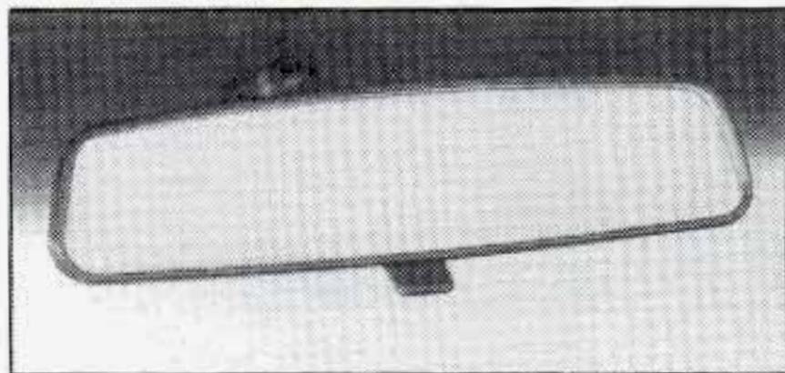
When you are sitting in a comfortable driving position, adjust the mirror so you can see clearly behind your vehicle. Grip the mirror in the center to move it up or down and side to side. The day/night adjustment allows you to adjust the mirror to avoid glare from the lamps behind you. Pull the tab forward for daytime use; push it back for night use.
