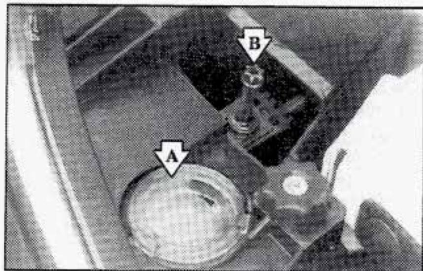
1. Check the vertical aim for each headlamp (A). The vehicle must be on a level surface. Turn the vertical aiming screw (B) until the bubble in the level is lined up with the 0 (zero).
