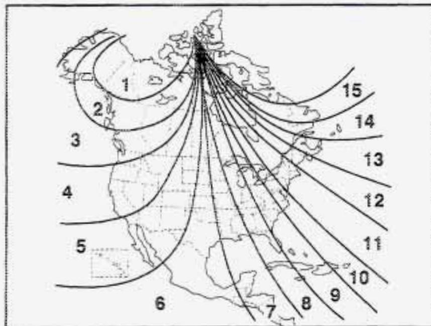
3. Press the COMPASS button on the bottom of the mirror until the new zone number appears in the display. After you stop pressing the button, the display will show a compass direction within a few seconds. (This is the automatic calibration mode. Drive in a circle to calibrate the mirror. See "Compass Calibration" following.)
