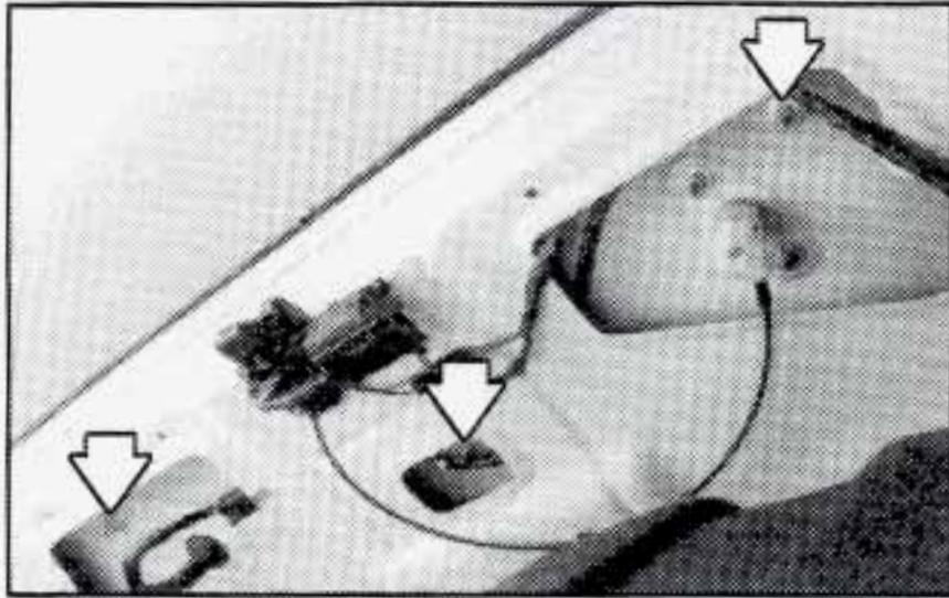
4. Hold the trunk trim back to expose the three remaining nuts holding the taillamp assembly in place.
