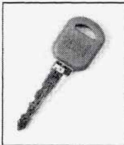
The valet key is used for the ignition and the two side doors only. It will not open the trunk or glove box. This is a theft-deterrent feature. The valet key should always be used when valet parking your vehicle.
