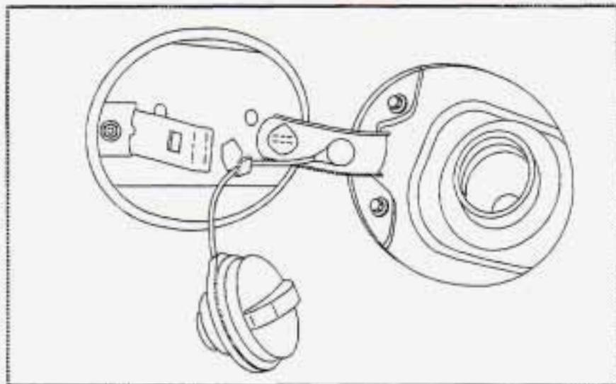
While refueling, hang the tethered cap on the fuel door latch. To remove the cap, turn it slowly to the left. The cap has a spring in it; if you let go of the cap too soon, it will spring back to the right.
