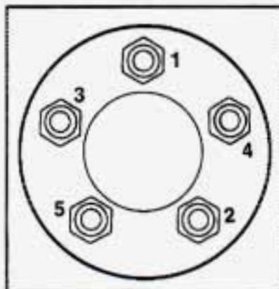
10. Using the wheel wrench, tighten the wheel nuts firmly in a crisscross sequence.
