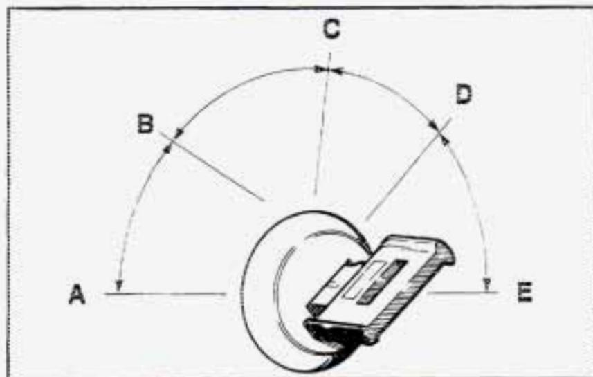
**ACCESSORY (A):** In this position you can operate your electrical power accessories. Press in the ignition switch as you turn the top of it toward you.
