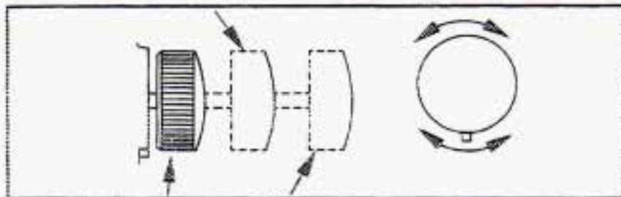
Pull the headlamp knob out to the first indent to turn on the parking lamps. Pull the knob out further, to the second indent to turn on the headlamps. Push the knob all the way back in to turn off the parking and headlamps.
