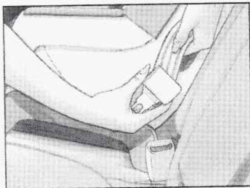
3. Tilt the latch plate to adjust the belt if needed.
