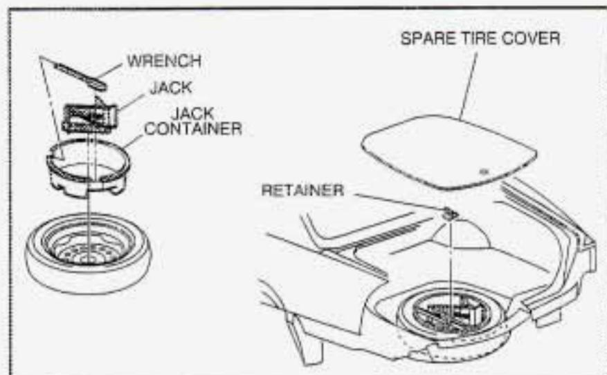
The compact spare tire is for temporary use only. Replace the compact spare tire with a full-size tire as soon as you can. See "Compact Spare Tire" later in this section.
