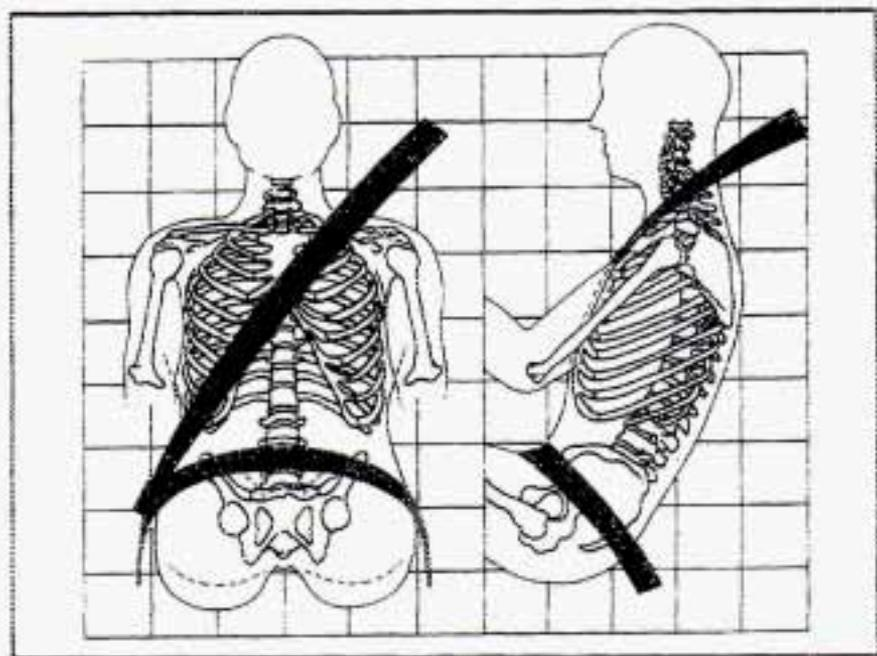
The lap part of the belt should be worn low and snug on the hips, just touching the thighs. In a crash, this applies force to the strong pelvic bones. And you'd be less likely
