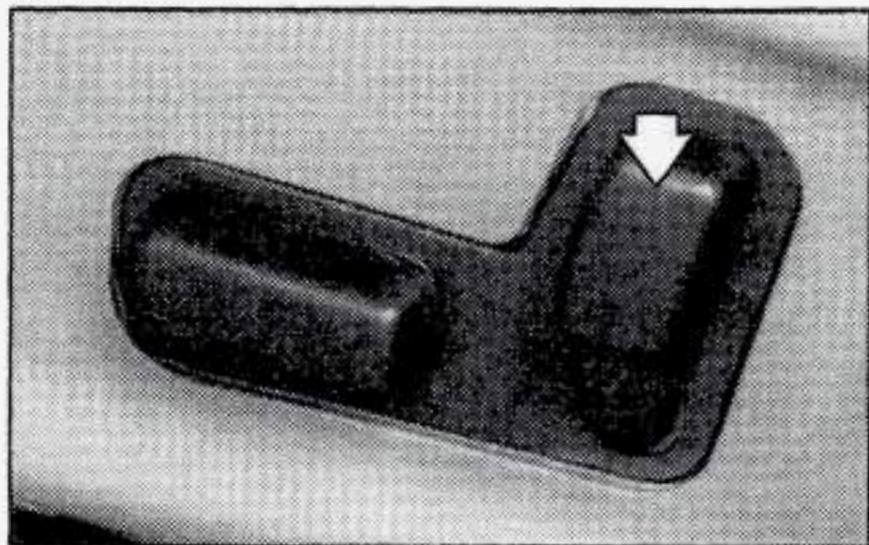
Use this switch to move a front head restraint up or down. Lift up on the switch to move the head restraint up. Press down on the switch to move the head restraint down. The top of the head restraint should be closest to the top of your ears. This position helps reduce the chance of a neck injury in a crash. When you move a front seat head restraint up or down, the shoulder belt height changes. On some models, the head restraints tilt forward and rearward also.
