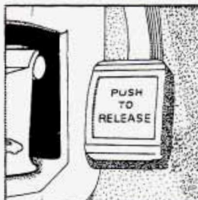
Your vehicle has a **PUSH TO RELEASE** parking brake pedal. To set the parking brake, hold the regular brake pedal down with your right foot. Push down the parking brake pedal with your left foot.
