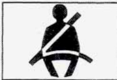
The safety belt light will also come on and stay on for about 20 seconds, then it will flash for about 55 seconds. If the driver's belt is already buckled, neither the chime nor the light will come on.
