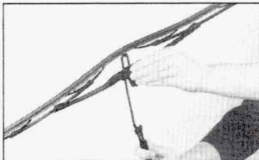
3. Push the tab on the wiper blade assembly and pull the assembly down enough to release it from the "U" hooked end of the wiper arm. Slide the assembly away from the arm.
