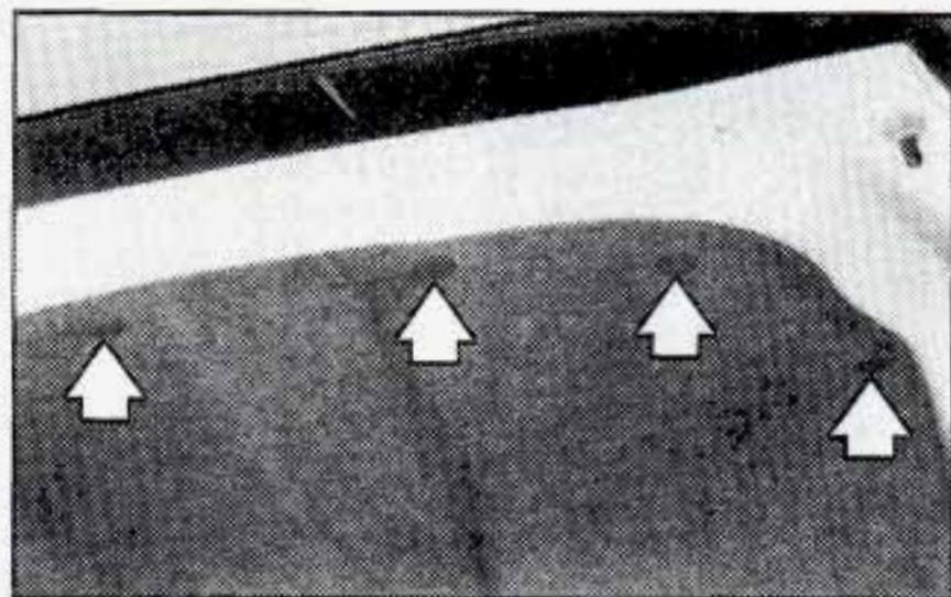
3. Next, there are eight fasteners along the top of the trunk lid (four on each side), holding the trunk trim in place. Remove these fasteners.
