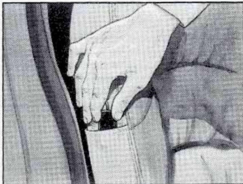
1. Remove the guide from its storage pocket on the side of the seatback.
