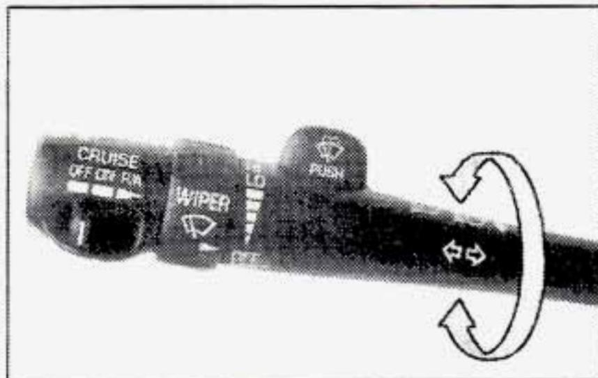
You control the windshield wipers by turning the band marked WIPER.
