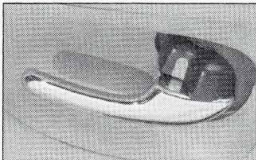
To lock the door from the inside, move the lock control on the door handle forward.
