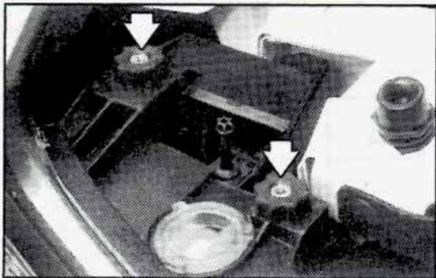
Each headlamp is attached by thumb screws.
