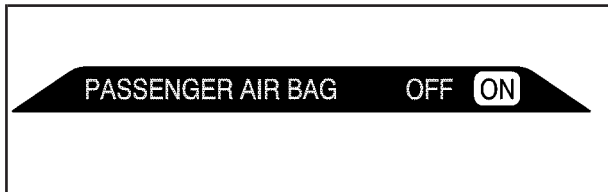
Passenger Airbag Status Indicator – United States
