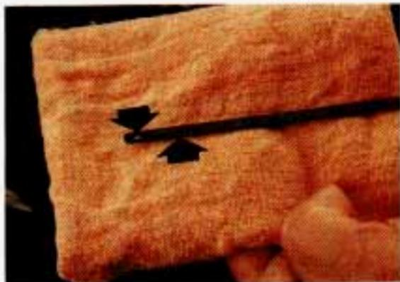
**When to Add Oil:** If the oil is at or below the ADD mark, you'll need to add some oil. But you must use the right kind. This section explains what kind of oil to use. For crankcase capacity, see "Capacities and Specifications" in the Index.
