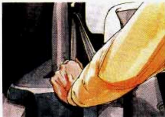
6. To tighten the belt, feed the shoulder belt into the retractor while you push down on the child restraint.
