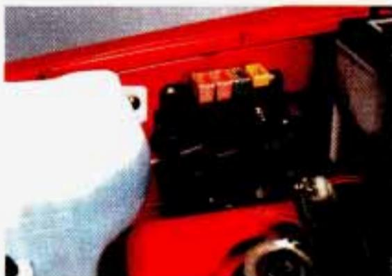
For access to the main fuses, pull off cover. A spare fuse is also inside the fuse box.
