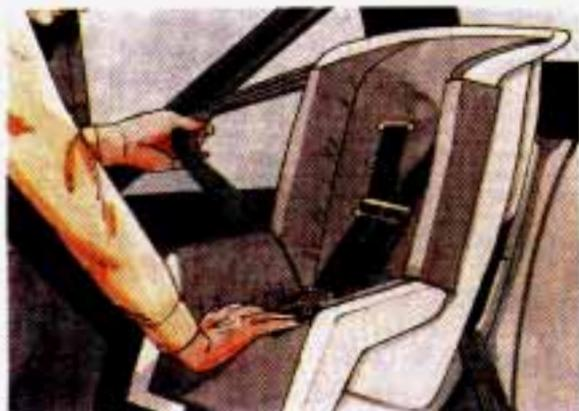
5. Pull the rest of the shoulder belt all the way out of the retractor to set the lock.
