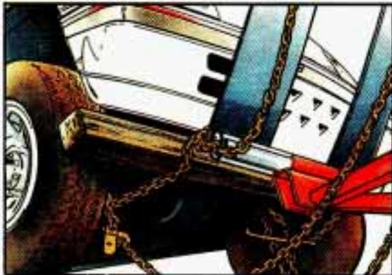
Position 4x4 wood beam across sling chains and against lower control arm front attachment brackets. Position the lower sling crossbar in front and against 4x4 wood beam.
