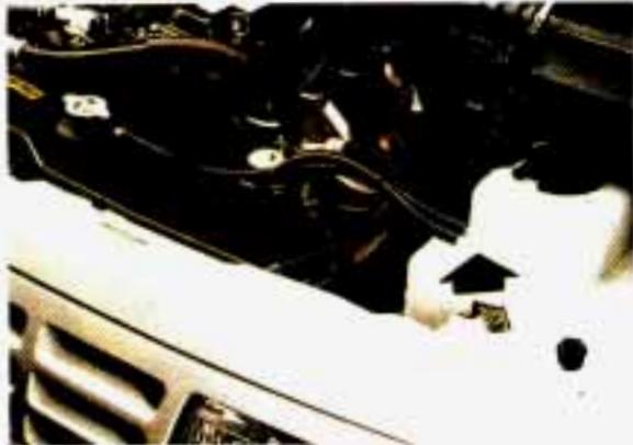
If the coolant inside the coolant recovery tank is boiling, don't do anything else until it cools down.
