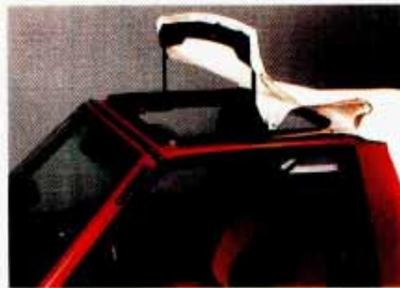
4. Swing the front top bow up and back while folding the canvas top out from between the top bow and the roof support. Be sure that you don't pinch the canvas top between the front top bow arms and the roof rails.
