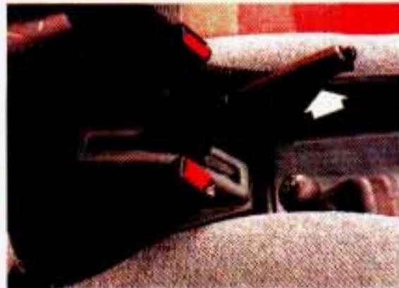
To set the parking brake: Hold the brake pedal down and pull up on the parking brake lever. If the ignition is on, the brake system warning light will come on.
