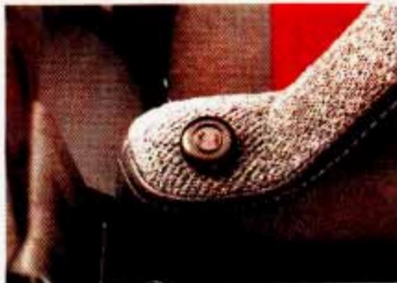
2. Pull the knobs on both sides of the seatback.
