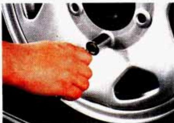
Insert your key into the wheel lock and pull the wheel lock off.
