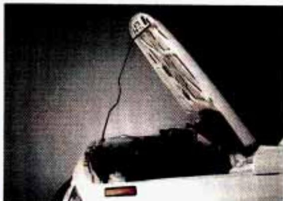
Lift the hood, release the hood prop from its retainer and put the hood prop into the slot in the hood.
