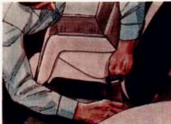
3. Pull out the vehicle's safety belt and run the lap part through or around the restraint. The child restraint instructions will show you how.
