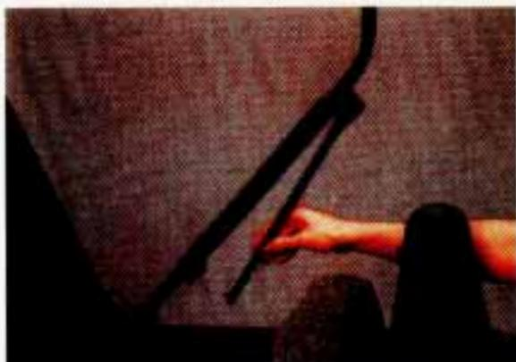
16. Pull up and back on the rear top bow struts and swing each strut forward.
