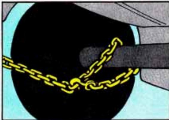
Attach a separate safety chain around the outboard end of each side of the rear axle.
