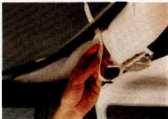
5. Unfasten the holding strap near the dome light and pull it through the slot in the front top bow.
