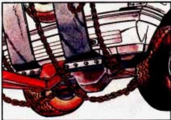
Position the sling crossbar under and forward of the rear bumper.
