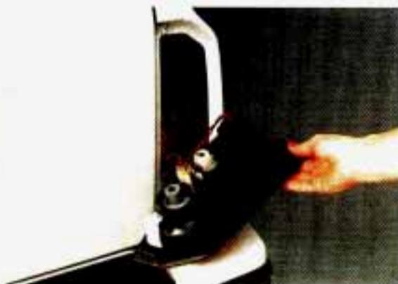
2. Pull the combination light out far enough to reach the bulb socket.
