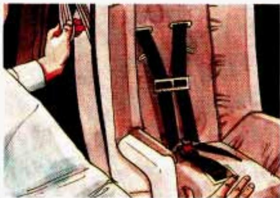
6. To tighten the belt, feed the shoulder belt back into the retractor while you push down on the child restraint.
