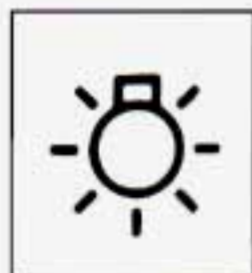
Master Lighting Switch
