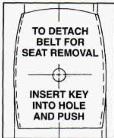
1. If you are removing the center seat, remove the right lap-shoulder belt. To do this, press the tip of a key into the release hole of the safety belt attachment while pulling up on the safety belt.
