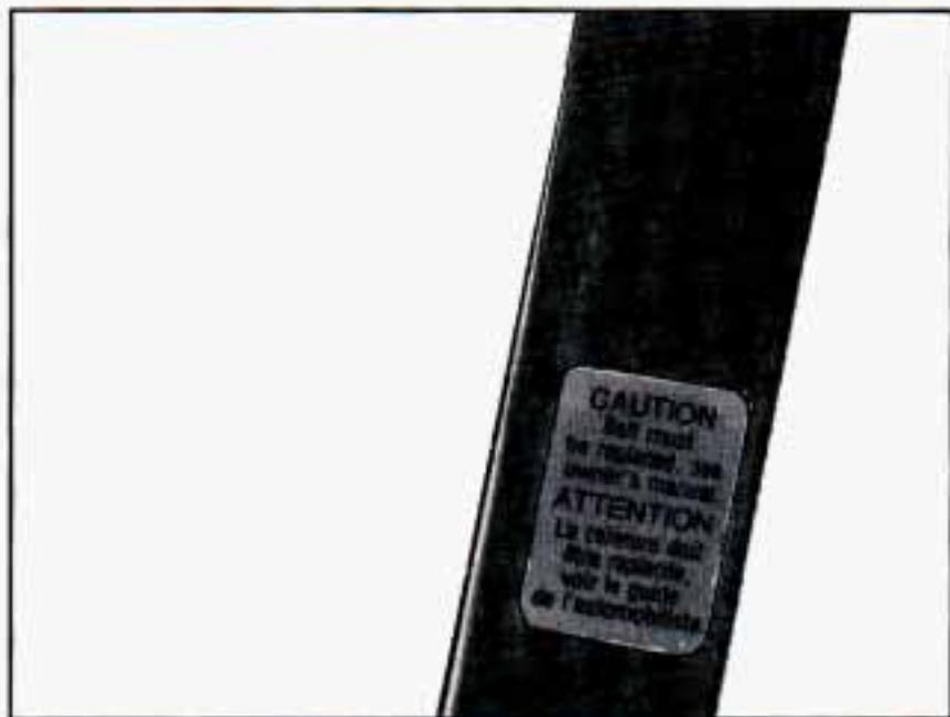
If you ever see a label on a right front safety belt that says to replace the belt, be sure to do so. Then the new belt will be there to help protect you in a collision. You would see this label on the belt near the latch plate.
