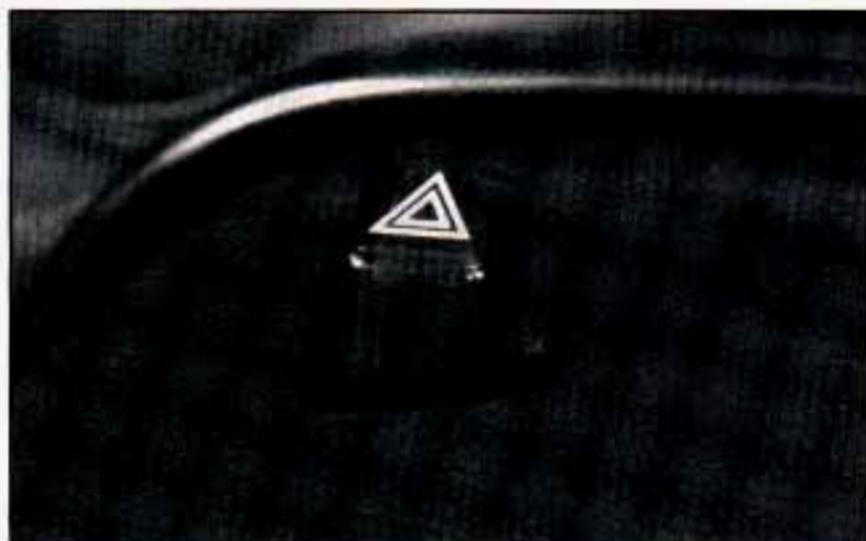
Press the button down to make your front and rear turn signal lamps flash on and off. Your hazard warning flashers work no matter what position your key is in, and even if the key isn't in.
