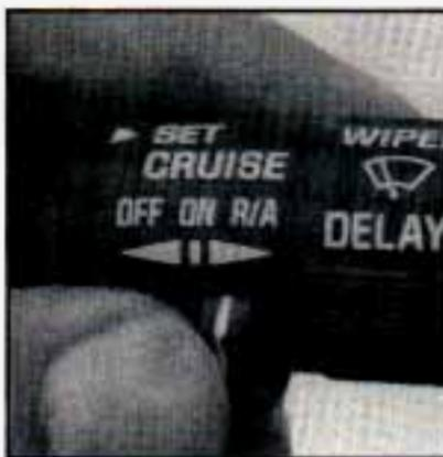
Once you're going about 25 mph (40 km/h) or more, you can move the cruise control switch from ON to R/A for about 1 1/2 seconds.
