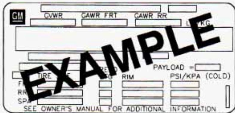
The Certification/Tire label is found on the rear edge of the driver's door. The label shows the size of your original tires and the inflation pressures needed to obtain the gross weight capacity of your vehicle.
