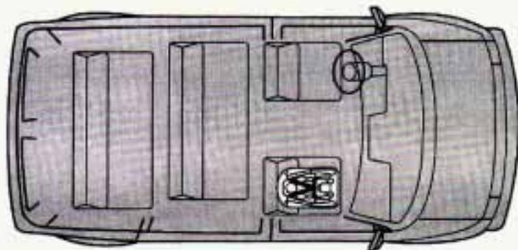
Your vehicle has a front passenger air bag. *Never* put a rear-facing child restraint in this seat. Here's why:
