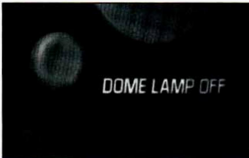
If the DOME LAMP OFF button is in the out position, your interior lamps will work as usual.
