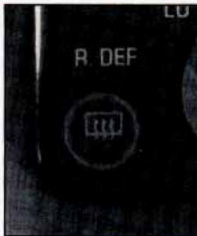
To turn on the rear window defogger, find the button to the left of the heater controls with the defog symbol on it.
