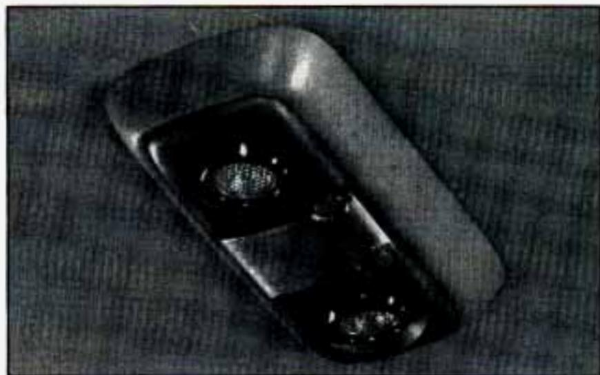
The dome lamps may come on when you open any of the doors. You can also turn on the dome lamps by turning the dimmer dial up until it clicks.
