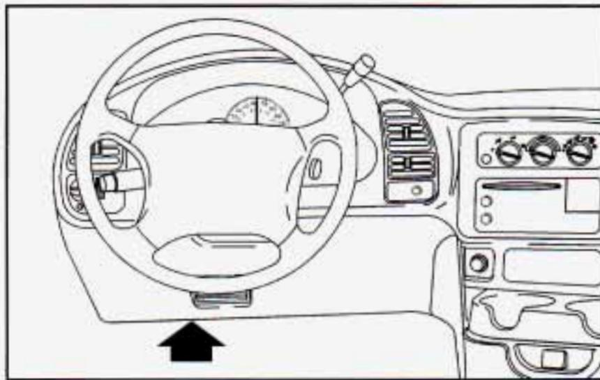
The fuse block is on the lower portion of the instrument panel on the driver's side.
