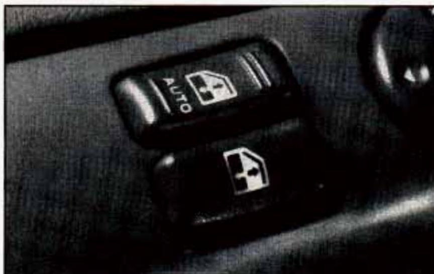
If you have the optional power windows, the controls are on each of the front side doors. The driver's door has a switch for the front passenger window as well. Your power windows will not move unless the ignition has been turned to the RUN position.
