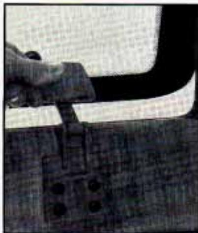
To open your swing-out windows, pull up on the latch and push the window out.
