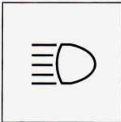
When the high beams are on, this indicator light on the instrument panel also will be on.
