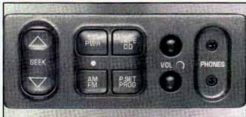
This feature allows rear seat passengers to listen to a different music source than the front seat passengers including AM-FM automatic tone control and cassette tapes. For example, rear seat passengers may listen to the cassette tape through headphones while the driver listens to the radio through the front speakers. The rear seat passengers have control of the volume for each headphone. Be aware that the front seat audio controls always override the rear seat audio controls.
