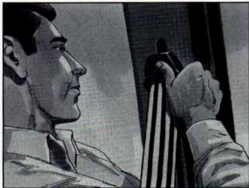
To move it down, push in at the top of the arrows and move the height adjuster to the desired position. You can move the adjuster up just by pushing up on the shoulder belt guide. After you move the adjuster to where you want it, try to move it down without pushing in to make sure it has locked into position.
