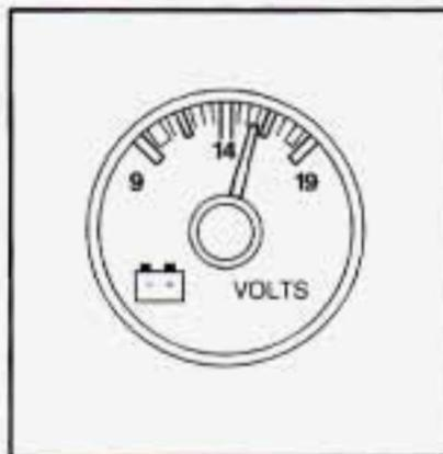
When your engine is not running, but the ignition is on (in the RUN position), the gage shows your battery's state of charge in DC volts.
