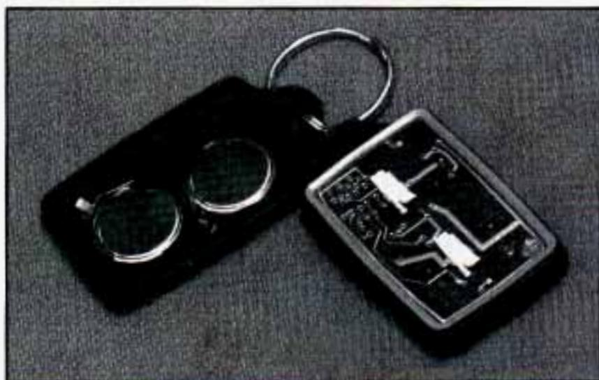
1. Insert a dime between two halves of the transmitter housing near the key ring hole.
