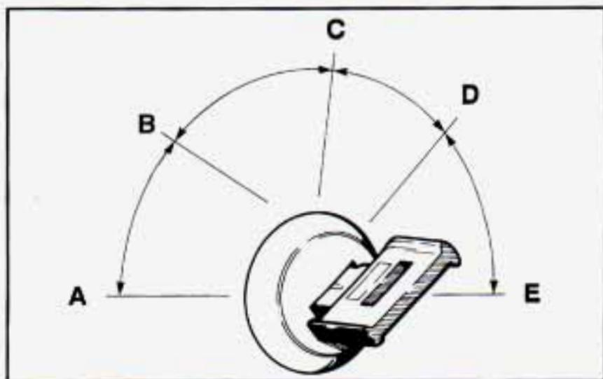
**ACCESSORY (A):** This position lets you use things like the radio and the windshield wipers when the engine is off. To get into ACCESSORY, push in the key and turn it toward you. Your steering wheel will remain locked, just as it was before you inserted the key.
