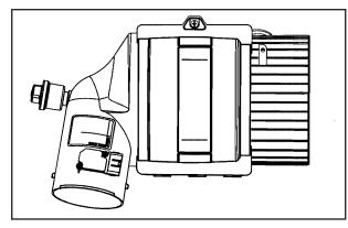
The air cleaner/filter assembly is located on the front corner of the engine compartment on the passenger's side of the vehicle.
