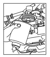
Unplug the water sensor wire connected to the fuel filter and unscrew the filter element.
