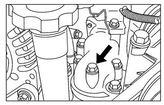
3. After the engine cools, open the air bleed valve on the thermostat housing.
