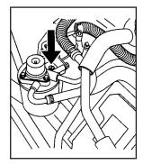
Open the fuel filter vent valve by turning the screw counterclockwise several full turns. The vent valve is located on top of the fuel filter housing.
