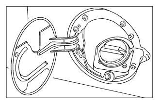
The fuel cap is located behind a hinged door on the driver's side of the vehicle.
