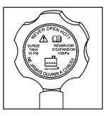
The surge tank pressure cap must be tightly installed.
