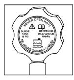
Park the vehicle on a level surface. You can remove the coolant surge tank pressure cap when the cooling system, including the coolant surge tank pressure cap and upper radiator hose, is no longer hot.
