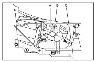
When the engine is cold, the coolant level should be at or above the COLD FILL mark.
