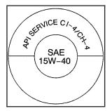
This doughnut-shaped logo (symbol) is used on most oil containers to help you select the correct oil. It means that the oil has been certified by the American Petroleum Institute.
