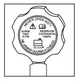
1. You can remove the coolant surge tank pressure cap when the cooling system, including the coolant surge tank pressure cap and upper radiator hose, is no longer hot. Turn the pressure cap slowly counterclockwise about one full turn.
