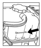
The coolant level should be at or above the FULL COLD mark. If it isn't, you may have a leak at the pressure cap or in the radiator hoses, heater hoses, radiator, water pump or somewhere else in the cooling system.
