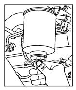
4. For pickup models, open the drain valve by turning it two to three turns. When fuel empties from the valve, all the water has been drained. Close the valve hand tight. To help remove all the water, press the priming pump several times.
