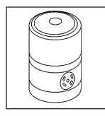
The air cleaner/filter assembly may have an air cleaner/filter restriction indicator that lets you know when the engine air cleaner/filter is dirty and needs to be serviced.
