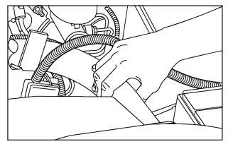
7. With the coolant surge tank pressure cap off, start the engine and let it run until you can feel the upper radiator hose getting hot. Watch out for the engine cooling fan.
