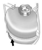
Fill the coolant surge tank with the proper DEX-COOL coolant mixture, to the COLD FILL line.  With the coolant surge tank pressure cap off, start the engine and let it run until the upper radiator hose can be felt getting hot. Watch out for the engine cooling fan(s).
