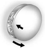
The fuel cap is behind the fuel door on the passenger side of the vehicle. To open the fuel door, push and release the rearward center edge of the door.
