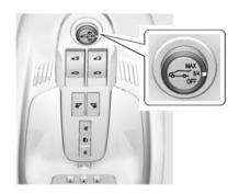
If equipped, the power liftgate switch is on the overhead console. The vehicle must be in P (Park) to operate. The taillamps flash when the power liftgate moves.
