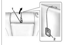
Stow the rear seat center armrest. Attach the retaining strap to the armrest loop (1) and to the center top tether anchor on the seatback (2). Make sure the retaining strap's clips are firmly attached.
