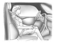
If a person of adult size is sitting in the front outboard passenger seat, but the off indicator is lit, it could be because that person is not sitting properly in the seat. If this happens, use the following steps to allow the system to detect that person and enable the front outboard passenger frontal airbag:
