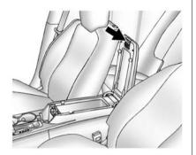
There is storage in the center console; lift the lever on the front to open. There may be a USB port and auxiliary input jack inside.
