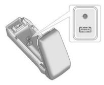
This jack is not an audio output. Do not plug headphones into the auxiliary input jack. Drivers are encouraged to set up any auxiliary device while the vehicle is in P (Park).
