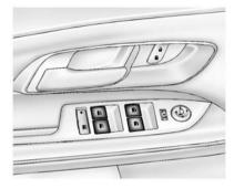
The power windows work when the ignition is in ON/RUN or ACC/ACCESSORY, or in Retained Accessory Power (RAP). See Retained Accessory Power (RAP) on page 9-22.
