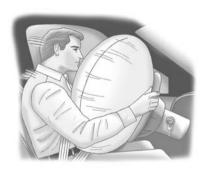
The driver frontal airbag is in the middle of the steering wheel.
