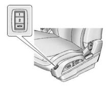
If available, the "1," "2," and MEM (Memory) buttons on the outboard side of the driver seat are used to manually save and recall the driver seat and outside mirror positions. These manually stored positions are referred to as Button Memory positions.
