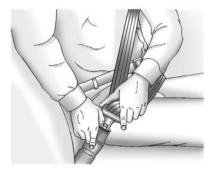
To unlatch the belt, push the button on the buckle.
