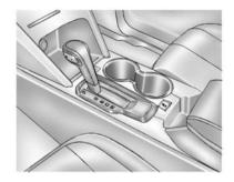
**P (Park):** This position locks the front wheels. Use P (Park) when starting the engine because the vehicle cannot move easily.
