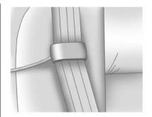
Be sure that the belt is not twisted and it lies flat. The elastic cord must be behind the belt with the plastic guide on the front.
