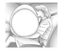
The front outboard passenger frontal airbag is in the instrument panel on the passenger side.
