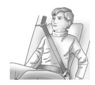
Buckle, position, and release the safety belt as described previously in this section. Make sure the shoulder portion of the belt is on the shoulder and not falling off of it. The belt should be close to, but not contacting, the neck. To remove and store the comfort guide, squeeze the belt edges together so that the safety belt can be removed from the guide. Slide the guide back into its storage pocket located on the side of the seatback.
