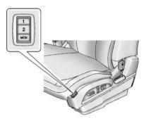
If available, the "1," "2," and MEM (Memory) buttons on the outboard side of the driver seat are used to manually save and recall the driver seat and outside mirror positions. These manually stored positions are referred to as Button Memory positions.
