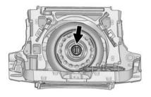
4. Turn the retainer nut counterclockwise and remove the spare tire.
