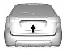
To open the liftgate, press the touch pad under the liftgate handle and lift up.
