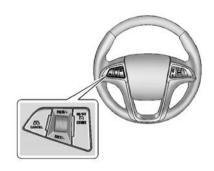
CRUSE: Press to turn the cruise control system on and off.
