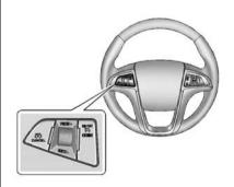
CRUISE (On/Off): Press to turn cruise control on or off.
