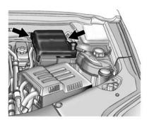
To remove the fuse block cover, squeeze the clips on the cover and lift it straight up. See Engine Compartment Overview on page 10-5.
