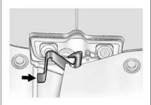
Go to the front of the vehicle to find the secondary hood release handle. The handle is under the front edge of the hood near the center. Push the handle to the right and at the same time raise the hood.
