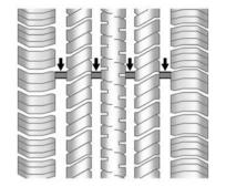
Treadwear indicators are one way to tell when it is time for new tires. Treadwear indicators appear when the tires have only 1.6 mm (1/16 in) or less of tread remaining. See *Tire Inspection on page 10-49* and *Tire Rotation on page 10-49*.
