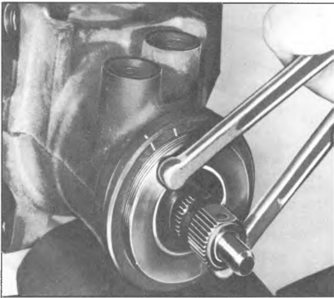
Fig. 3B-40--Align Hole With Second Mark
