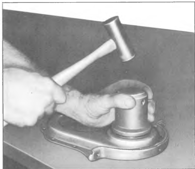
Fig. 6A-42V--Installing Oil Seal (Cover Removed)
