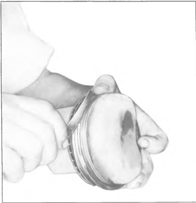
Fig. 6A-68--Measuring Ring Groove Clearance
