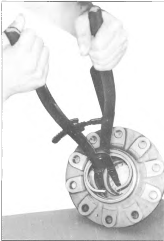
Fig. 4B-37-Removing Hub Outer Bearing Retainer Ring
