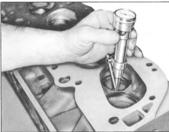
Fig. 6A-28--Measuring Valve Seat Concentricity (Typical)
