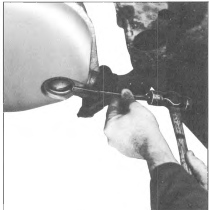
Fig. 6F-5--Removing Pressed Plug
