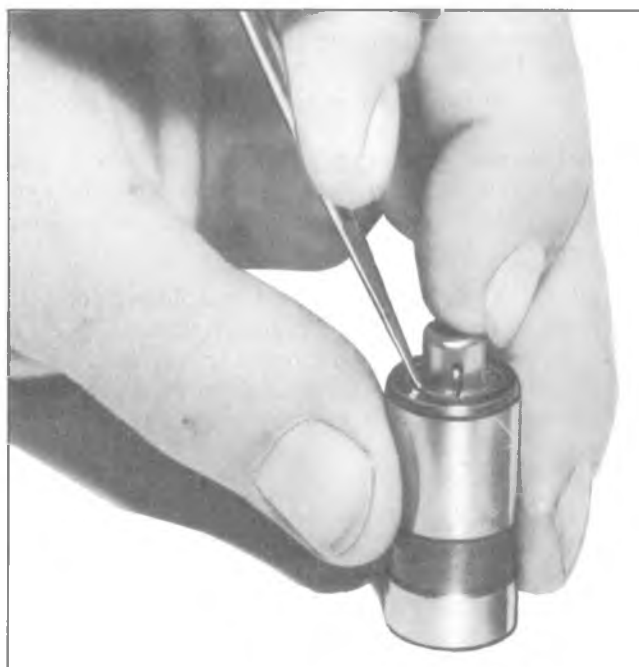
Fig. 6A-19V--Installing Ball Check Valve
