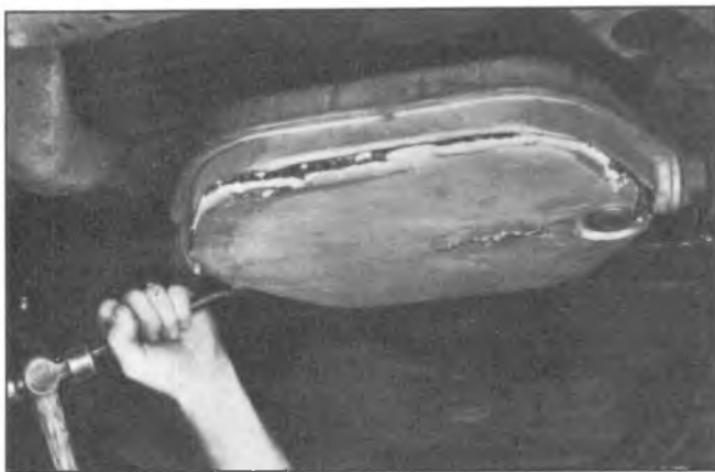
Fig. 6F-14--Removing Bottom Cover
