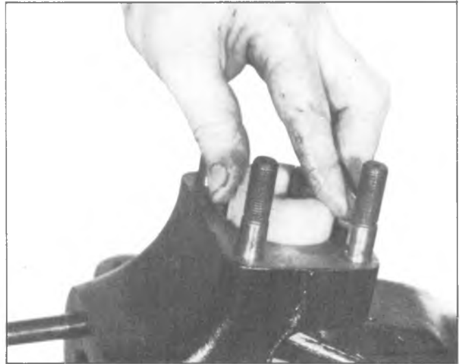
Fig. 3C-21K--Removing Tapered Bushing
