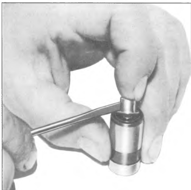
Fig. 6A-18V--Removing Ball Check Valve
