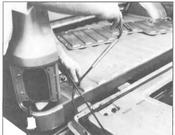
Fig. 2D-66--Removing Torque Rod (14)
