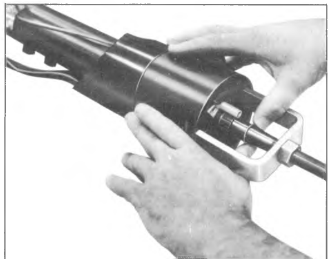
Fig. 3B-55-Installing Snap Ring
