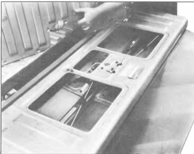
Fig. 2D-64--Removing Access Cover (14)
