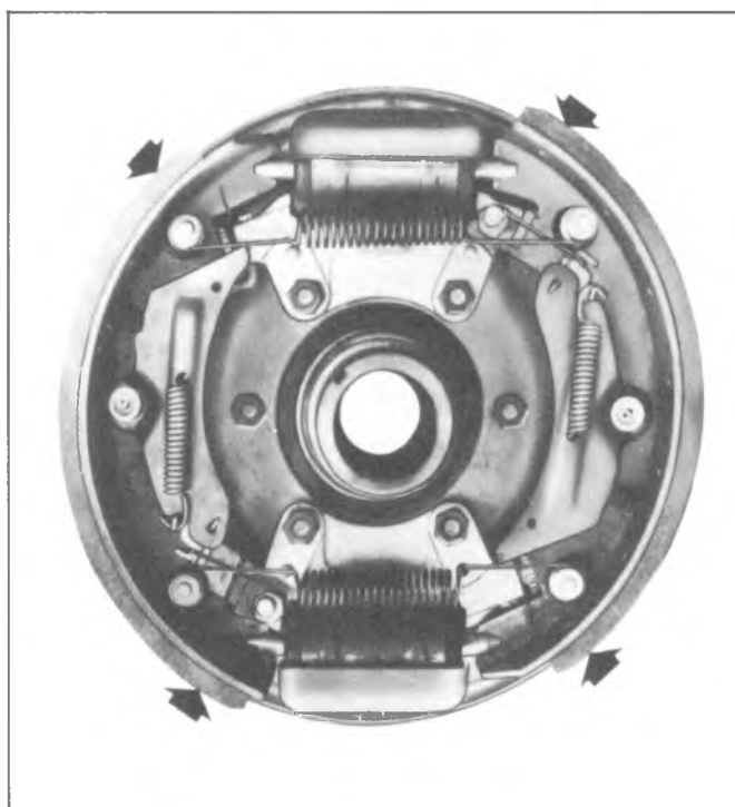
Fig. 5-51-Measuring Points for Shoe Centering
