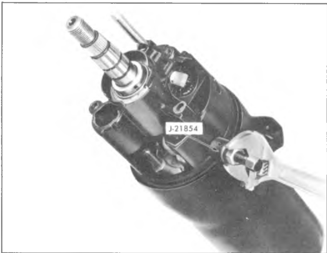
Fig. 3B-77--Removing Bearing Housing Pivot Pins
