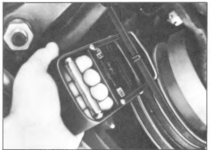
Fig. 3B-42--Checking Belt Tension with J-23600
