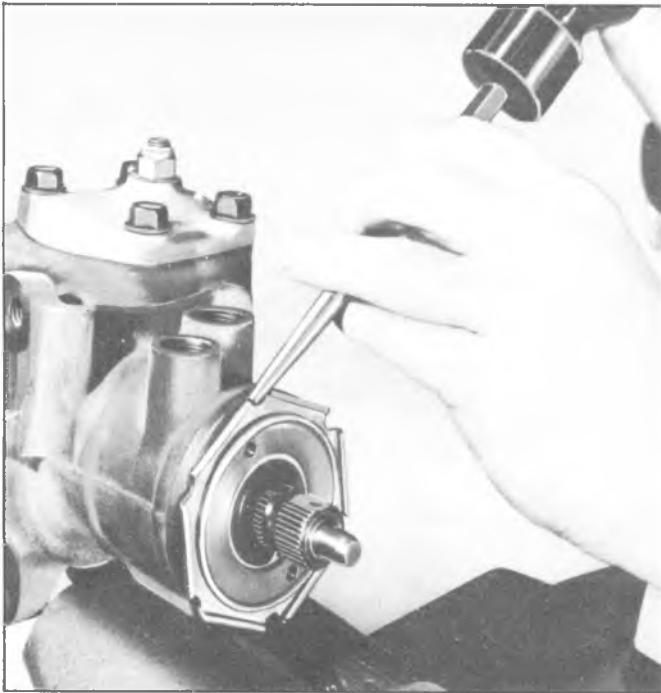
Fig. 3B-35--Loosening Lock Nut
