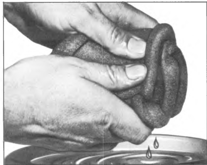
Fig. 6E-26--Cleaning Polywrap Band
