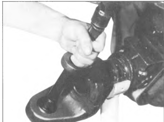
Fig. 3C-23K--Removing Cup, Cone and Seal
