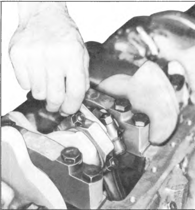
Fig. 6A-58V--Measuring Connecting Rod Side Clearance
