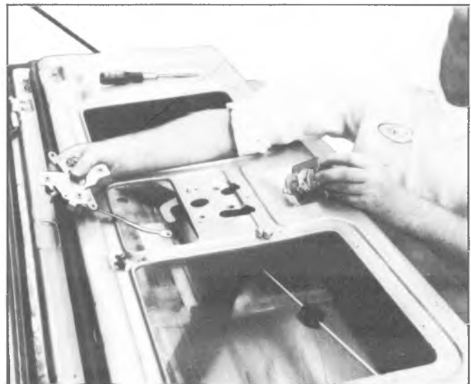
Fig. 2D-70--Removing Control Assembly and Inside Handle
