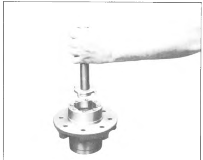
Fig. 4B-33-Removing Outer Bearing and Cup
