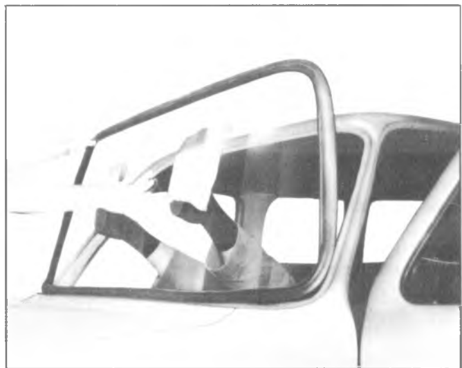
Fig. 2D-16--Removing Windshield from Opening
