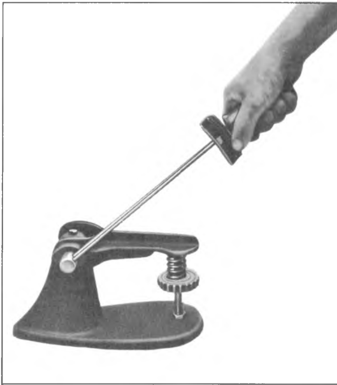
Fig. 6A-26V-Checking Valve Spring Tension
