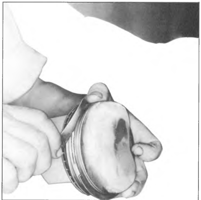
Fig. 6A-75V--Measuring Ring Groove Clearance
