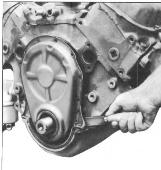
Fig. 6A-39V--Cutting Tabs on Oil Pan Front Seal
