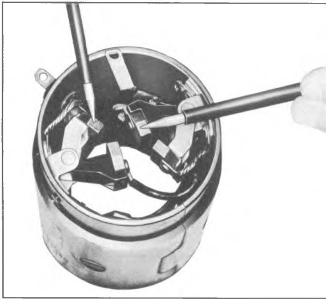
Fig. 6D-21S--Field Coil Ground Test
