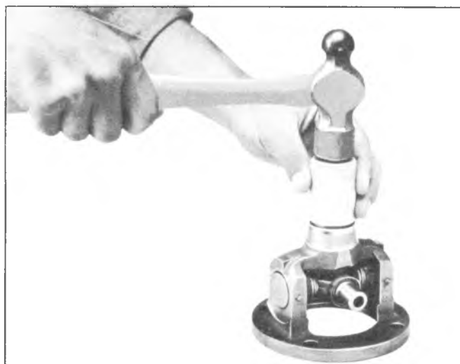
Fig. 4A-32--Installing Centering Ball Seal
