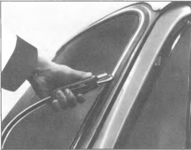
Fig. 2D-19--Installing Reveal Molding
