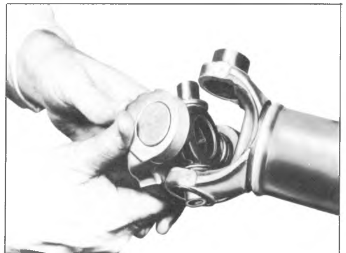
Fig. 4A-15--Installing Trunnion into Yoke
