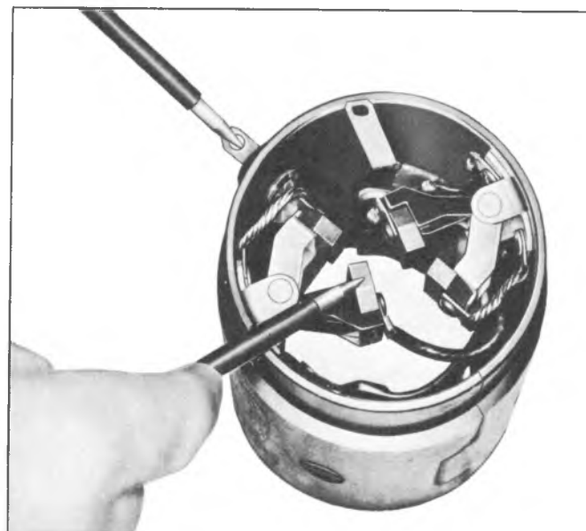
Fig. 6D-20S--Field Coil Open Circuit Test
