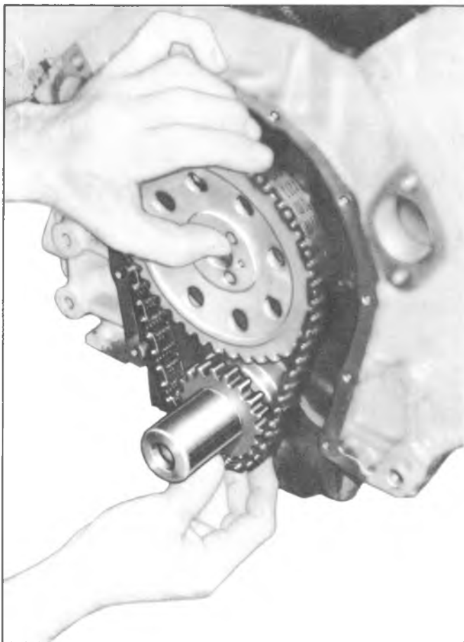
Fig. 6A-48V-Installing Timing Chain
