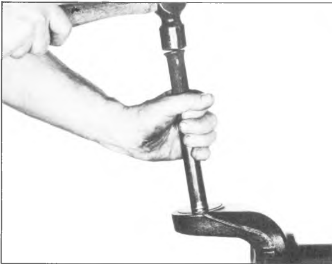
Fig. 3C-24K--Installing Grease Retainer
