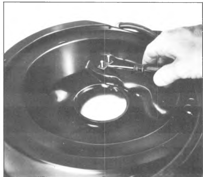
Fig. 6E-36--Removing Sensor Unit
