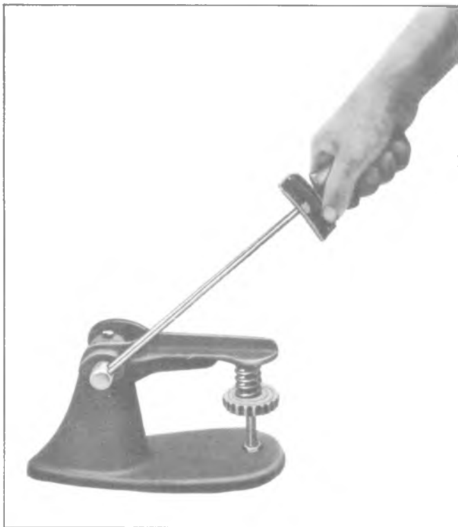
Fig. 6A-22--Checking Valve Spring Tension
