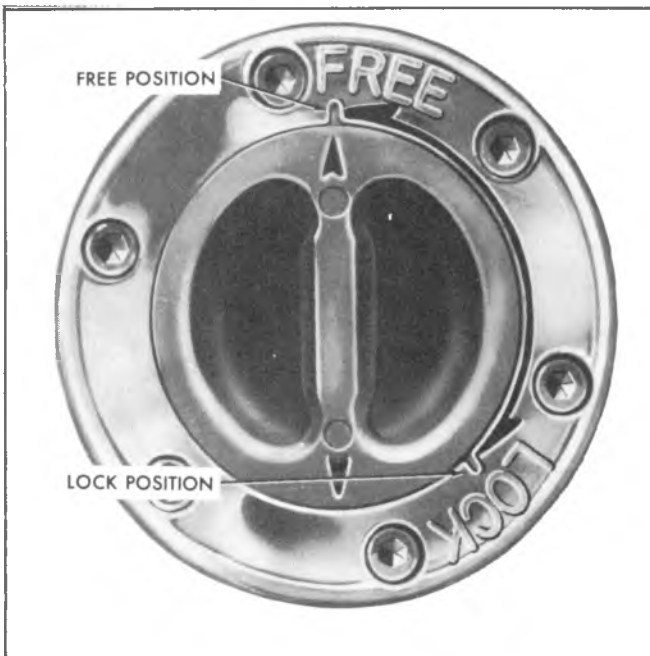
Fig. 3C-5K--Hub Key Position - Typical
