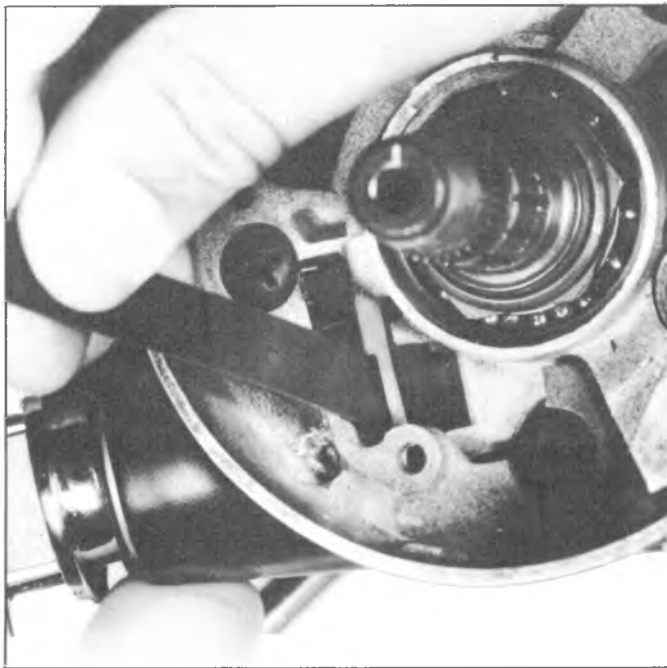
Fig. 3B-56--Lock Cylinder Removal
