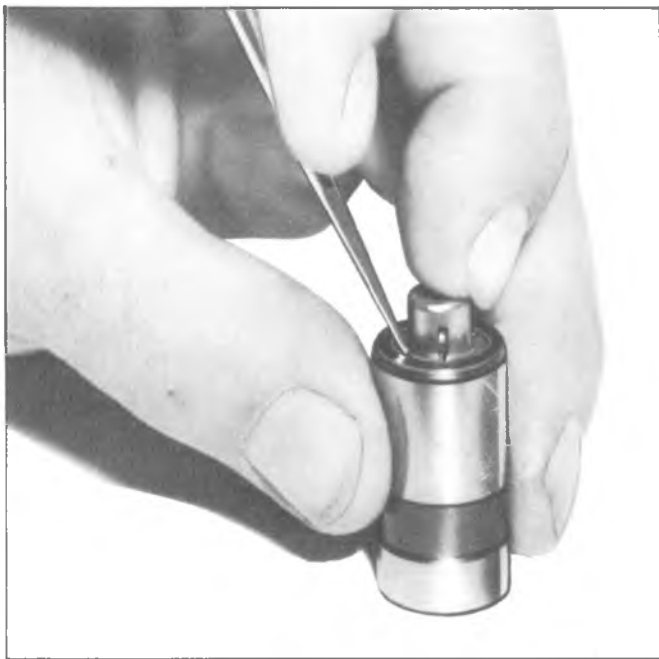
Fig. 6A-16--Installing Ball Check Valve
