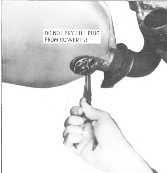
Fig. 6F-6--Removing Pressed Plug With Pliers
