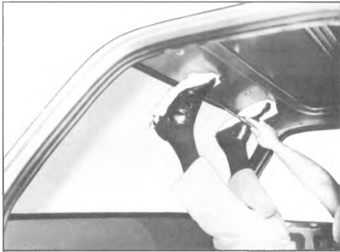
Fig. 2D-14--Applying Pressure to Windshield
