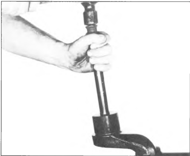
Fig. 3C-25K--Installing Oil Seal
