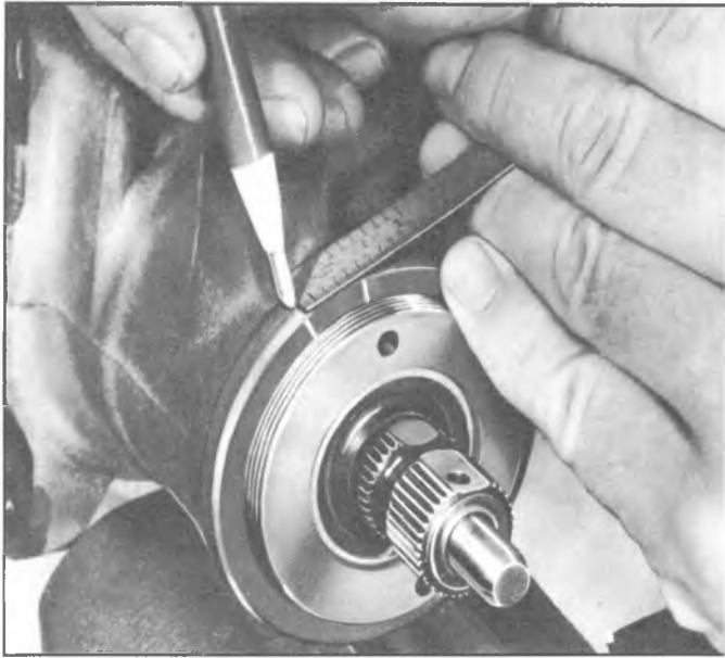
Fig. 3B-39--Measure Back and Remark Housing
