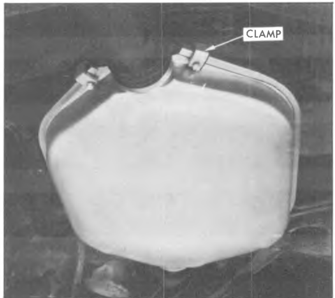
Fig. 6F-20--Installing Bottom Cover Clamps
