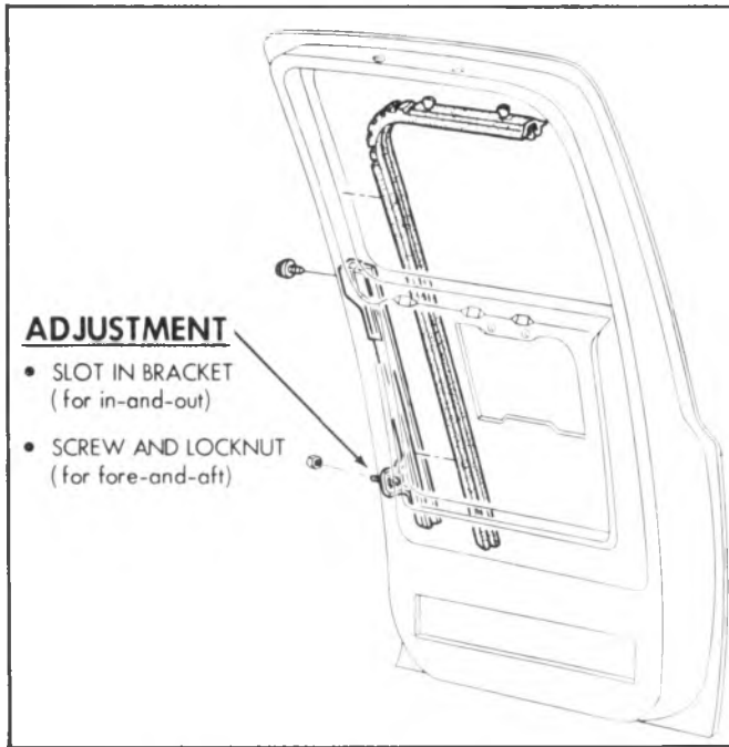
Fig. 2D-44--Glass Run Channel Adjustment
