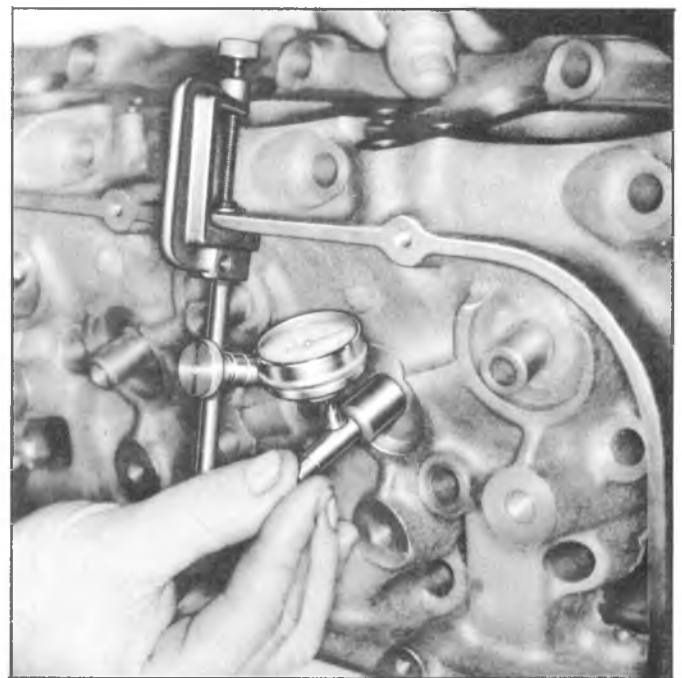
Fig. 6A-21--Measuring Valve Stem Clearance (Typical)
