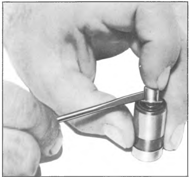
Fig. 6A-15--Removing Ball Check Valve
