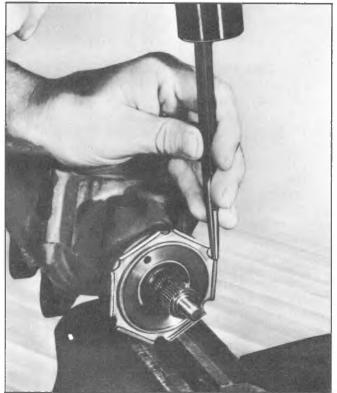
Fig. 3B-41--Tighten Lock Nut
