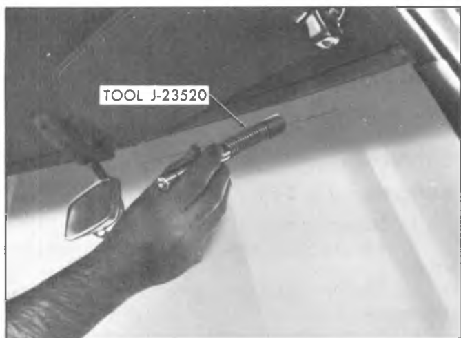
Fig. 9-1R--Testing Windshield Antenna (Typical)
