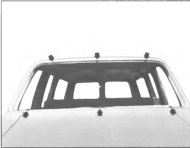
Fig. 2D-17-Checking Windshield Opening
