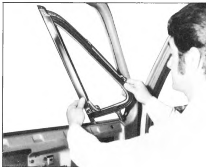
Fig. 2D-28--Removing Ventilator Assembly
