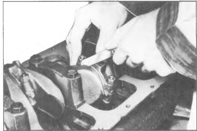
Fig. 6A-50--Measuring Connecting Rod Side Clearance
