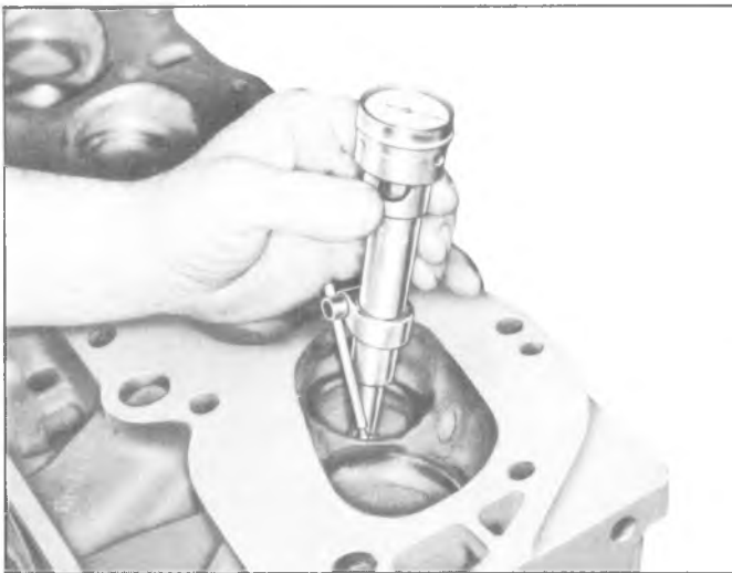
Fig. 6A-36V--Measuring Valve Seat Concentricity
