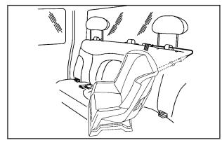
2.1. When using a child restraint with a top tether in the rear driver's side position, raise the head restraint and route the top tether through the fabric loop and under the center shoulder belt. Then, attach the top tether to the metal anchor point at the center rear seating position.
