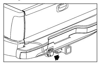
For vehicles equipped with heavy duty trailering, the harness is connected to the trailer mounted to the hitch platform. The eight-wire harness contains the following trailer circuits:
