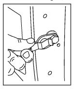
Raise the tailgate slightly and release both retaining cable clips. To release the retaining cable clips, lift the cable so it points straight out and push the cable clip forward.
