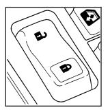
If your vehicle has this power door lock switch, press the raised side of the switch, with the lock symbol, on either front door to lock all the doors at once.
