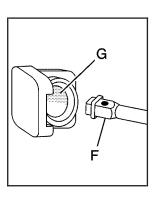
Insert the hoist end (F) through the hole (G) in the rear bumper and into the hoist shaft.
