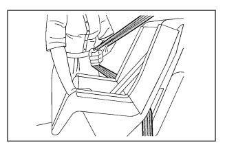
Pull the rest of the shoulder belt all the way out of the retractor to set the lock.
