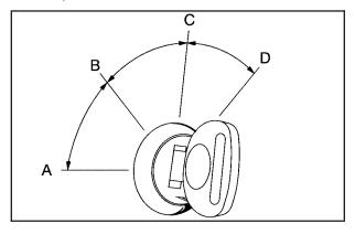
Notice: Using a tool to force the key from the ignition switch could cause damage or break the key. Use the correct key and turn the key only with your hand. Make sure the key is all the way in. If it is, turn the steering wheel left and right while you turn the key hard. If none of this works, then your vehicle needs service.
