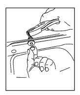
While continuing to pull downward on the push-pin, squeeze and turn the expandable end of the push-pin with a tool until it releases from the retainer.
