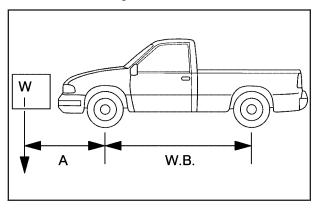
(W x (A + W.B.)) /W.B.= Weight the accessory is adding to the front axle.
