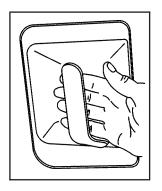
To open a rear access door from the inside, the front door must be opened first. Then, use the handle located on the inside of the rear access door to open it.
