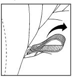
Pull up on the strap loop at the rear of the seat cushion. Then, pull the seat cushion up and flip it forward.  After folding the seat cushion fully forward, pull the seatback forward until it is flat. If the seatback cannot fold flat because it interferes with the cushion, try moving the front seat forward and/or bringing the front seat more upright. The lever at the base of the seat must be turned rearward to release the seatback.
