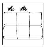
(Top Tether Anchor): Seating positions with top tether anchors. Do not install a child restraint in the center seat position. See Securing a Child Restraint in the Center Front Seat Position on page 1-56 for more information.
