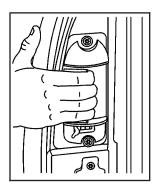
To open a rear access door from the outside, first open the front door.
