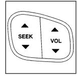
If your vehicle has this feature, some audio controls can be adjusted at the steering wheel. They include the following:
