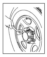
If your vehicle has wheel nut caps, loosen them by turning the wheel wrench counterclockwise.
