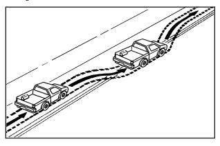
If the level of the shoulder is only slightly below the pavement, recovery should be fairly easy. Ease off the accelerator and then, if there is nothing in the way, steer so that your vehicle straddles the edge of the pavement. You can turn the steering wheel up to one-quarter turn until the right front tire contacts the pavement edge. Then turn your steering wheel to go straight down the roadway.
