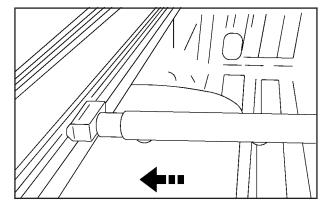
Remove the three bows by gently pushing them against the spring-loaded end. The three bows are labeled front, center, rear to remind you of the order in which to reinstall them.
