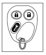
button once to unlock the driver's door. The interior lamps will come on. Pressing unlock again within three seconds will cause the remaining doors to unlock.
