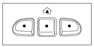
The Universal Home Remote System, a combined universal transmitter and receiver, provides a way to replace up to three hand-held transmitters used to activate devices such as gate operators, garage door openers, entry door locks, security systems, and home lighting.
