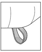
Push down on the front of the seat cushion while pulling down on the release strap which is located under the seat cushion.
