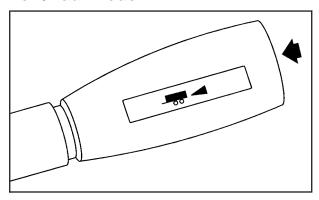
If your vehicle has an automatic transmission, it may have a Tow/Haul mode. If your vehicle has an Allison Transmission® see "Tow/Haul Mode (Allison Transmission®) following. Tow/Haul mode adjusts the transmission shift pattern to reduce shift cycling, providing increased performance, vehicle control, and transmission cooling when towing or hauling heavy loads.
