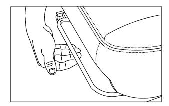
If your vehicle has a manual bucket or a split bench seat, you can adjust the seat forward or rearward with the bar located under the front of the seat cushion.
