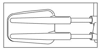
If your vehicle is equipped with this style camper-type mirrors, they can be adjusted so you can have a clear view of the objects behind you.
