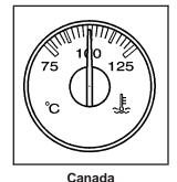
This gage shows the engine coolant temperature.
