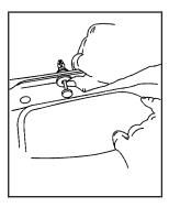
Line up each push-pin with its intended retainer and push the washer portion of the push-pin toward the retainer until it locks into place.
