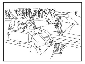
As you brake, your computer keeps receiving updates on wheel speed and controls braking pressure accordingly.
