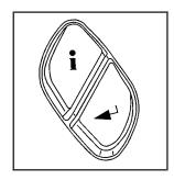
(Trip Information): Press this button to display the odometer, trip odometers, timer, engine hours, and selected range if your vehicle has an Allison Transmission®.
