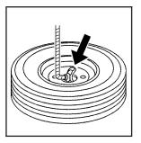
Tilt the retainer downward and through the wheel opening. Make sure the retainer is fully seated across the underside of the wheel.
