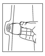
Your vehicle may have swing-out windows. To open a rear swing-out window, flip the latch open and swing the glass out.
