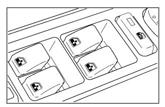
If your vehicle is equipped with power windows, the controls are located on each of the side doors in the front and rear for crew cab models.
