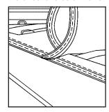
To remove, unsnap the cover. Roll it up and stow it using the buckle and the strap located at the front of the box.
