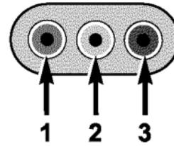
Audio/Video RCA Jacks (AUX Jacks) on the rear of the center console enable the monitor to display video directly from a video camera, connect video games for display on the screen, or play music directly from an MP3 player.
