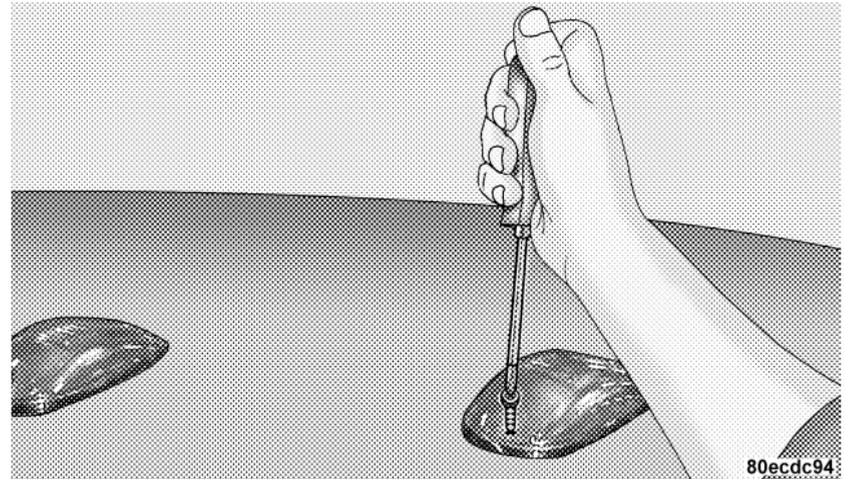
2. Rotate the socket  $\frac{1}{4}$  turn and pull it from the light assembly.
