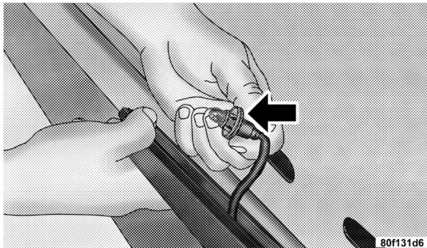
3. Pull bulb straight out from socket.
