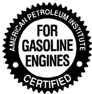
This symbol means that the oil has been certified by the American Petroleum Institute (API). The manufacture only recommends API Certified engine oils that meet the requirements of DaimlerChrysler Material Standard MS-6395. Use Mopar or an equivalent oil meeting the speci-
