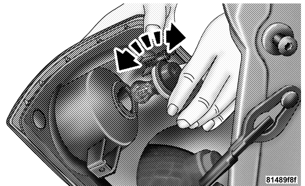
Rotating Bulb Socket From Housing
