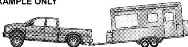
**FIG. 1 WITHOUT WEIGHT DISTRIBUTION (INCORRECT)**
