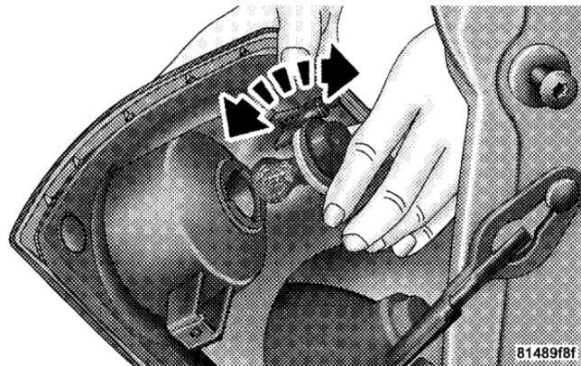
**Rotating Bulb Socket From Housing**
