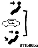
Select the recirculation modes when the outside air contains smoke, odors, high humidity, or if rapid cooling is desired. This feature allows for recirculation of interior air only. Air flows through the panel only or through both the panel and floor vents depending on the selected mode (panel vs bi-level).
