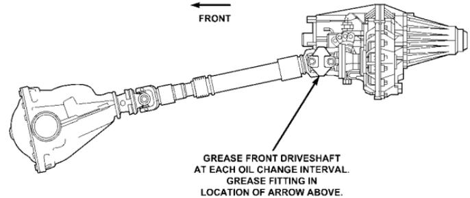
Front Driveshaft Grease Fitting
