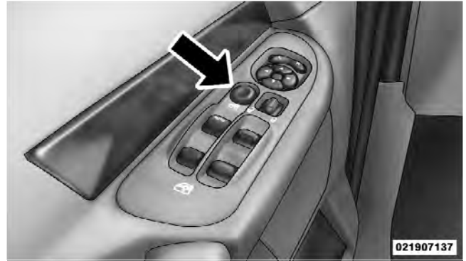
Window Lockout Switch
