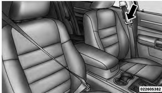
Pulling Out the Lap/Shoulder Belt Latch Plate
