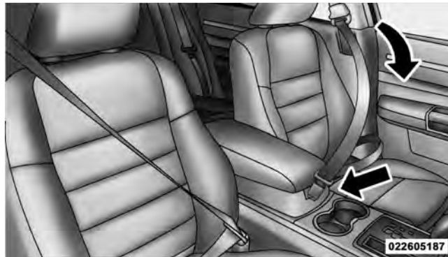
Removing Slack from Belt
