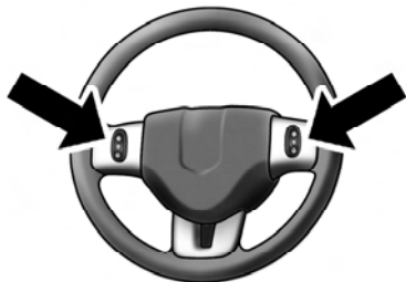
Remote Sound System Controls
