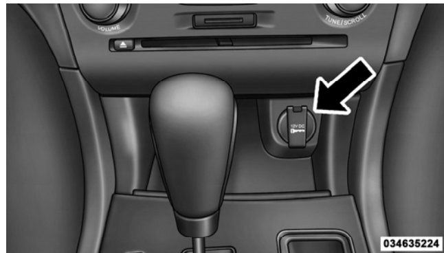
Front Power Outlet
