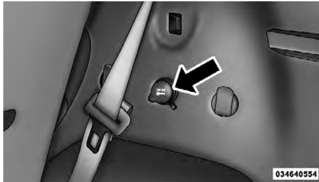
Rear Power Outlet
