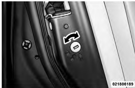
Child-Protection Door Lock Function
