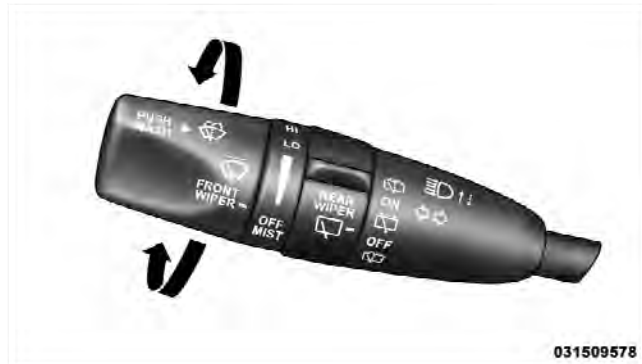
Windshield Wiper Operation
