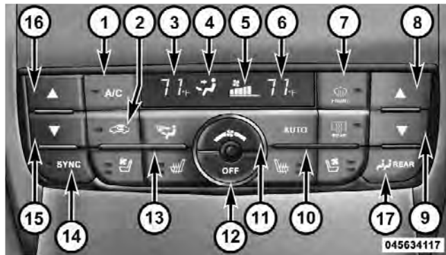
Automatic Temperature Control (ATC) Panel
