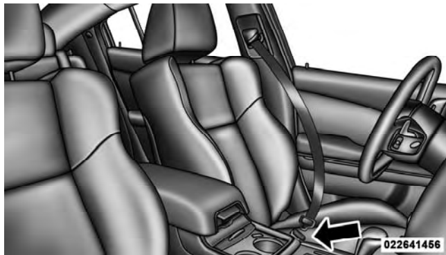
Inserting Latch Plate Into Buckle
