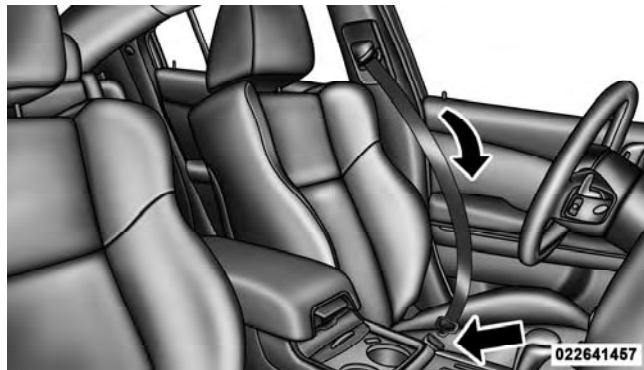
Pulling Out The Lap/Shoulder Belt Latch Plate
