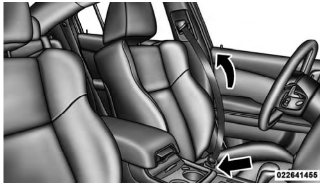
Removing Slack From Belt
