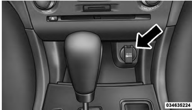
Front Power Outlet
