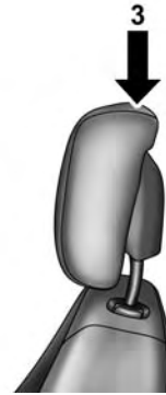
3 — Final Downward Movement To Engage Locking Mechanism
