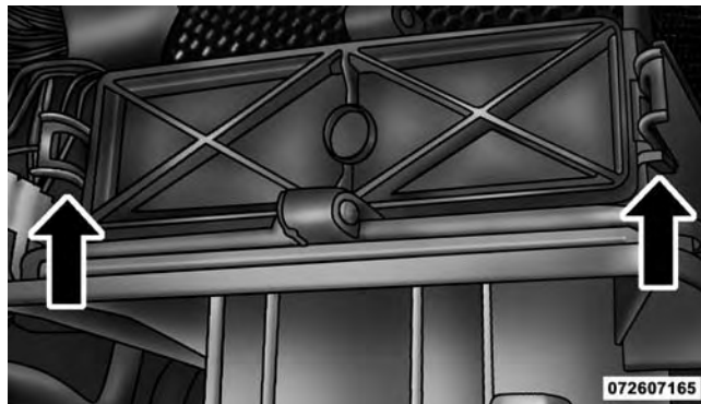
A/C Air Filter Replacement
