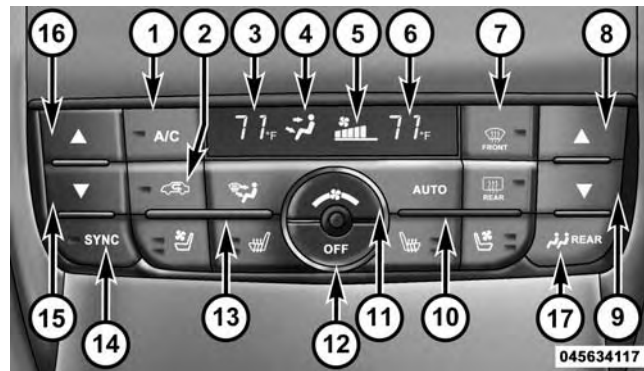
Automatic Temperature Control (ATC) Panel
