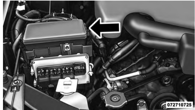
Totally Integrated Power Module
