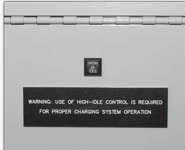
Fast Idle Switch is shown as mounted on Driver's Overhead Control Panel (ref. page 20)
