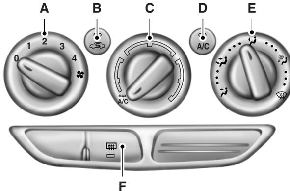
A. **Fan speed control:** Controls the volume of air circulated in your vehicle. Adjust to select the desired fan speed or switch off. If you switch the fan off, the windshield may fog up.
