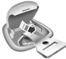
4. Clip the tether strap to the anchor as shown.
