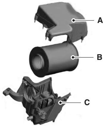
1. Loosen the screws that secure the air filter housing cover (A).
