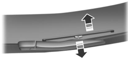
1. Press the wiper blade against the glass with one hand and hold it.
