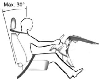
When you use them properly, the seat, head restraint, safety belt and airbags will provide optimum protection in the event of a crash.
