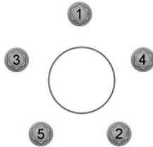
12. Remove the jack and fully tighten the lug nuts in the order shown. See *Wheel Lug Nut Torque Specifications* in this chapter for the proper lug nut torque specification.
