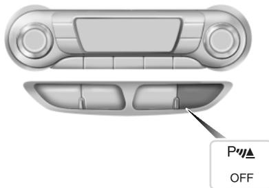
Press the button to switch the system off. It will remain off for the entire ignition cycle.
