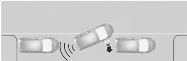
When automatic steering is finished, the touch screen displays a message indicating that the active park assist process is done. The driver is responsible for checking the parking job and making any necessary corrections before putting the transmission in P (Park).
