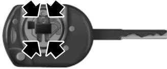
3. Insert the new battery. Refer to the instructions inside the transmitter for the correct orientation of the battery. Press the battery down to make sure it is fully in the housing.
