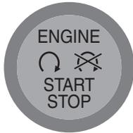
To switch the ignition on, press the start button. All electrical circuits and accessories are operational, and warning lamps and indicators illuminate.
