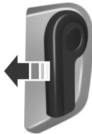
1. Inside the vehicle, pull the hood release handle located under the instrument panel.
