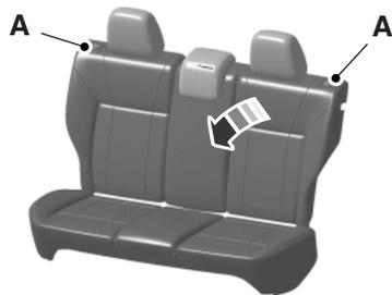
1. Press the unlock buttons (A) down.
