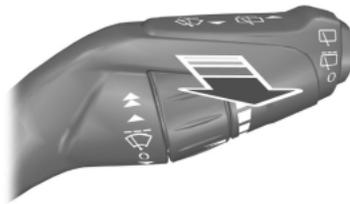
The washer will spray for as long as the lever is pulled toward you. After you release the lever, the wipers will operate for a short time.
