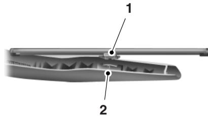
3. To attach the new wiper to the wiper arm, align the slot (1) and cross pin (2) and firmly press the wiper arm into the wiper blade until a click is heard.
