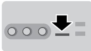
The slot is located either in the center console or behind a small access door in the instrument panel. To access and play music from your cardt, press the lower left corner of the touchscreen, and then select the **SD Card** tab.
