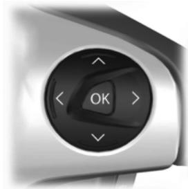
Use the arrows on the right side of steering wheel to navigate through the available menus. Press **OK** to make a selection.
