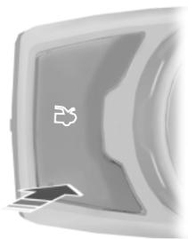
Press the button. It is located on the instrument panel to the left of the steering wheel.
