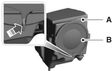
6. Align the tab on the closed end of the air filter element (B) with the slot in the air filter housing.
