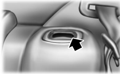
When raising the seat back(s), make sure you hear the seat latch into place and that no red portion is visible on the release button on both sides.
