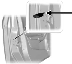
If the central locking function fails to operate, lock the doors individually using the key in the position shown.
