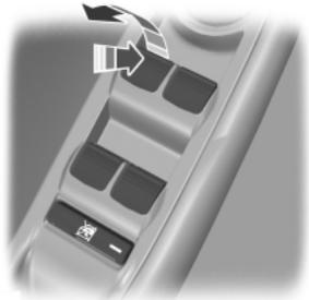
Press the switch to open the window.
