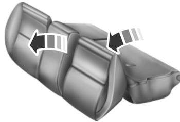
For additional cargo space, flip the seat cushions up before folding the seat back. This feature is only available on vehicles with a split folding seat back.
