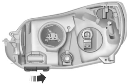
1. Remove the service cap by turning it counterclockwise.
