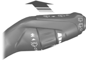
The washer will spray for as long as you push the lever away from you. When you release the lever, the wiper will operate for a short time.
