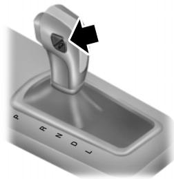
Pressing the transmission control switch on the side of the gearshift lever activates overdrive cancel and grade assist.
