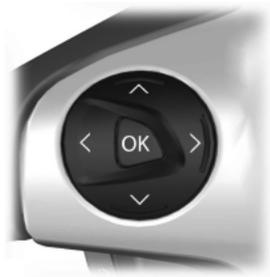
Press the OK button to acknowledge and remove some messages from the information display. Other messages will be removed automatically after a short time. Certain messages need to be confirmed before you can access the menus.
