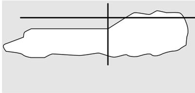
There is a distinct cut-off (change from light to dark) in the left portion of the beam pattern. The top edge of this cut-off should be positioned 2 inches (5 centimeters) below the horizontal reference line.
