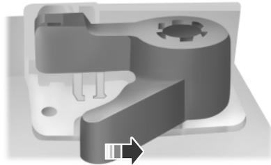
2. Go to the front of the vehicle and locate the auxiliary latch located under the front of the hood (left of center) and then release it by pushing the auxiliary latch to the right.
