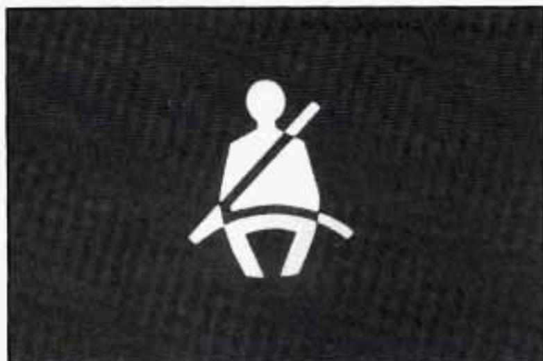
When the key is turned to RUN or START, a tone will come on for about eight seconds to remind people to fasten their safety belts, unless the driver's safety belt is already buckled. The safety belt light will also come on and stay on for about 20 seconds, then it will flash for about 55 seconds. If the driver's belt is already buckled, neither the tone nor the light will come on.
