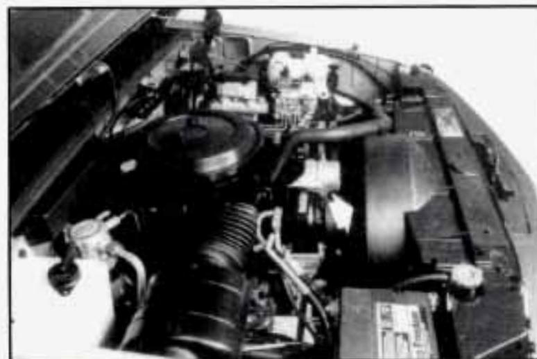
Your vehicle, if it has air conditioning, may have a auxiliary engine fan in addition to the belt driven fan.
