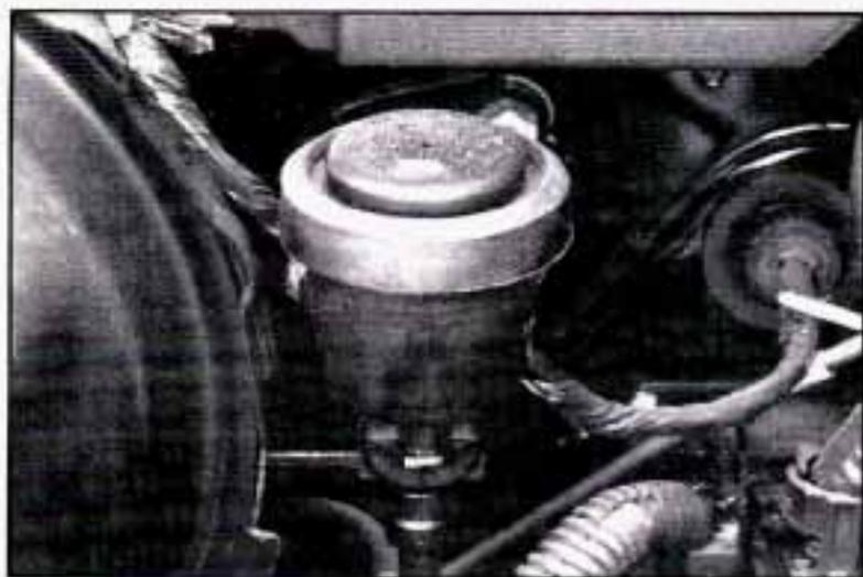
Refer to the Maintenance Schedule to determine how often you should check the fluid level in your clutch master cylinder reservoir and for the proper fluid.
