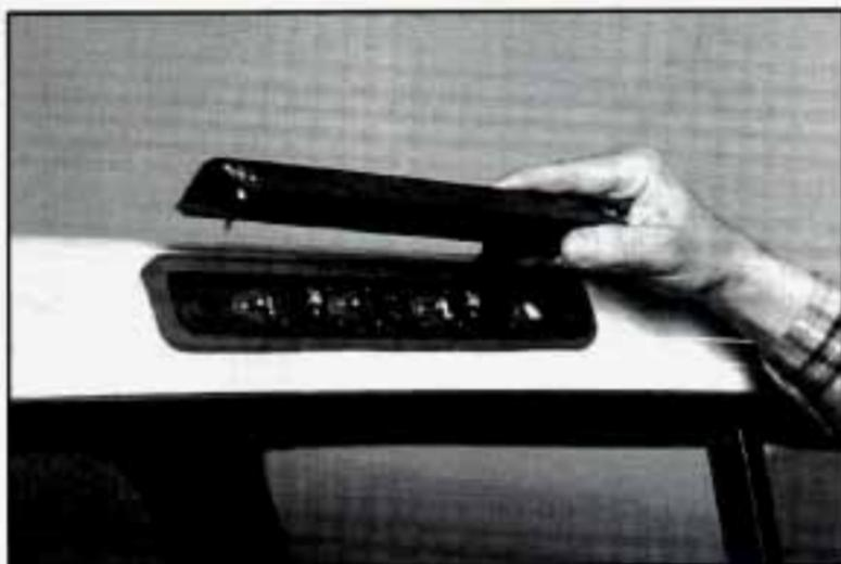
1. Remove the screws and lift off the lens.
