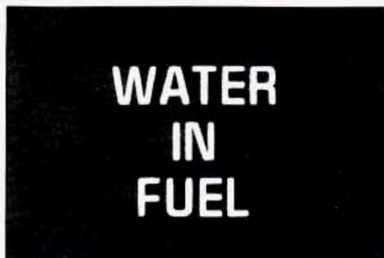
This red light will come on to warn you if there is water in the diesel fuel system. For more information on how this light works, see "Diesel Fuel Requirements and Fuel System" in the Index.
