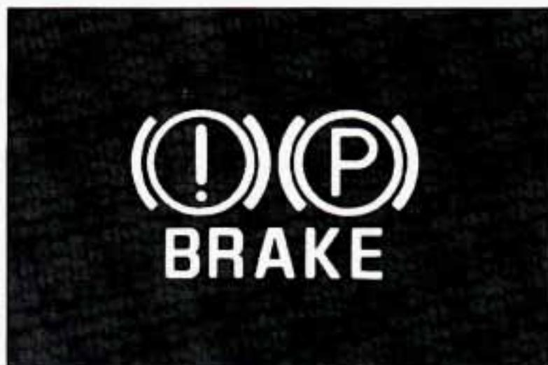
Your vehicle's hydraulic brake system is divided into two parts. If one part isn't working, the other part can still work and stop you. For good braking, though, you need both parts working well.
