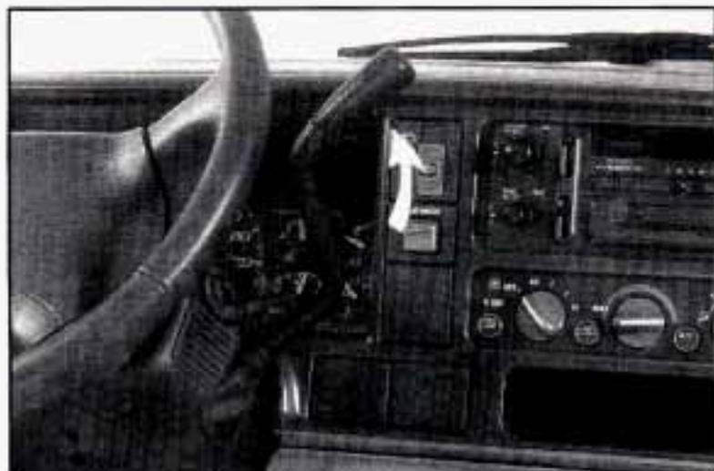
1. Hold the brake pedal down with your right foot and set the parking brake.
