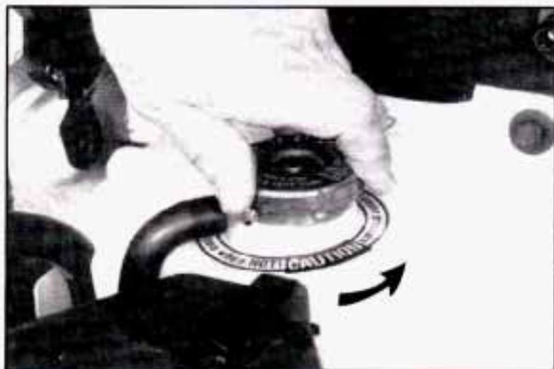
1. You can remove the coolant surge tank pressure cap when the cooling system, including the coolant surge tank pressure cap and upper radiator hose, is no longer hot. Turn the pressure cap slowly to the left until it first stops. (Don't press down while turning the pressure cap.)
