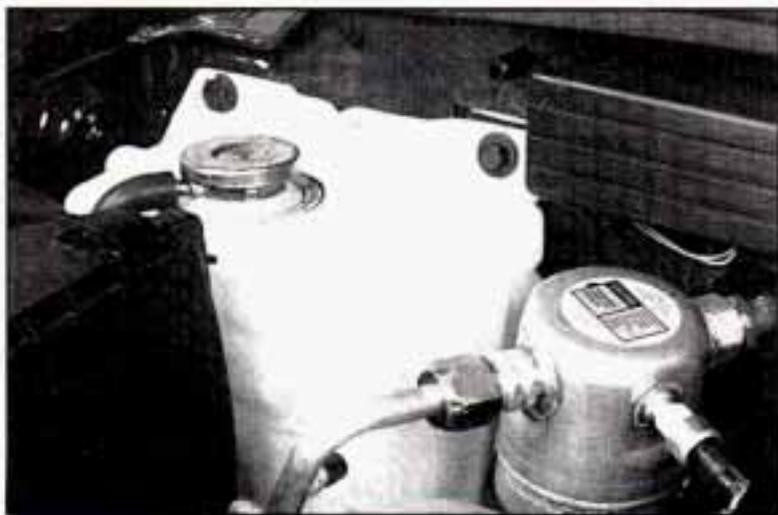
The coolant surge tank is located on the passenger side at the rear corner of the engine compartment.
