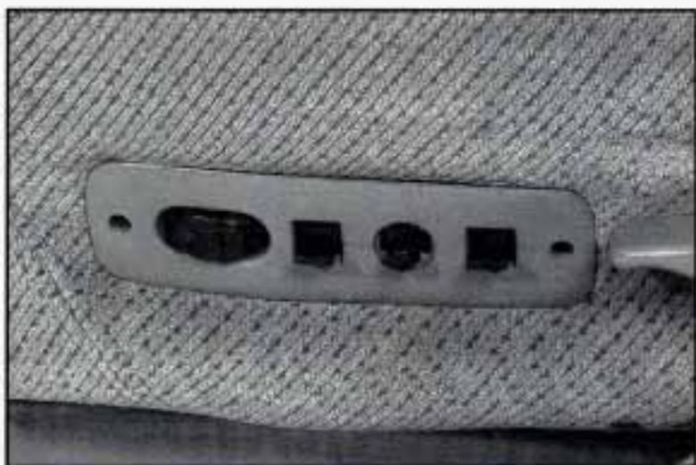
If your vehicle has a power seat on the driver's side, you can adjust it with this switch at the outside edge of the seat.
