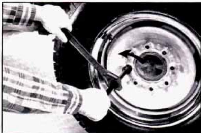
Now, use the ratchet and wheel wrench to loosen all the wheel nuts. Turn the wheel wrench counterclockwise, with DOWN facing you, to loosen the wheel nuts.
