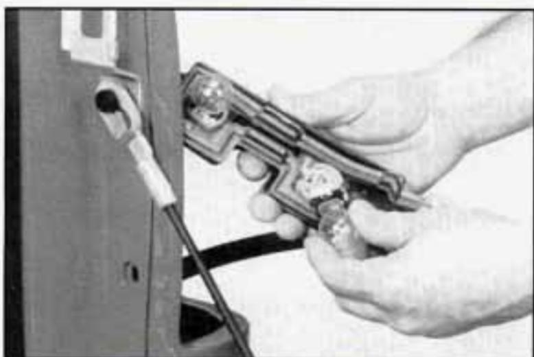
4. Pull the old bulb straight out of the socket.
