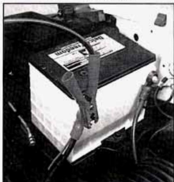
7. Don't let the other end touch metal. Connect it to the positive (+) terminal of the good battery. Use a remote positive (+) terminal if the vehicle has one.
