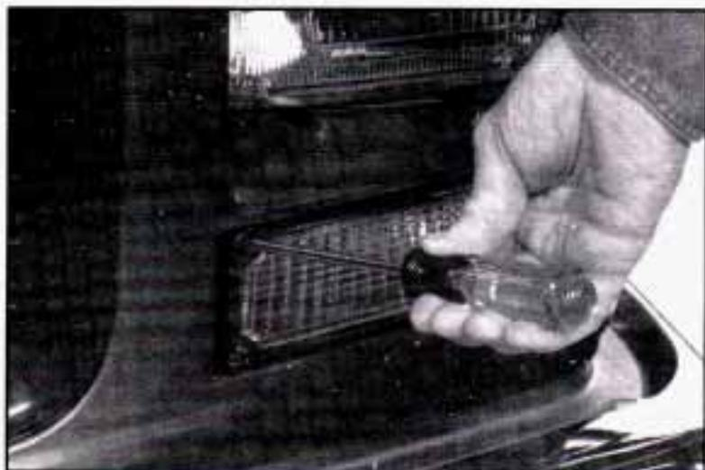
1. Remove the two screws at the inside edge of the parking/turn signal lamp assembly.
