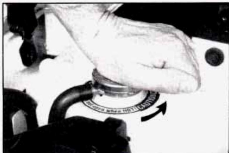
2. Then keep turning the cap, but now push down as you turn it. Remove the pressure cap.
