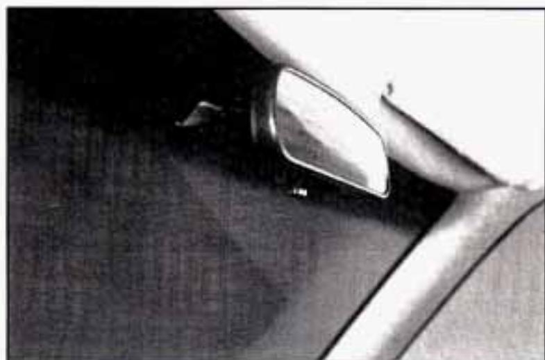
Push or pull the tab under the mirror to reduce glare from headlamps behind you after dark.
