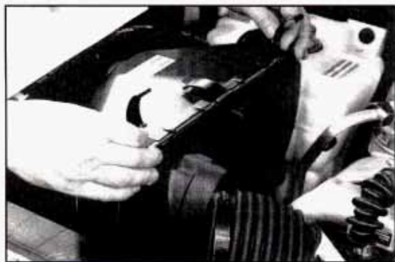
Then, unhook the cover retaining clips and push the rear of the cover toward the engine.
