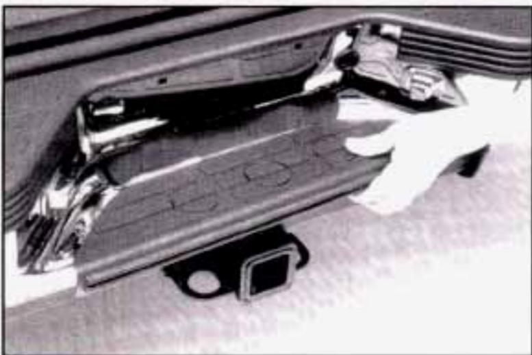
To remove the pad, lift the edge of the pad from the rear of the bumper and swing it forward. When the pad releases from the bumper holes, lift the pad off.
