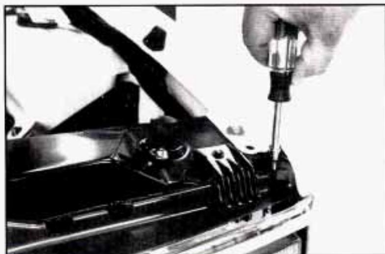
1. Remove the two screws at the top of the radiator support.
