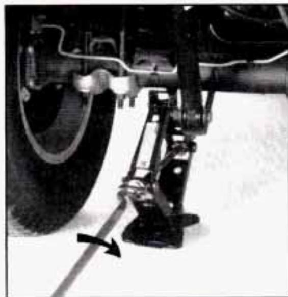
With UP on the ratchet facing you, raise the vehicle by rotating the ratchet and wheel wrench clockwise. Raise the vehicle far enough off the ground so there is enough room for the spare tire to fit.
