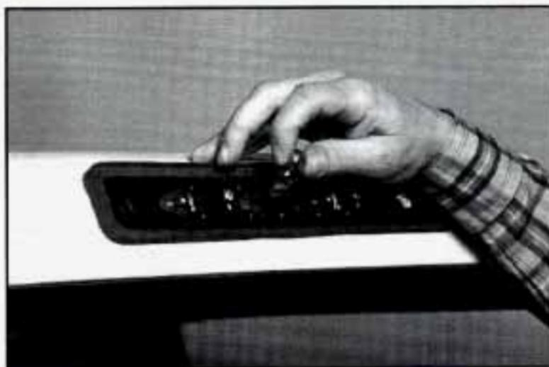
3. Put a new bulb into the socket and push it in until it is tight.
