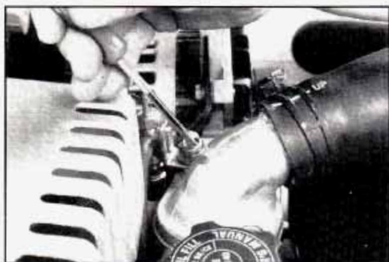
3. After the engine cools, open the air bleed valve on the thermostat housing.
