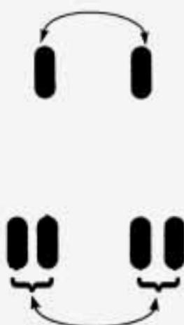
If your vehicle has dual rear wheels and the load range or tread design for your front tires is different from your rear tires, always use the correct rotation pattern shown here when rotating your tires. The dual tires are rotated as a pair, and the inside rear tires become the outside rear tires.
