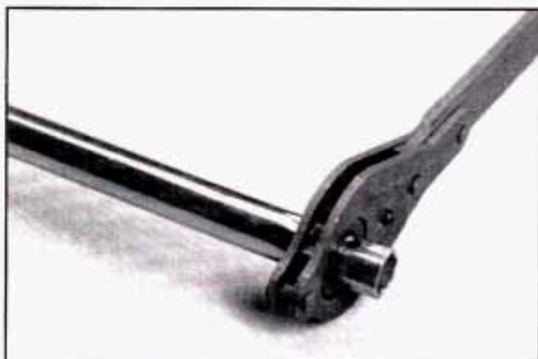
Attach the ratchet to the wheel wrench with the DOWN marking facing you.
