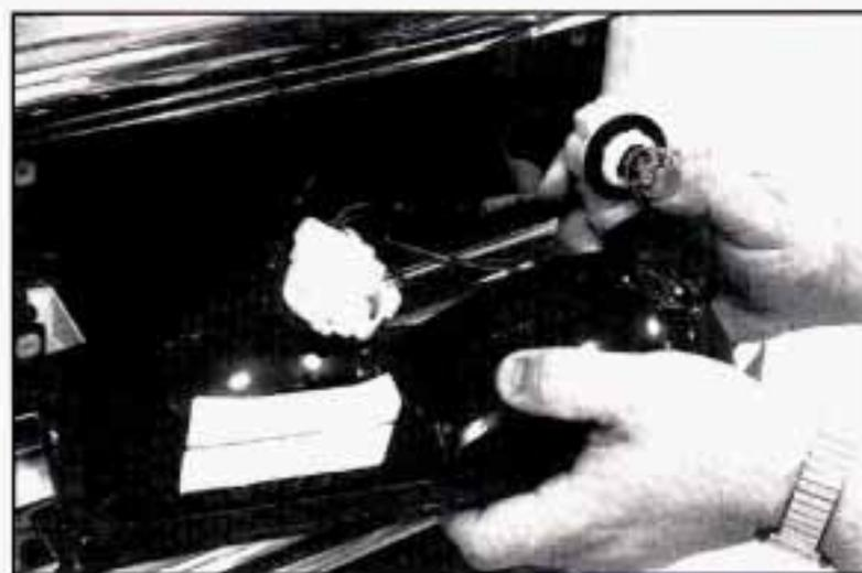
3. Pull the socket out of the lamp assembly.
