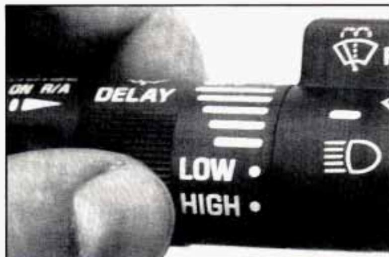
You control the windshield wipers by turning the band with the wiper symbol on it.
