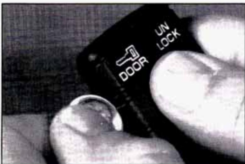
1. Insert a dime in the side seam of the transmitter housing, near the key ring hole.
