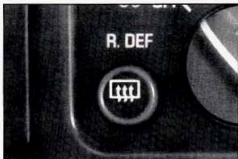
To turn on the rear window defogger, press the rear defog button next to the fan control knob.
