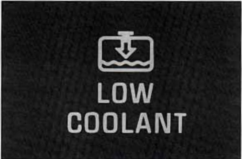
A black rectangular box containing a white icon of a coolant reservoir with a downward arrow and wavy lines below it, and the text "LOW COOLANT" in white, bold, sans-serif capital letters below the icon.
