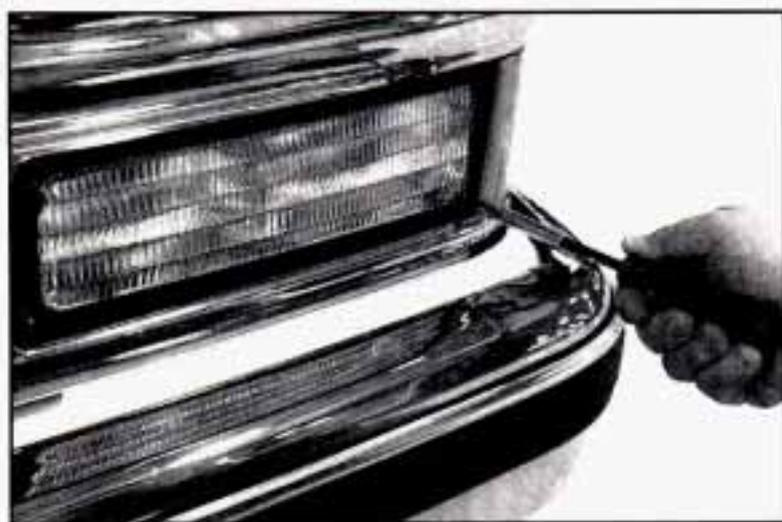
1. Remove the screws and take out the parking/turn signal lamp assembly.
