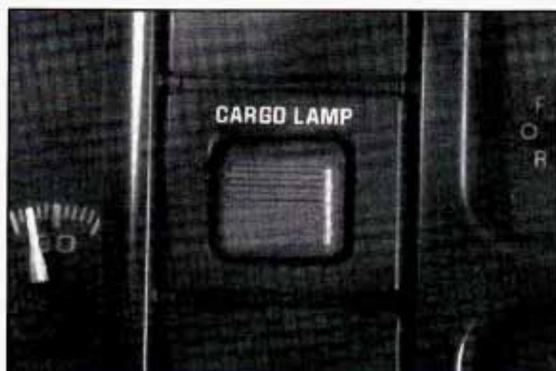
Press the top, ribbed part of the switch to turn the cargo lamp on, and press the bottom of the switch to turn it off.
