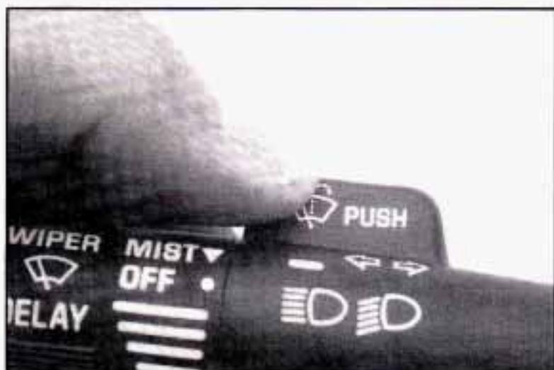
At the top of the lever there's a paddle with the word **PUSH** on it. To spray washer fluid on the windshield, push the paddle.
