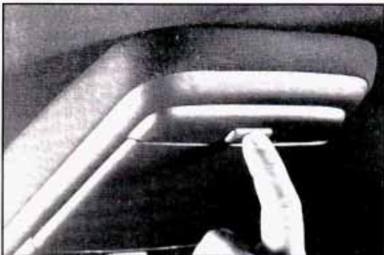
To open the rear compartment, press the release button located at the rear of the compartment door.
