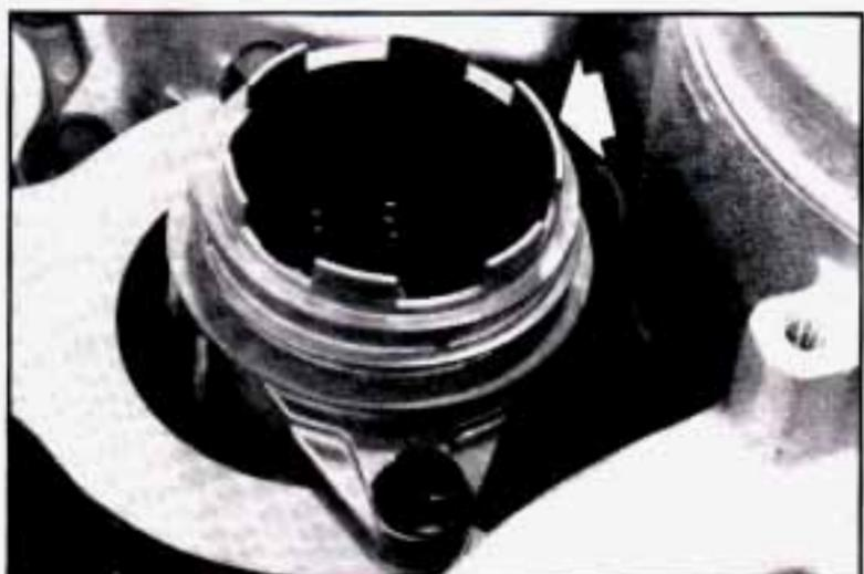
6. Line up the widest slot in the top of the new element with the widest key on the top of the filter head. Push the element in until the mating surfaces touch.
