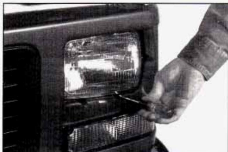
1. Remove the four screws from the headlamp retainer.
