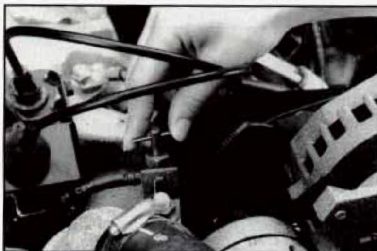
4. With the engine off, open the water drain valve 2 to 3 turns. When standing in front of the vehicle, the valve is located on the right side of the thermostat housing.
