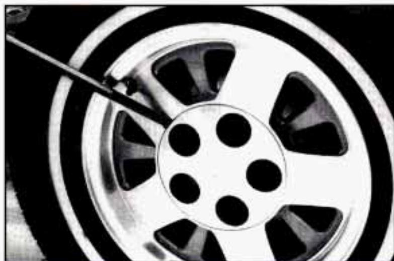
If the wheel has a smooth center piece or a center piece with recessed nuts, place the wheel wrench in the slot on the wheel and gently pry out.
