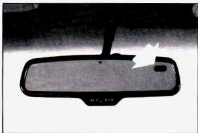
Your vehicle may have an optional electrochromic inside rearview mirror. An electrochromic inside rearview mirror, when on, automatically dims to the proper level to minimize glare from lights behind you after dark.
