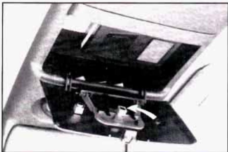
Add one peg at a time until the PUSH button on the compartment door operates the garage door opener, with the compartment door closed, when you push the button marked PUSH.
