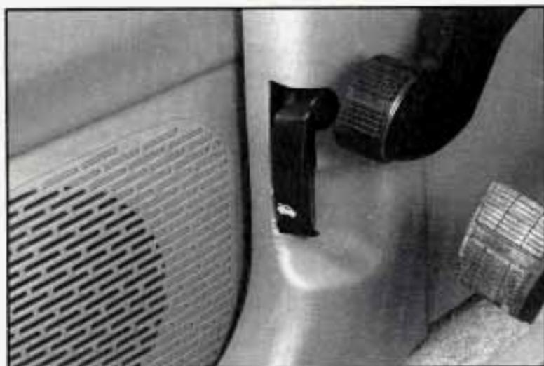
To open the hood, first pull the handle inside the vehicle.
