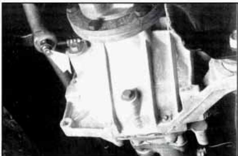
If the level is below the bottom of the filler plug hole, you'll need to add some lubricant.
