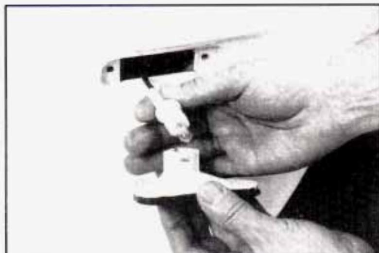
2. Turn the bulb socket to the left and remove it from the lens assembly.
