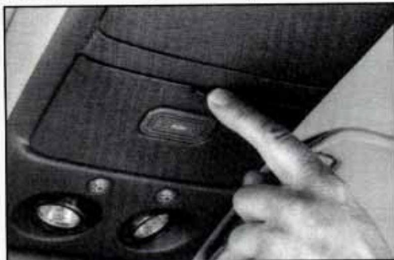
To install the garage door opener, first open the compartment door by pressing the release button forward.
