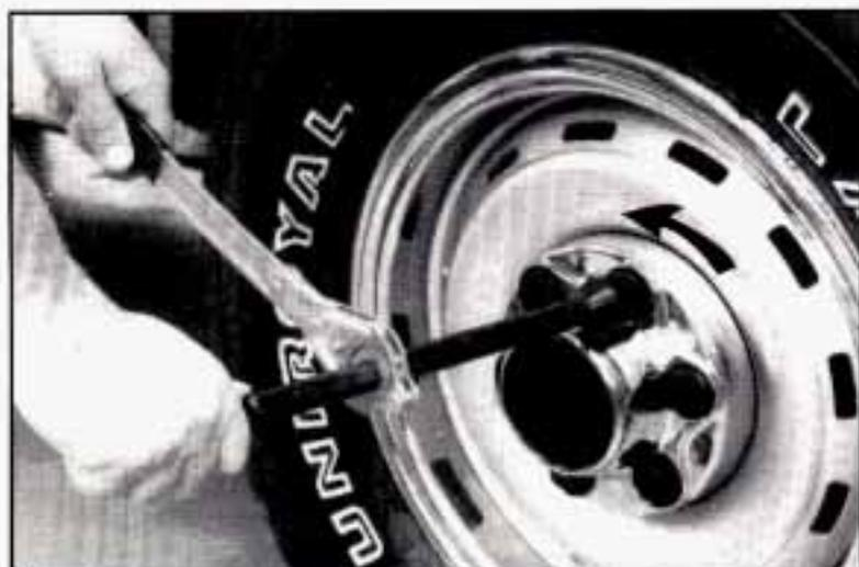
If your vehicle has wheel nut caps, use the wheel wrench and ratchet to remove them. Turn the wheel wrench counterclockwise, with DOWN facing you, to remove the wheel nut caps. Then take off the hub cap.
