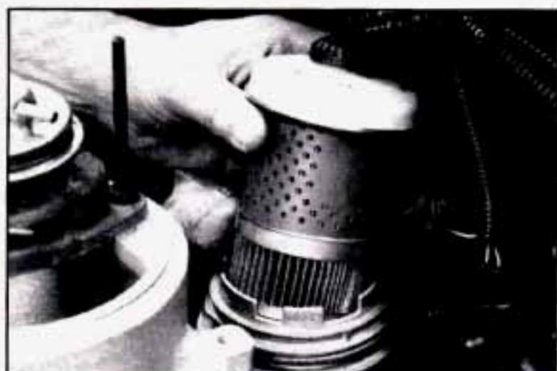
4. Lift the element out of the filter head.
