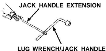
8. Remove the lug nuts, wheel cover and wheel.
