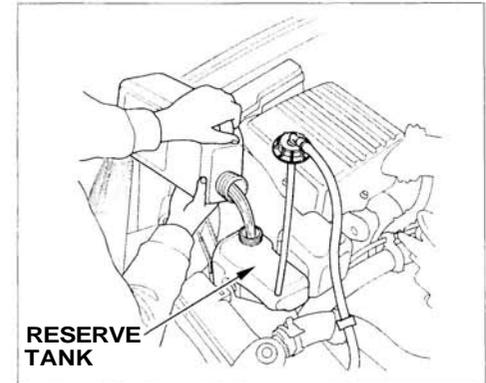
12. Fill the reserve tank to the MAX mark. Install the reserve tank cap.
