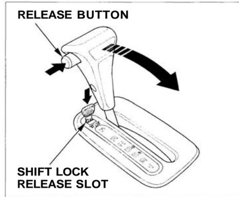
3. Insert the key in the Shift Lock Release slot next to the shift lever.
