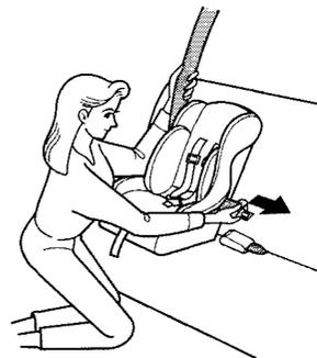
1. With the child seat in the desired seating position, route the belt through the child seat according to the seat maker's instructions, then insert the latch plate into the buckle.
