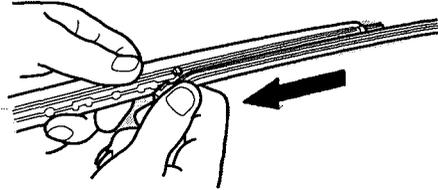
5. Slide the new blade into the holder. Make sure it is engaged in the slot along its full length.
