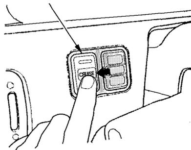
1. Push in the Cruise Control Master Switch to the left of the steering column. The indicator in the switch will light.
