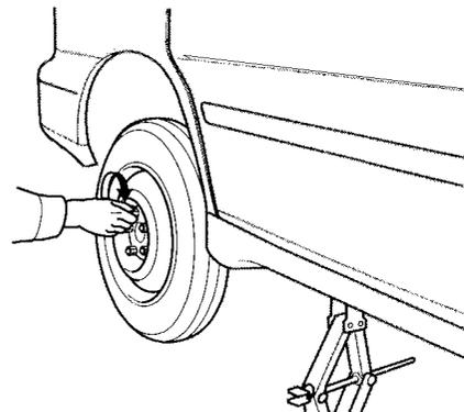
14. Put on the spare tire. Put the wheel nuts back on finger-tight, then tighten them in a crisscross pattern with the wheel wrench until the wheel is firmly against the hub. Do not try to tighten them fully.
