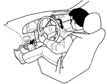
**Reverse (R)** — To shift to Reverse from Park, see the explanation under Park. To shift to Reverse from Neutral, come to a complete stop and then shift. Pull the shift lever towards you before shifting into Reverse from Neutral.
