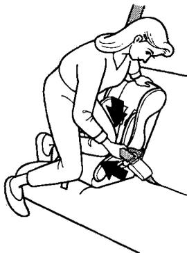
4. After confirming that the belt is locked, grab the shoulder part of the belt near the buckle and pull up to remove any slack from the lap part of the belt. Remember, if the lap part of the belt is not tight, the child seat will not be secure. It may help to put weight on the child seat, or push on the back of the seat while pulling up on the belt.
