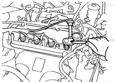
5. Torque the spark plug. (If you do not have a torque wrench, tighten the spark plug two-thirds of a turn after it contacts the cylinder head.)
