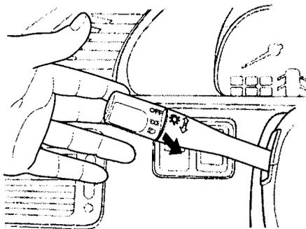
To change between low beams and high beams, pull the turn signal lever until you hear a click, then let go. The blue high beam indicator will light (see page 54).
