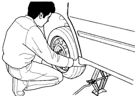
12. Remove the wheel nuts and flat tire. Temporarily place the flat tire on the ground with the outside surface of the wheel facing up. You could scratch the wheel if you put it face down.
