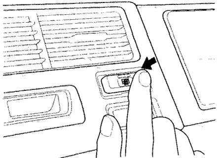
The rear window defogger will clear fog, frost, and thin ice from the window. Push the defogger button to turn it on and off. The light in the button lights to show the defogger is on. If you do not turn it off, the defogger will shut itself off after about 25 minutes. It also shuts off when you turn off the ignition. You have to turn it on again when you restart the vehicle.
