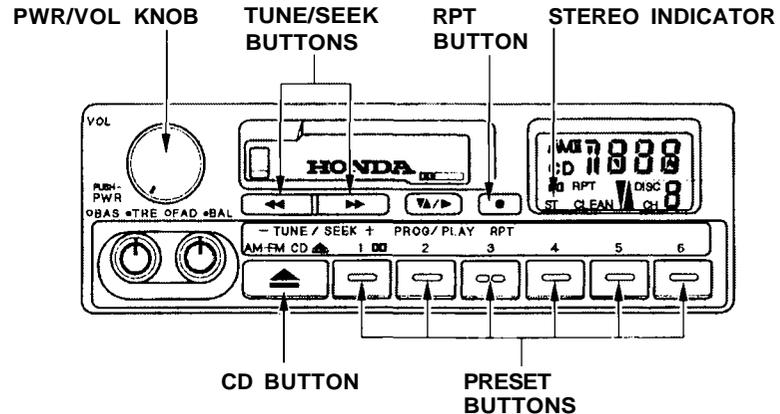
To select a different disc, press the appropriate preset button (1 — 6). If you select an empty slot in the magazine, the changer will, after finding that slot empty, try to load the CD in the next slot. This continues until it finds a CD to load and play.
