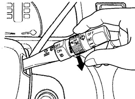
To operate the wipers in mist mode, push the control lever down. The wipers run at high speed until you release the lever. This gives you a quick way to clear the windshield.
