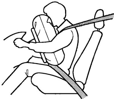
If you ever have a severe frontal collision, the sensors will detect rapid deceleration and signal the control unit to instantly inflate the airbags.
