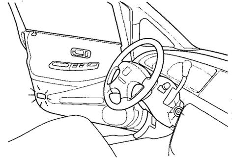
Each door has a courtesy light. This light comes on when you open the door. Your vehicle also has a courtesy light in the ignition switch. This light comes on when you open the driver's door. It remains on for several seconds after the door is closed.
