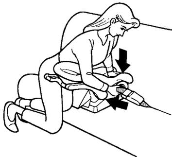
To install a rear-facing child seat with the lap belt, follow instruction number 1 on page 28 for routing and latching the seat belt. Then pull hard on the loose end of the belt to remove any slack (it may help to put weight on the child seat while pulling on the belt). Finally, follow instruction number 5 of page 29 to verify that the child seat is secure.
