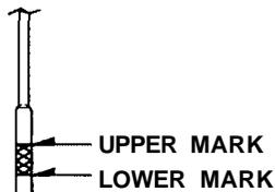
3. Insert the dipstick all the way into the transmission.
