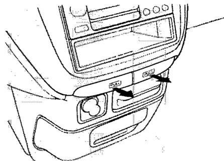
To use the front beverage holder, pull on the front. Push the holder all the way in to close it.
