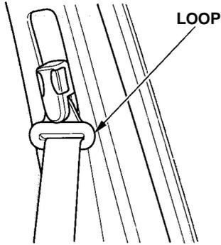
If your seat belts get dirty, you can use a soft brush with a mixture of mild soap and warm water to clean them. Do not use bleach, dye, or cleaning solvents. They can weaken the belt material. Let the belts air-dry before you use the vehicle.
