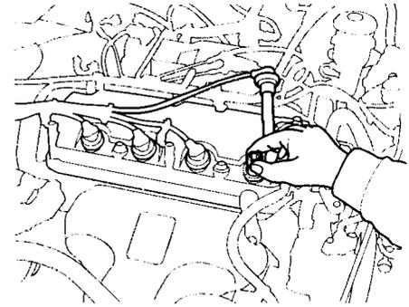
4. Put the new spark plug into the socket; then screw it into the hole. Screw it in by hand so you do not crossthead it.
