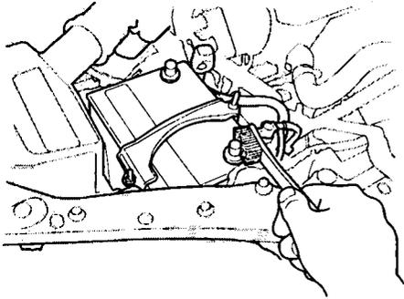
If the terminals are severely corroded, clean them with baking soda and water. Then use a wrench to loosen and remove the cables from the terminals. Always disconnect the negative (—) cable first and reconnect it last. Clean the battery terminals with a terminal cleaning tool or wire brush. Reconnect and tighten the cables, then coat the terminals with grease.
