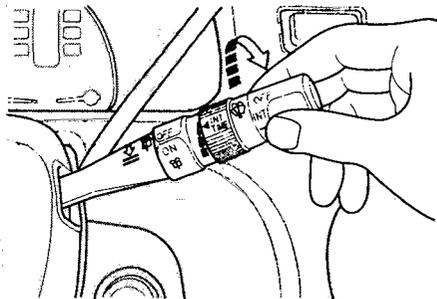
The right lever controls the windshield wipers and washers. The rotary switch at the end of the lever has three positions:
