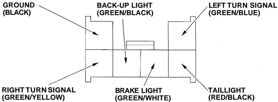
Your vehicle has a trailer lighting connector. To use the connector, remove the left rear light cover. Refer to the drawing above for the wiring color code and purpose of each connector pin.
