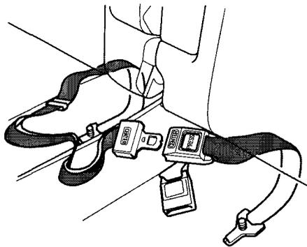
To fasten the belt, insert the latch plate into the buckle marked **CENTER**, then tug on the belt to make sure the buckle is latched.
