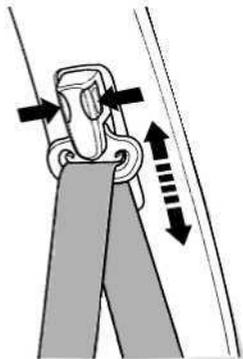
If the seat belt touches or crosses your neck, or if it crosses your arm instead of your shoulder, you need to adjust the seat belt anchor height. An improperly positioned seat belt can cause severe neck injuries if the belt is positioned too high, or serious chest or internal injuries if the belt is positioned too low.
