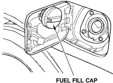
3. Remove the fuel fill cap slowly. You may hear a hissing sound as pressure inside the tank escapes. Place the cap in the holder on the fuel fill door.
