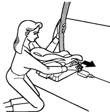
1. With the child seat in the desired back seating position, route the belt through the child seat according to the seat maker's instructions, then insert the latch plate into the buckle.
