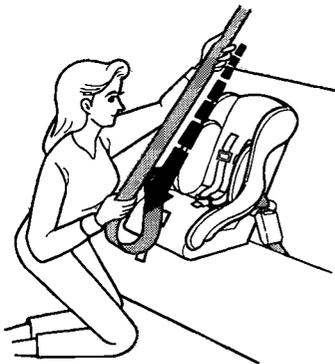
2. To activate the lockable retractor, slowly pull the shoulder part of the belt all the way out until it stops, then let the belt feed back into the retractor (you might hear a clicking noise as the belt retracts).
