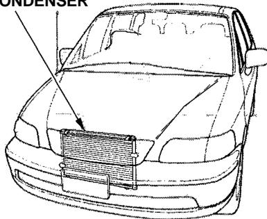
Run the air conditioning at least once a week during the cold weather months. Run it for at least ten minutes while you are driving at a steady speed with the engine at normal operating temperature. This circulates the lubricating oil contained in the refrigerant.
