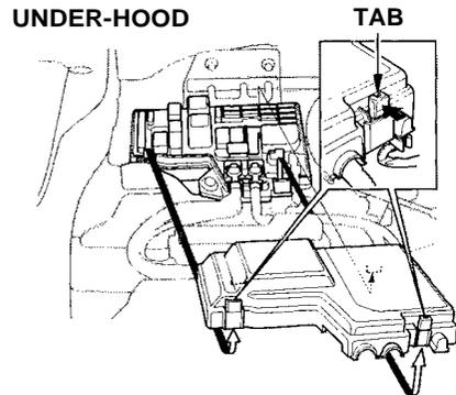
The under-hood fuse box is located in the engine compartment on the passenger's side. To open, push the tab as shown.
