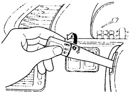
The rotating switch on the left lever controls the lights. Turning this switch to the “OFF” position turns on the parking lights, taillights, instrument panel lights, side-marker lights, and rear license plate lights. Turning the switch to the “D” position turns on the headlights.
