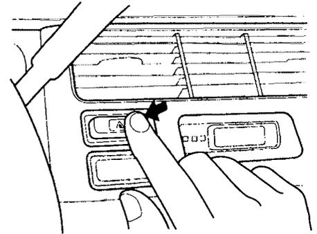
Push the red button to the left of the clock to turn on the *hazard* warning lights (four-way flashers). This causes all four outside turn signals and both indicators in the instrument panel to flash. Use the *hazard* warning lights if you need to park in a dangerous area near heavy traffic, or if your vehicle is disabled.
