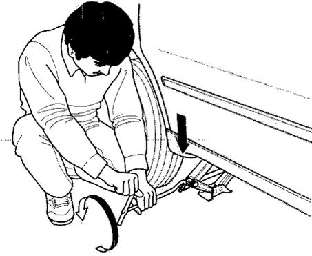
15. Lower the vehicle to the ground and remove the jack.
