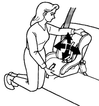
5. Push and pull the child seat forward and from side to side to verify that it is secure enough to stay upright during normal driving maneuvers. If the child seat is not secure, unlatch the belt, allow it to retract fully, then repeat these steps.
