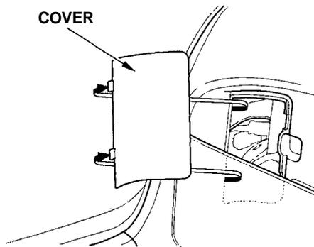
1. Open the tailgate. Swing the taillight cover open and remove it. To replace a bulb on the right side, remove the spare tire (see page [224](#)).
