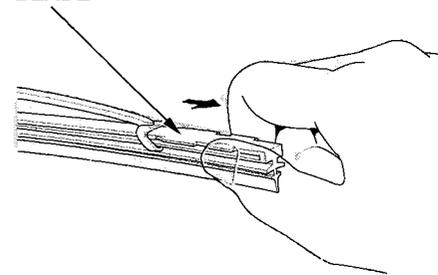
3. Remove the blade from its holder by grasping the tabbed end of the blade. Pull firmly until the tabs come out of the holder.
