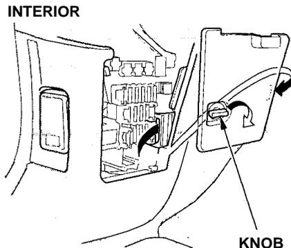
The interior fuse box is underneath the dashboard on the driver's side. To open it, turn the knob as shown.
