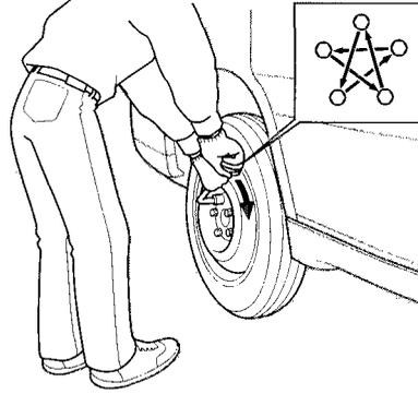
16. Tighten the wheel nuts securely in the same crisscross pattern. Have the wheel nut torque checked at the nearest automotive service facility.
