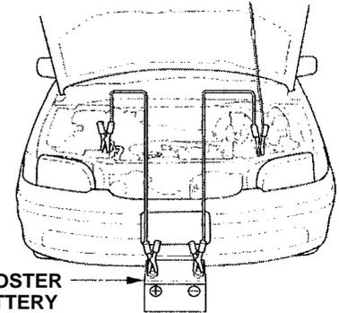
6. Start your vehicle. If the starter motor still operates slowly, check the jumper cable connections to make sure they have good metal-to-metal contact.
