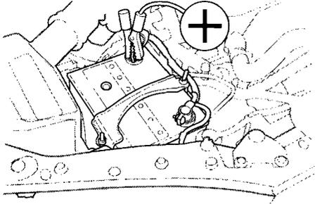
3. Connect one jumper cable to the positive (+) terminal on the booster battery. Connect the other end to the positive (+) terminal on your Honda's battery.
