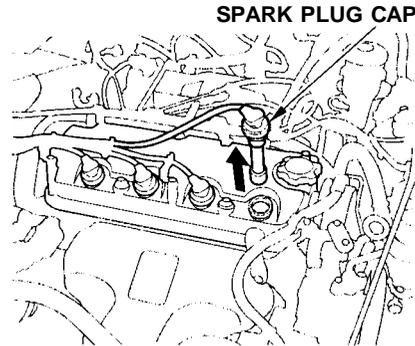
1. Clean up any dirt and oil around the spark plug caps.
