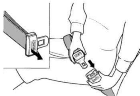
Insert the latch plate into the buckle marked CENTER.
