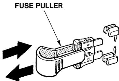
4. Check the smaller fuses in the under-hood fuse box and all the fuses in the interior fuse box by pulling out each fuse with the fuse puller provided in the interior fuse box.
