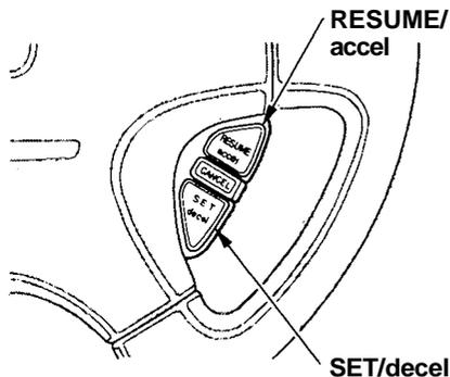
3. Press and hold the SET/decel button on the steering wheel until the CRUISE CONTROL light on the instrument panel comes on. This shows the system is now activated.
