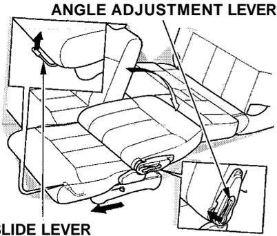
2. Lift the lever and slide the seat forward as far as it will go. Pull the seat-back angle adjustment lever and pivot the seat-back backward. Release the lever when the seat-back is even with the cushion on the third seat.
