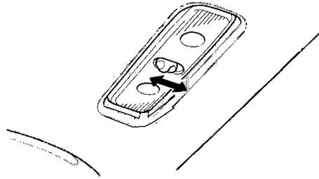
The tailgate light has a two position switch. In the OFF (down) position, the light does not come on. In the ON (up) position, the light comes on when you open the tailgate.
