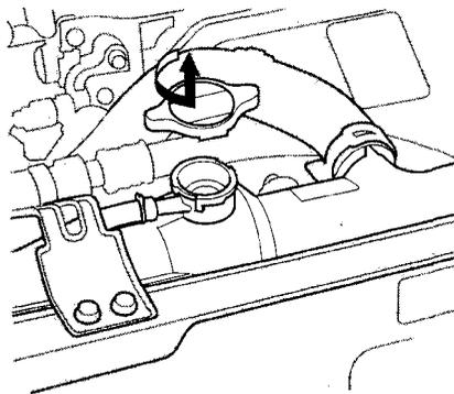
1. Slide the heater temperature control lever to maximum heat. Open the hood. Make sure the engine and radiator are cool to the touch.
