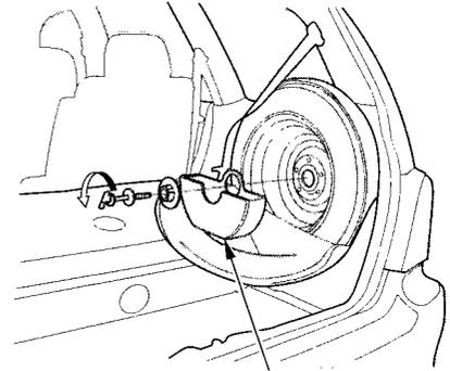
8. Unscrew the wing bolt. Remove the storage bin and spare tire.
