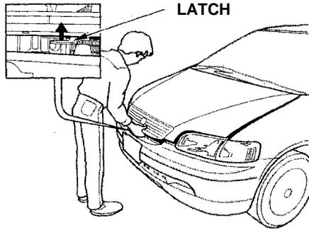
2. Standing in front of the vehicle, put your fingers under the front edge of the hood to the right of center. Slide your hand to the left until you feel the hood latch handle. Push this handle up until it releases the hood. Lift the hood.
