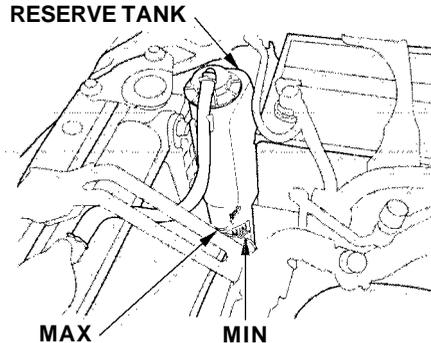
Look at the coolant level in the radiator reserve tank. Make sure it is between the MAX and MIN lines. If it is below the MIN line, see **Adding Engine Coolant** on page [177](#) for information on adding the proper coolant.
