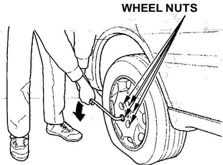
9. Loosen the five wheel nuts 1/2 turn with the wheel wrench.
