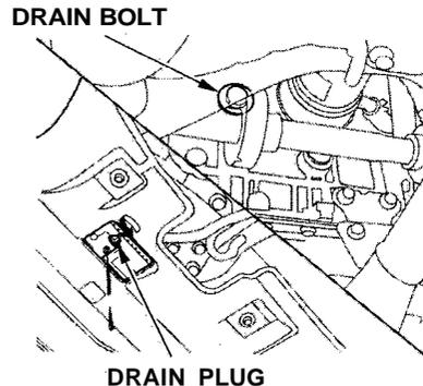
3. Loosen the drain plug on the bottom of the radiator. The coolant will drain through the splash guard. Remove the drain bolt and washer from the engine block.
