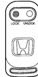
You can lock and unlock your vehicle with the remote transmitter. When you push the LOCK button, all doors and the tailgate lock.
