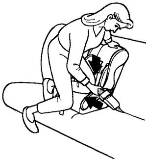
To install a forward-facing child seat with the lap belt, follow instruction number 1 on page 32 for routing and latching the seat belt. Then pull hard on the loose end of the belt to remove any slack (it may help to put weight on the child seat while pulling on the belt). Finally, follow instruction number 5 on page 33 to verify that the child seat is secure.
