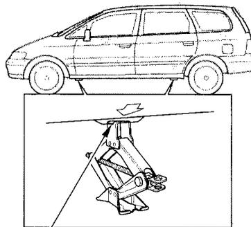
10. Find the jacking point nearest the wheel you are removing. Place the jack under the jacking point. Turn the end bracket clockwise until the top of the jack contacts the jacking point. Make sure the jacking point tab is resting in the jack notch.
