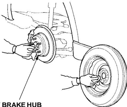
13. Before mounting the spare tire, wipe any dirt off the mounting surface of the wheel and hub with a clean cloth. Wipe the hub carefully, it may be hot from driving.
