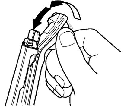
6. Insert both ends of the blade into the holder slots. Make sure they are secure.
