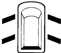
Your vehicle has a door and tailgate monitor light on the instrument panel to indicate when a specific door or the tailgate is not tightly closed.
