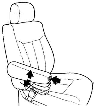
To adjust the front seat armrests, push the button on the front.
