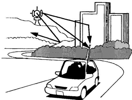
Radio signals, especially on the FM band, are deflected by large objects such as buildings and hills. Your radio then receives both the direct signal from the station's transmitter, and the deflected signal. This causes the sound to distort or flutter. This is a main cause of poor radio reception in city driving.
