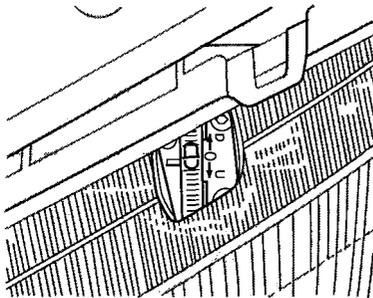
5. Check the vertical angle gauge. The bubble should be centered underneath the longest scribe mark on the gauge.
