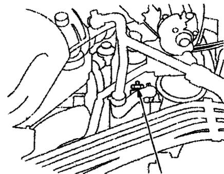
8. Loosen the bleeder bolt on top of the engine. Tighten it again when coolant comes out in a steady stream with no bubbles.
