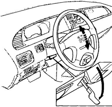
To adjust the steering wheel upward or downward:
