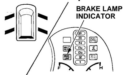
The appropriate light comes on in this display if the tailgate or any door is not closed tightly. If a brake light does not work, the **BRAKE LAMP** indicator comes on when you push the brake pedal with the ignition switch ON (II).
