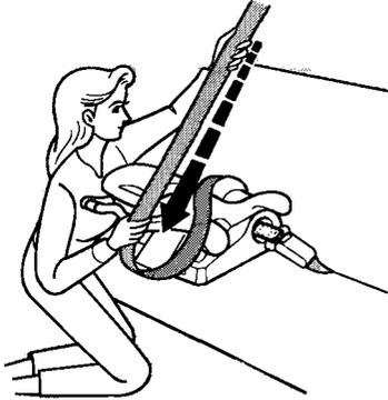
2. To activate the lockable retractor, slowly pull the shoulder part of the belt all the way out until it stops, then let the belt feed back into the retractor (you might hear a clicking noise as the belt retracts).
