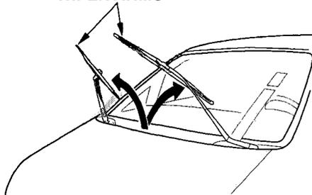
Check the condition of the wiper blades at least every six months. Look for signs of cracking in the rubber, or areas that are getting hard. Replace the blades if you find these signs, or they leave streaks and unwiped areas when used.
