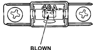
3. Check each of the large fuses in the under-hood fuse box by looking through the top at the wire inside. Removing these fuses requires a Phillips-head screwdriver.
