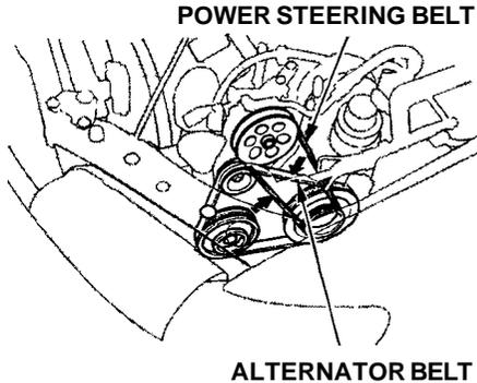
Check the condition of the two drive belts. Examine the edges of each belt for cracks or fraying. Check the tension of each belt by pushing on it with your thumb midway between the pulleys. The belts should have the following "play" or deflection.
