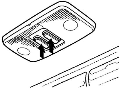
You can turn on the spotlight by pushing the button next to each light when the position lights are turned on. Push the button again to turn it off.
