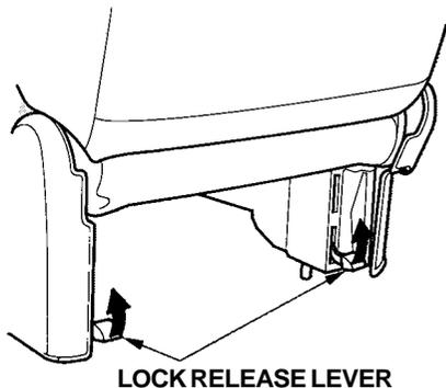
Both seats can be removed to give more cargo capacity.
