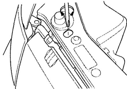
7. If you cannot get an indicator to align, have your Honda dealer inspect the vehicle for body damage or suspension problems.
