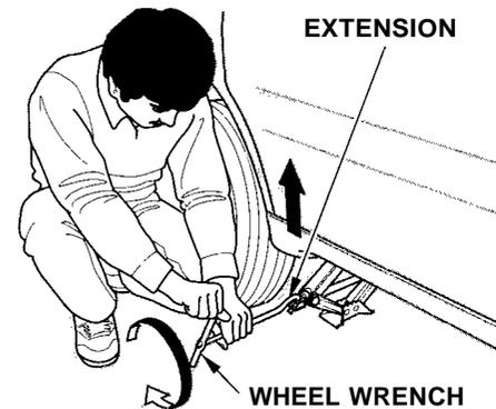
11. Use the extension and wheel wrench as shown to raise the vehicle until the flat tire is off the ground.
