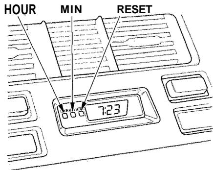
The digital clock displays the time with the ignition switch ON (II). To set the clock:
