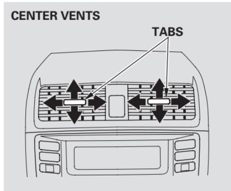
To adjust the air flow from each vent, move the tab in the center of each vent up-and-down and side-to-side.
