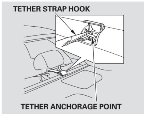
Attach the tether strap hook to the tether anchorage point as shown in the illustration, then tighten the strap according to the child seat maker's instructions. Make sure the strap is not twisted.
