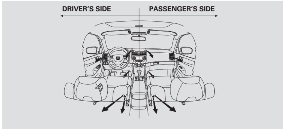
To set the driver's side temperature to a different value than the passenger's, press the DUAL button, then turn the driver's control dial. To set the passenger's side to a different value than the driver's side, turn the passenger's control dial (see page [131](#)). You can adjust the passenger's side without pressing the DUAL button first.
