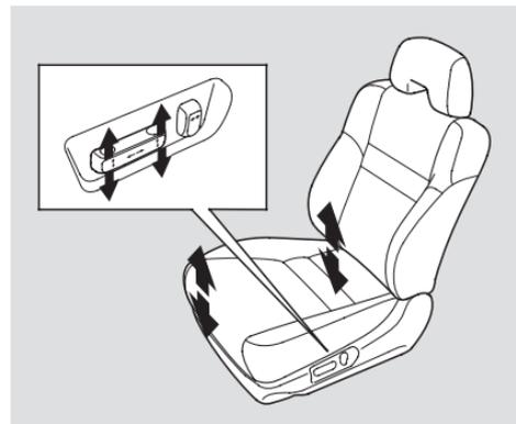
Pull up or push down on the front of the switch to move the seat bottom's front edge up or down. Pull up or push down on the rear of the switch to move the rear of the seat bottom up or down.
