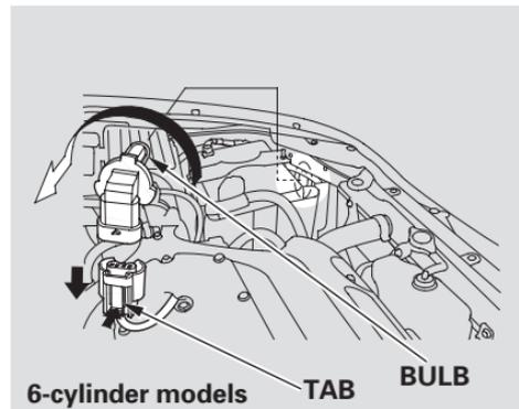
5. Push the electrical connector back onto the bulb. Make sure it is on all the way.
