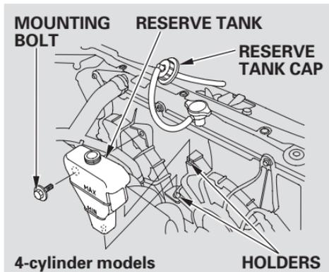
5. Remove the reserve tank mounting bolt with a wrench.
