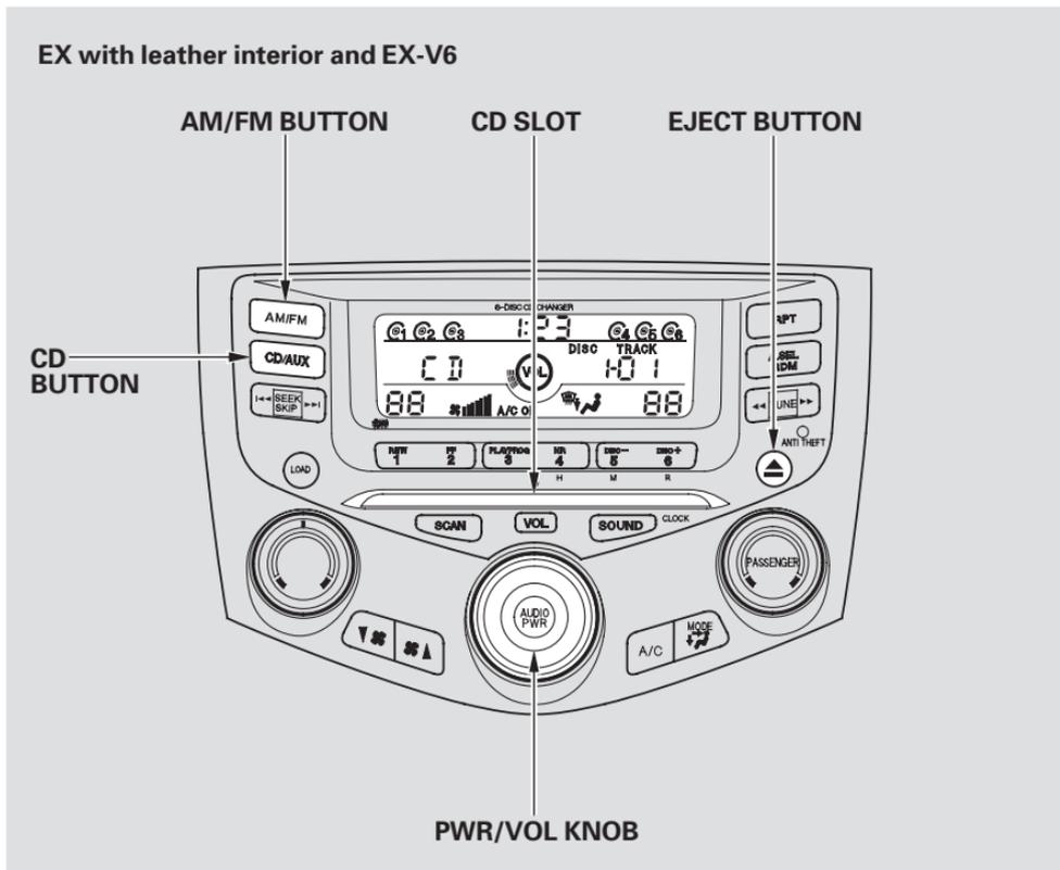
If you press the eject button while listening to the radio, or with the audio system turned off, the disc that was last selected is ejected. After that disc is ejected, pressing the eject button again will eject the next disc in numerical order. By doing this six times, you can remove all the CDs from the changer.
