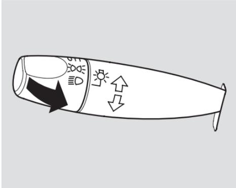
To flash the high beams, pull the turn signal lever back lightly, then release it. The high beams will come on and go off.
