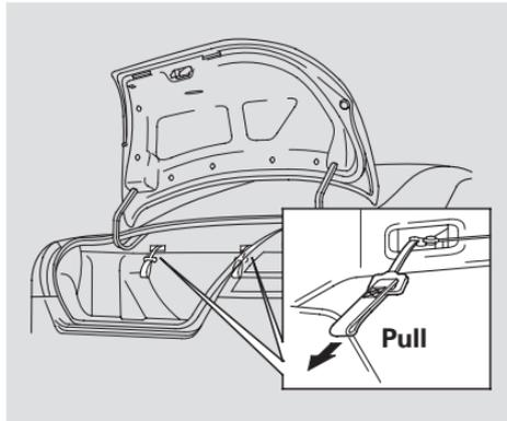
To release the seat-back from inside the trunk, pull the release under the trunk panel. Push the seat-back down, then let go of the release.
