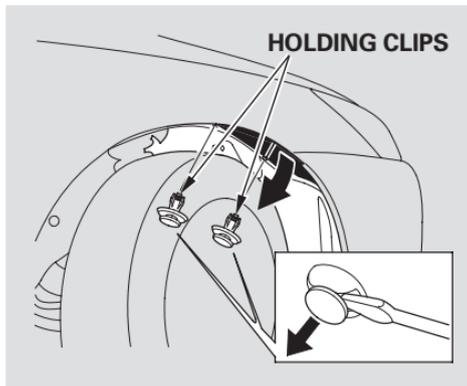
2. Use a flat-tipped screwdriver to remove the two holding clips from the inner fender.
