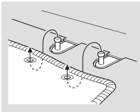
The Honda driver's floor mat that came with your car was designed to be hooked over the floor mat anchors. This keeps the floor mat from sliding forward and possibly interfering with the pedals.
