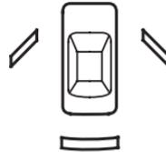
The appropriate light comes on in this display if the trunk or either door is not closed tightly.
