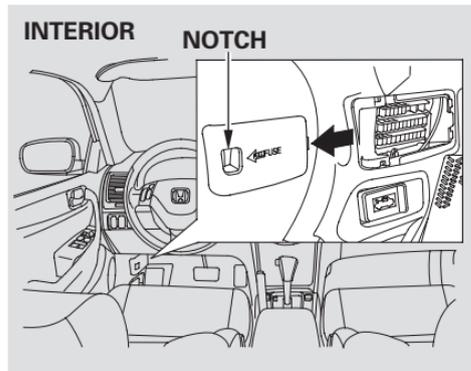
The interior fuse box is on the driver's lower left side. To remove the fuse box lid, put your finger in the notch on the lid, and pull it upward slightly, then pull it toward you and take it out of its hinges.
