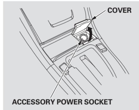
Your car has two accessory power sockets, one is located in the front of the center console, and the other is in the center console compartment. To use an accessory power socket, the ignition switch must be in ACCESSORY (I) or ON (II).
