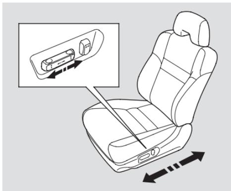
Push the horizontal switch forward or backward to move the seat forward or backward.
