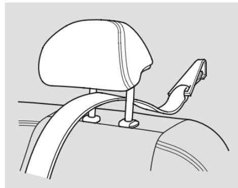
To use either outside anchorage point, lift the rear head restraint, then route the tether strap over the seat-back between the legs of the head restraint.
