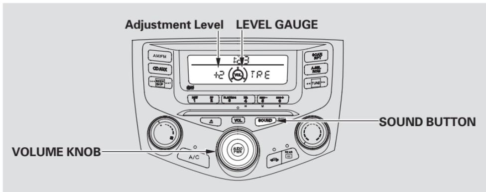
**Treble/Bass** — Use these modes to adjust the tone to your liking. Select TRE or BAS by pressing the SOUND button. Adjust the desired mode by turning the VOLUME knob.
