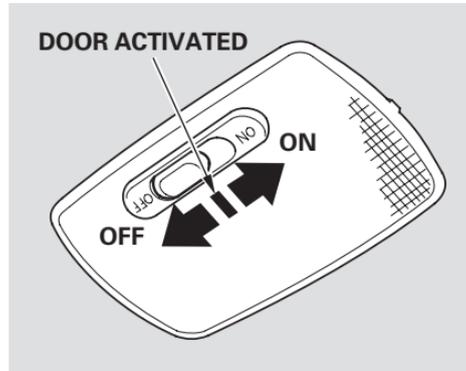
The ceiling light has a three-position switch. In the OFF position, the light does not come on. In the center position, the ceiling light comes on when you open either door.
