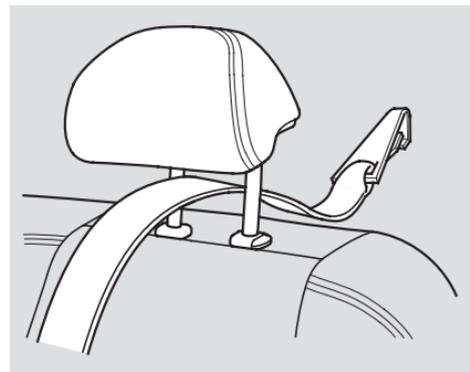
5. Lift the rear head restraint, then route the tether strap over the seat-back between the legs of the head restraint.
