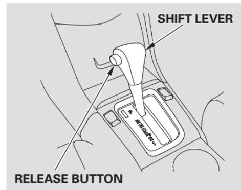
The shift lever has seven positions. It must be in Park or Neutral to start the engine. When you are stopped in D, D3, 2, 1, N or R, press firmly on the brake pedal, and keep your foot off the accelerator pedal.
