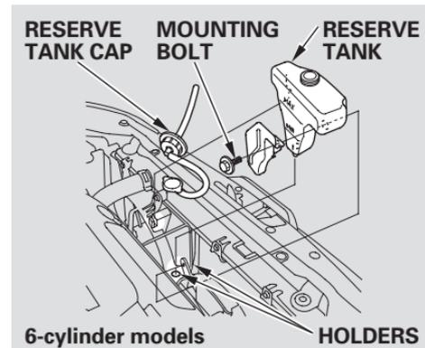
6. Remove the reserve tank from its holder by pulling it straight up. Drain the coolant into an appropriate container, then put the tank back in its holder. Install the mounting bolt securely.
