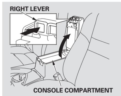
To open the console compartment, pull up on the right lever and lift the armrest.
