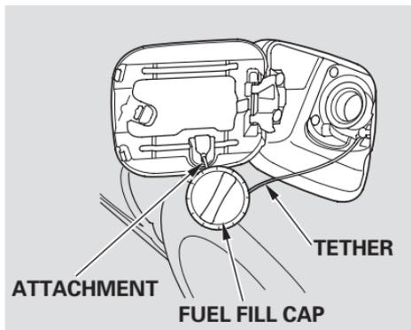
3. Remove the fuel fill cap slowly. You may hear a hissing sound as pressure inside the tank escapes. The fuel fill cap is attached to the fuel filler with a tether. Put the tether end attachment on the fuel fill cap into the slot on the fuel fill door.
