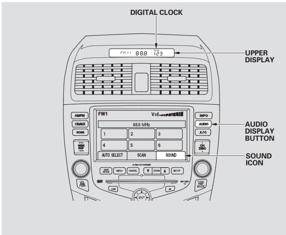
If you want to adjust the sound while the radio/CD is playing, push the AUDIO DISPLAY button, then touch the SOUND icon in the display.
