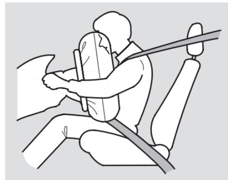
Your car is equipped with dual-stage, dual-threshold airbags to help reduce the chance of airbag-caused injuries.
