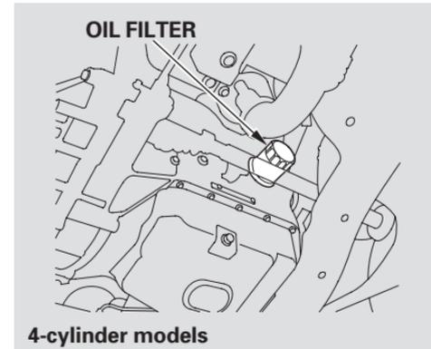
4. Install a new oil filter according to instructions that come with it. Make sure to clean off any dirt and dust on the connecting surface of a new oil filter.
