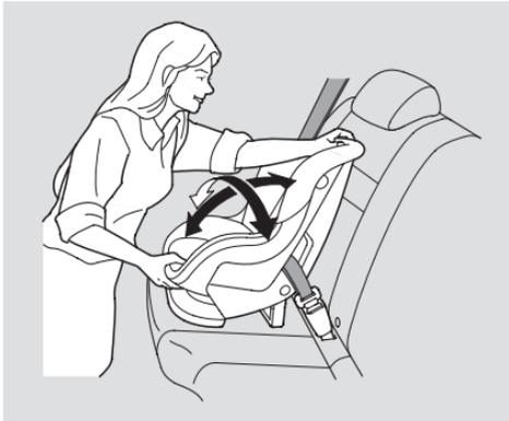
To deactivate the locking mechanism and remove a child seat, unlatch the buckle, unrout the seat belt, and let the belt fully retract.
