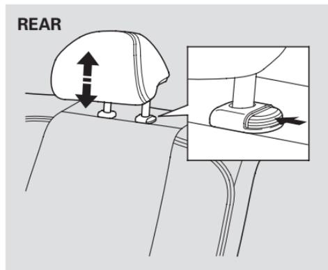
To remove a head restraint for cleaning or repair, pull it up as far as it will go. Push the release button and pull the restraint out of the seat-back.
