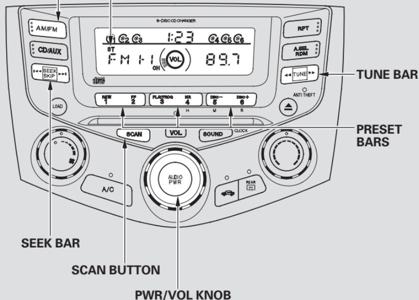
You can use any of five methods to find radio stations on the selected band: TUNE, SEEK, SCAN, AUTO SELECT, and the preset bars.
