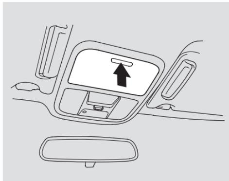
To open the sunglasses holder, push on the front edge. It will unlatch and swing down. To close it, push it until it latches. Make sure the holder is closed while you are driving.
