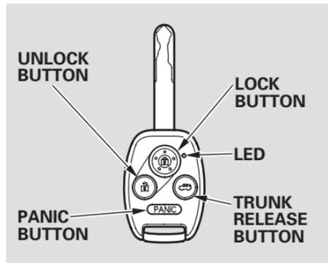
You can lock and unlock your car with the remote transmitter. When you push the LOCK button, both doors lock. The parking lights, side marker lights, and taillights flash once.
