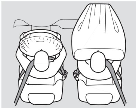
Your car has a Supplemental Restraint System (SRS) with dual-stage, dual-threshold front airbags to help protect the heads and chests of the driver and a front seat passenger during a moderate to severe frontal collision.
