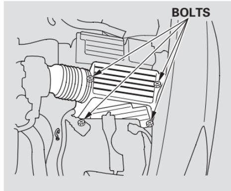
1. Loosen the four bolts, and remove the air cleaner housing cover.
