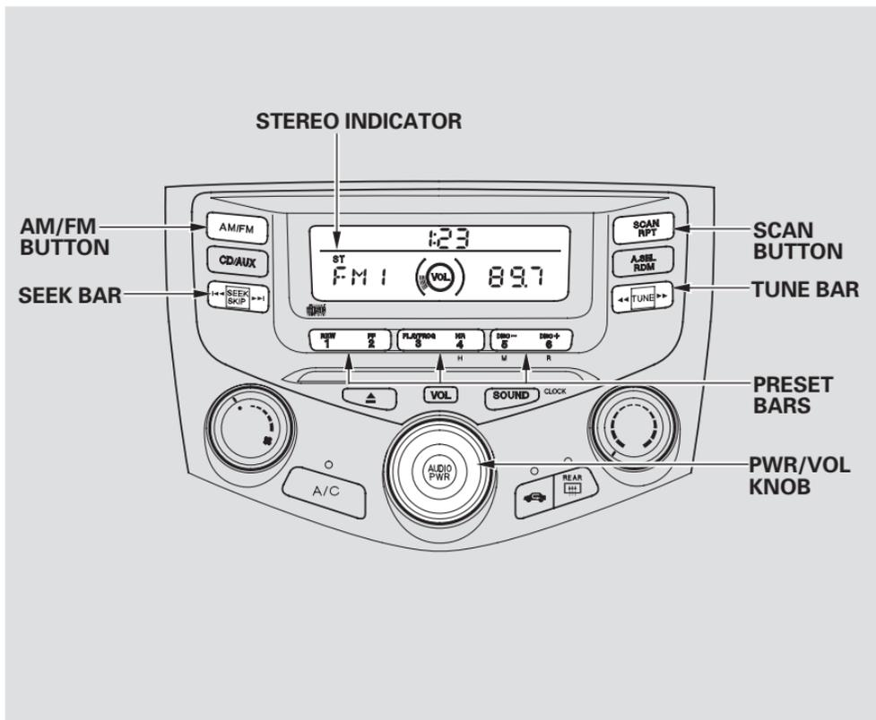
You can use any of five methods to find radio stations on the selected band: TUNE, SEEK, SCAN, AUTO SELECT, and the preset bars.
