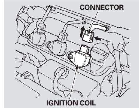
2. Clean off any dirt and oil that has collected around the ignition coil.
