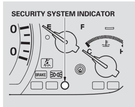
This indicator lights when the security system is set. See page [213](#) for complete information on the security system.
