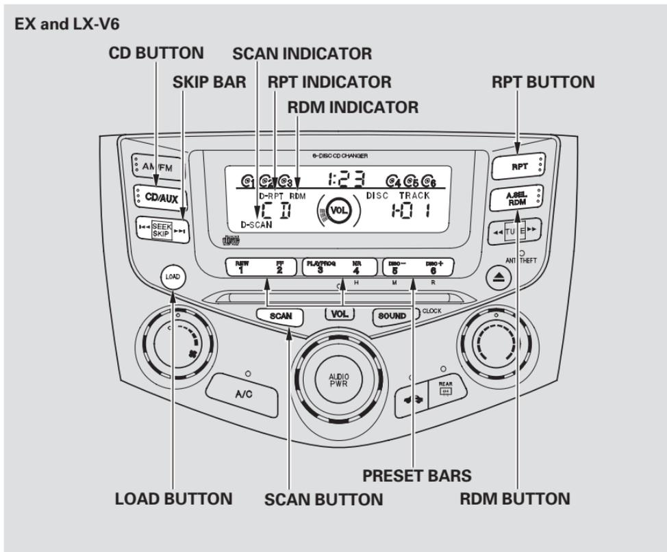
**D-REPEAT** — This feature, when activated, replays all the tracks on the selected disc in the order they are recorded on the CD. To activate the disc repeat feature, select the D-Repeat mode by pressing and holding the RPT button. You will see D-RPT in the display. The system continuously replays the current CD. Press the RPT button again to turn it off. Pressing either side of the SKIP or TUNE bar also turns off the repeat feature.
