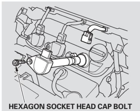
4. Use a wrench to remove the hexagon socket head cap bolt holding the ignition coil. Remove the ignition coil by pulling it straight out.
