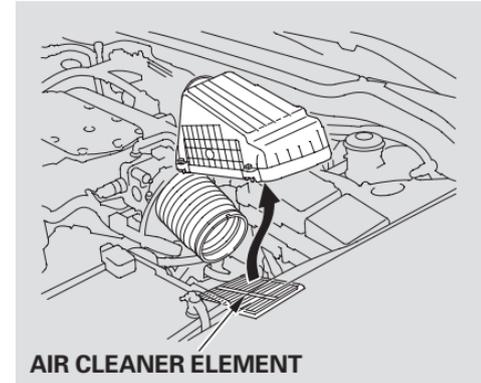
4. Place the new air cleaner element in the air cleaner housing.
