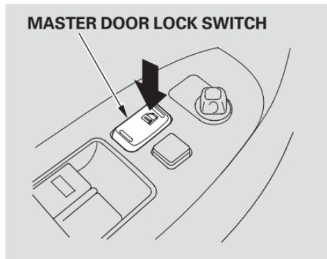
Each door has a master door lock switch. Either switch locks and unlocks both doors. Push the top of the switch to lock both doors; push the bottom to unlock them.
