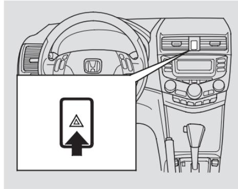
Push the button between the center vents to turn on the hazard warning lights (four-way flashers). This causes all four outside turn signals and both turn indicators in the instrument panel to flash. Use the hazard warning lights if you need to park in a dangerous area near heavy traffic, or if your car is disabled.
