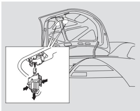
3. Remove the socket from the light assembly by squeezing the tabs on both sides of the socket.
