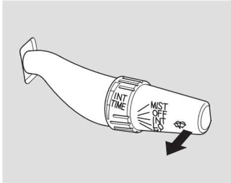
To clean the windshield, pull back on the wiper control lever. The washers spray until you release the lever. The wipers run at low speed while you're pulling the lever, then complete one more sweep of the windshield after you release it.
