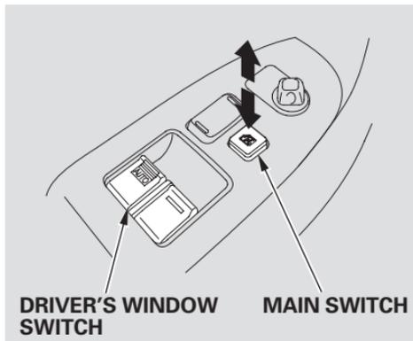
The driver's armrest has a master power window control panel. To open the passenger's window, push down on the switch and hold it down until the window reaches the desired position. To close the window, pull back on the window switch. Release the switch when the window gets to the position you want.
