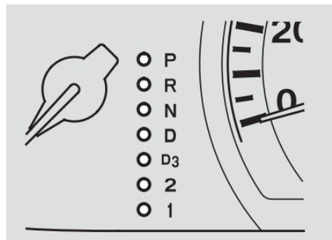
This indicator between the tachometer and speedometer shows which position the shift lever is in.
