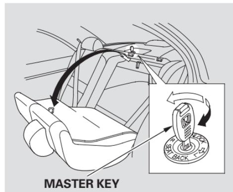
To fold down either side of the seat-back from inside the car, insert the master key in the lock on the rear shelf. To fold down the driver's side, turn the key clockwise, pull down the top of the seat-back, then release the key. To fold down the passenger's side, turn the key counterclockwise and perform the same procedure.
