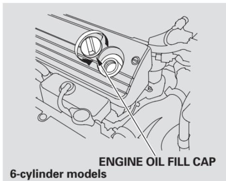
Pour the oil slowly and carefully so you do not spill. Clean up any spills immediately. Spilled oil could damage components in the engine compartment.
