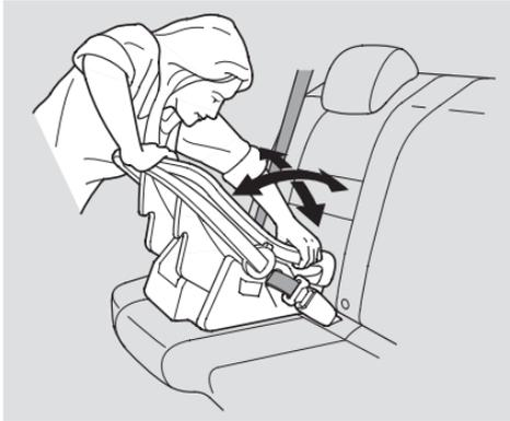
5. Push and pull the child seat forward and from side to side to verify that it is secure enough to stay upright during normal driving maneuvers. If the child seat is not secure, unlatch the buckle, allow it to retract fully, then repeat these steps.
