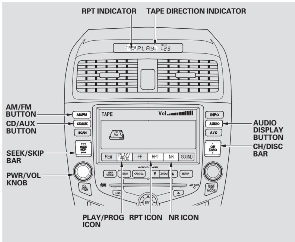
The tape direction indicator will light on the upper display to show you which side of the cassette is playing. The ▲ indicates the side you inserted facing upward is now playing. If you want to play the other side, push the AUDIO DISPLAY button to change to the audio display, and touch the PLAY/PROG icon.
