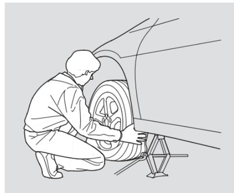
11. Remove the wheel nuts, then remove the flat tire. Temporarily place the flat tire on the ground with the outside surface of the wheel facing up. You could scratch the wheel if you put it face down.
