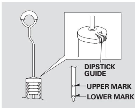
3. Insert the dipstick all the way into the transmission securely as shown in the illustration. Make sure the notch in the rubber cap fits in the dipstick guide and that you push the dipstick in all the way.
