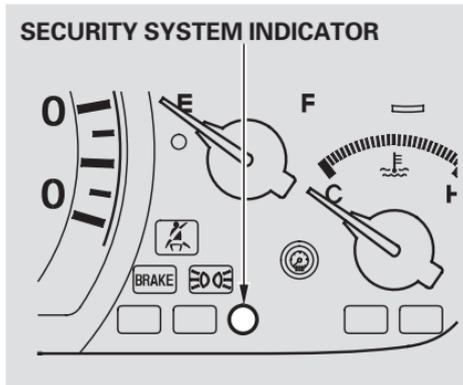
Once the security system is set, opening either door (without using the key or the remote transmitter), the hood, or the trunk will cause it to sound. It also sounds if the radio is removed from the dashboard or the wiring is cut.
