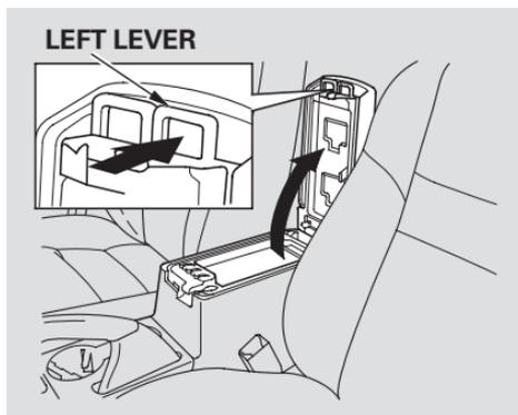
You can put small items in the tray located in the console compartment lid. To use the tray, pull up on the left lever and lift up the armrest.
