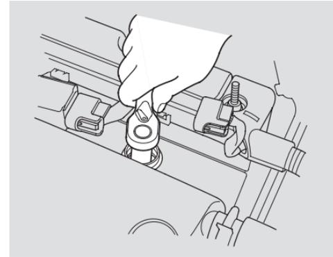
8. Torque the spark plug. (If you do not have a torque wrench, tighten the spark plug two-thirds of a turn after it contacts the cylinder head.)
