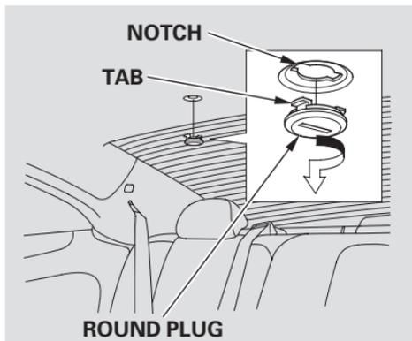
4. To remove the round plug in the center of the headliner, turn the plug by using a screwdriver or coin, then pry it out. Make sure to align the tabs on the round plug to the notches on the ceiling as shown in the illustration.
