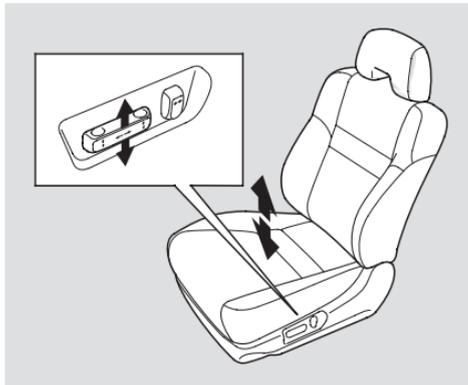
Pull the center of the horizontal switch up to raise the seat. Push it down to lower the seat.
