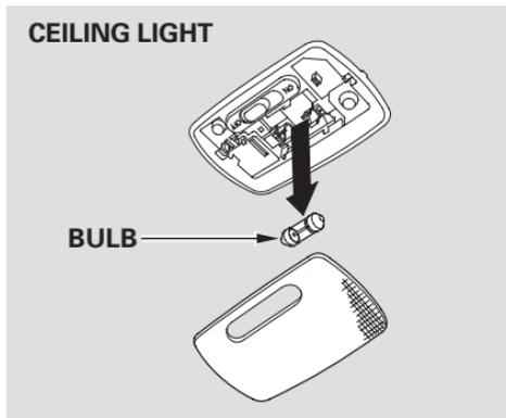
2. Remove the bulb by pulling it straight out of its metal tabs.
