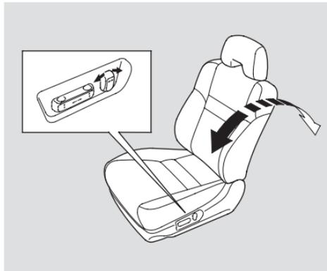
Adjust the seat-back angle by pushing the rear switch in the direction you want to move.
