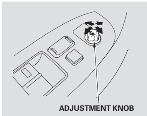
3. Push or pull the adjustment knob in the appropriate direction to move the mirror right, left, up, or down.
