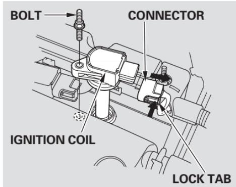
2. Clean up any dirt and oil that have collected around the ignition coils.
