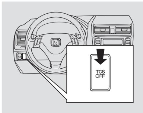
This switch is under the side vent. It lets you turn the Traction Control System on and off. You cannot turn off the TCS while the TCS Activation light is flashing.
