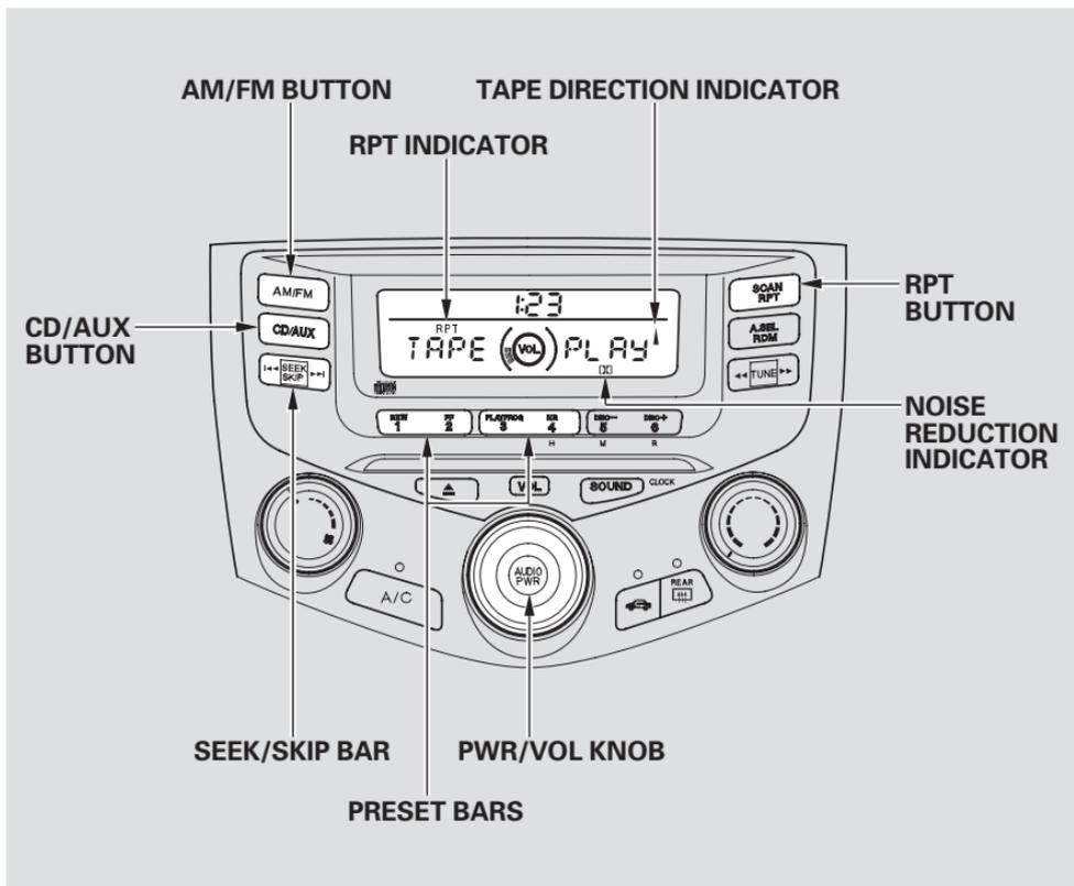
The tape direction indicator will light to show you which side of the cassette is playing. The ▲ indicates the side you inserted facing upward is now playing. If you want to play the other side, press the Preset 3 (PLAY/PROG) side of the preset bar.
