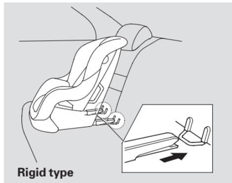
3. Put the child seat in the rear left or right vehicle seat and attach the child seat to the lower anchors according to the child seat maker's instructions.
