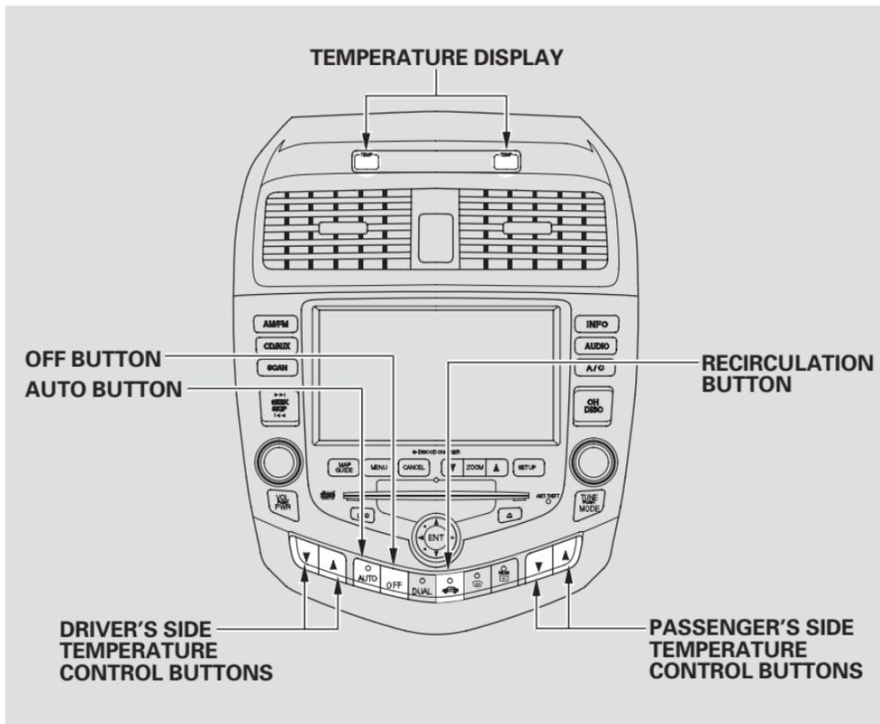
When you set the temperature to its lower limit “ Lo ” or its upper limit “ Hi ”, the system runs at full cooling or heating only. It does not regulate the interior temperature.
