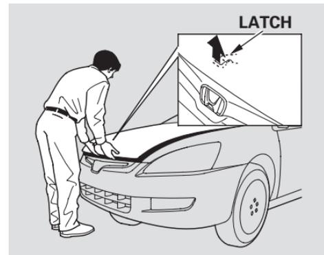
2. Standing in front of the vehicle, reach in between the hood and the front grille with your finger. The hood latch handle is above and to the left of the "H" logo. Push this handle up until it releases the hood. Lift the hood.
