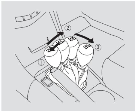
1. With the clutch pedal depressed, move the shift lever to the First/Second gear side of the Neutral gate, then shift to Reverse.
