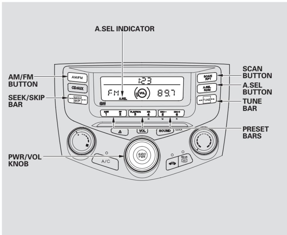
Once a station's frequency is stored, simply press and release the left or right side of the proper preset bar to tune to it.
