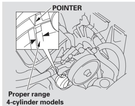
Check the condition of the drive belt. Examine the edges of the belt for cracks or fraying.
