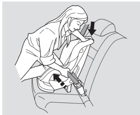
4. After confirming that the belt is locked, grab the shoulder part of the belt near the buckle and pull up to remove any slack from the lap part of the belt. Remember, if the lap part of the belt is not tight, the child seat will not be secure. It may help to put weight on the child seat, or push on the back of the seat, while pulling up on the belt.
