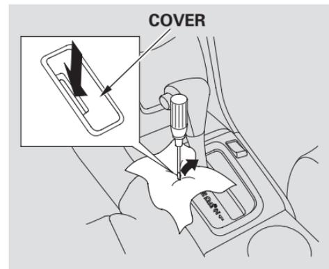
3. Put a cloth on the edge of the Shift Lock Release slot cover next to the shift lever. Use a small flat-tipped screwdriver or small metal plate (neither are included in the tool kit) to remove the cover. Carefully pry off the edge of the cover.
