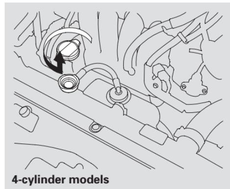
1. Open the hood. Make sure the engine and radiator are cool to the touch.
