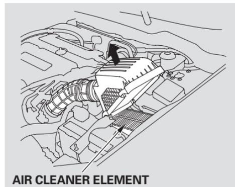
3. Carefully clean the inside of the air cleaner housing with a damp rag.
