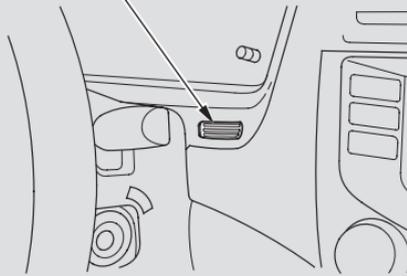
The climate control system has two sensors. A sunlight sensor is located in the top of the dashboard and a temperature sensor is next to the steering column. Do not cover the sensors or spill any liquid on them.
