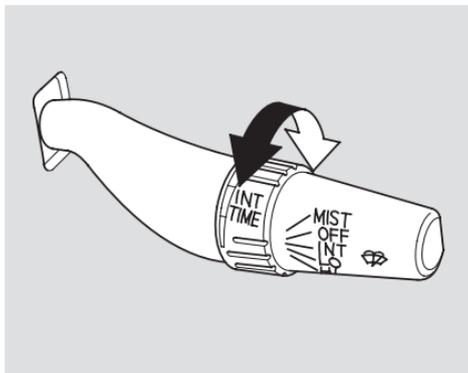
You can vary how often the wipers sweep the windshield by turning the INT TIME ring on the lever.
