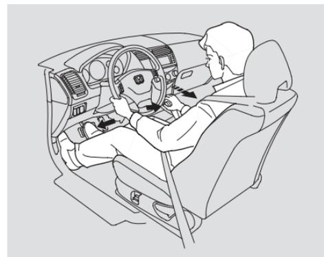
**Reverse (R)** — To shift to Reverse from Park, see the explanation under Park. To shift to Reverse from Neutral, come to a complete stop and then shift. Press the release button before shifting into Reverse from Neutral.
