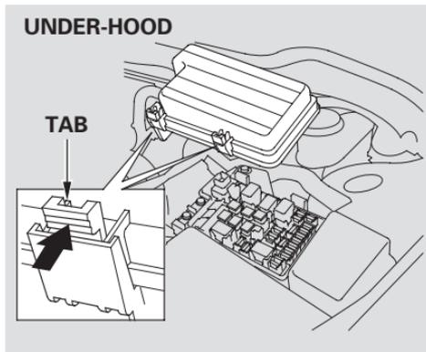
The under-hood fuse box is located near the back of the engine compartment on the driver's side. To open it, push the tabs as shown.
