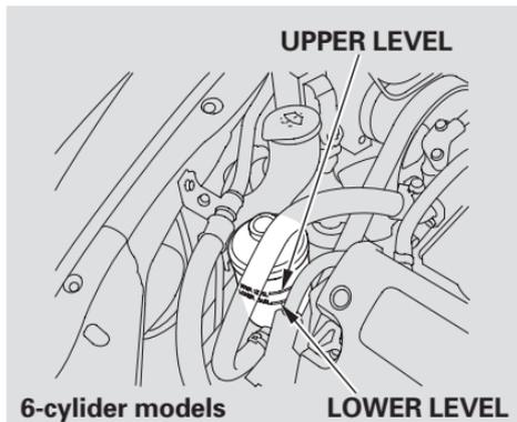
Pour the fluid slowly and carefully so you do not spill. Clean up any spills immediately. Spilled fluid could damage components in the engine compartment.
