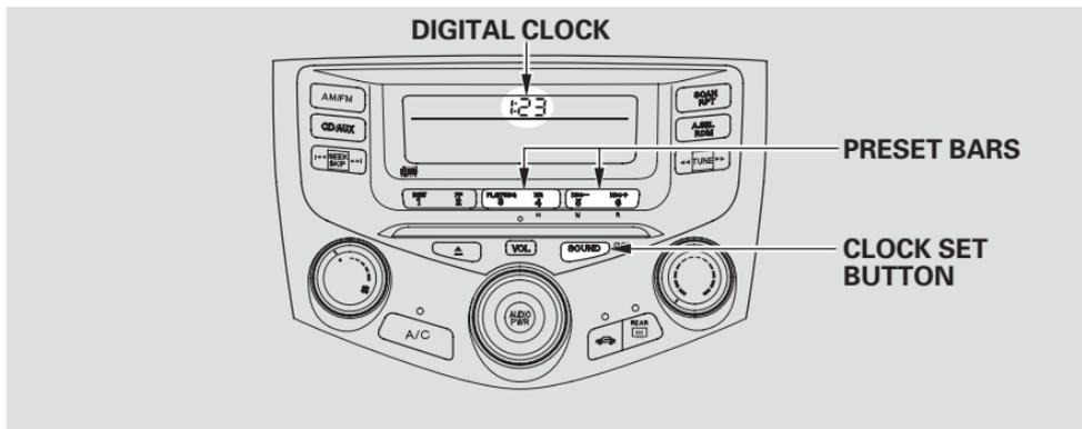
You can use the R (Preset 6) side of the bar to quickly set the time to the nearest hour. Press the Clock Set button (SOUND) until you hear a beep, then press the R (Preset 6) side of the bar. If the displayed time is before the half hour, pressing R sets the clock back to the previous hour. If the displayed time is after the half hour, pressing R sets the clock forward to the beginning of the next hour.
