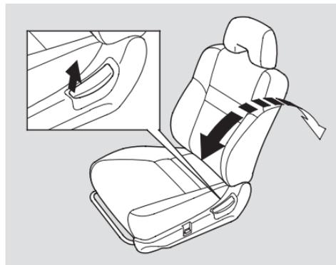
To change the angle of the seat-back, pull up on the lever on the outside of the seat bottom. Move the seat-back to the desired position and release the lever. Let the seat-back latch into the new position.
