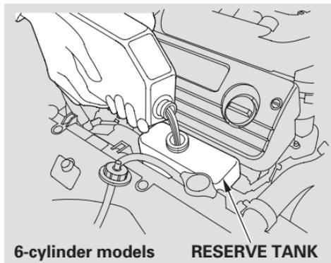
Do not add any rust inhibitors or other additives to your car's cooling system. They may not be compatible with the coolant or engine components.
