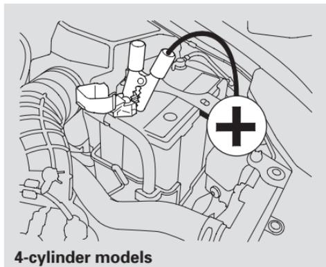
3. Connect one jumper cable to the positive (+) terminal on your Honda's battery. Connect the other end to the positive (+) terminal on the booster battery.
