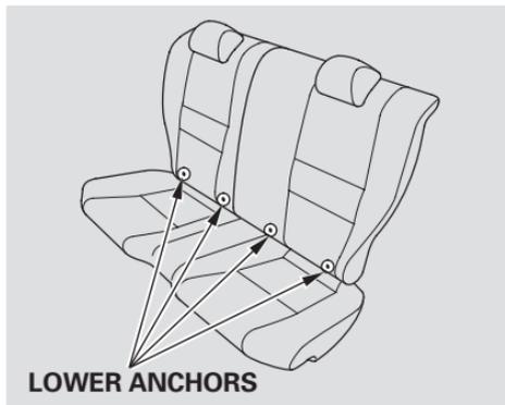
Your car is equipped with LATCH (Lower Anchors and Tethers for Children) at the outer rear seats. The lower anchors are located between the seat-back and seat bottom and are to be used only with a child seat designed for use with LATCH.
