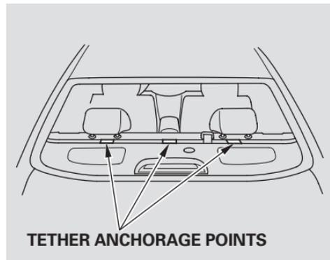
Your car has three tether anchorage points under the rear window for securing a tether-style child seat to the car.
