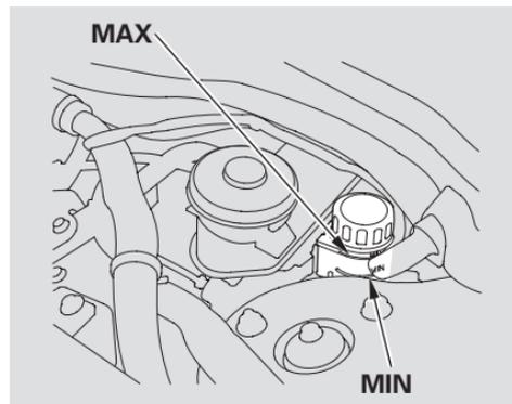
Low fluid level can indicate a leak in the clutch system. Have this system inspected as soon as possible.
