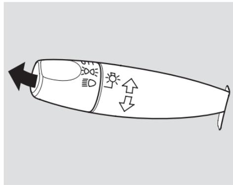
To change from low beams to high beams, push the turn signal lever forward until you hear a click. The blue high beam indicator will light (see page 67). To return to low beams, pull the turn signal lever back.
