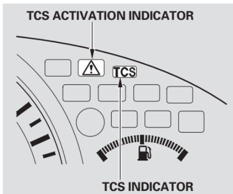
When starting out or driving on a loose or slippery road surface, you may notice that the car does not respond to the accelerator in the same way it does at other times. This is a sign TCS is activating. You will see the TCS Activation indicator light flash.
