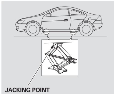
9. Locate the jacking point nearest the tire you need to change. Place the jack under the jacking point. Turn the end bracket clockwise until the top of the jack contacts the jacking point. Make sure the jacking point tab is resting in the jack notch.
