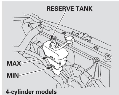
Look at the coolant level in the radiator reserve tank. Make sure it is between the MAX and MIN lines. If it is below the MIN line, see **Adding Engine Coolant** on page 299 for information on adding the proper coolant.
