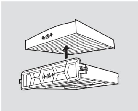
5. Remove the filter from the case.
