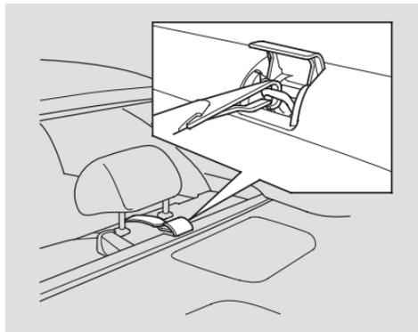
6. Attach the tether strap hook to the tether anchorage point, and tighten the strap according to the child seat maker's instructions. Make sure the strap is not twisted.
