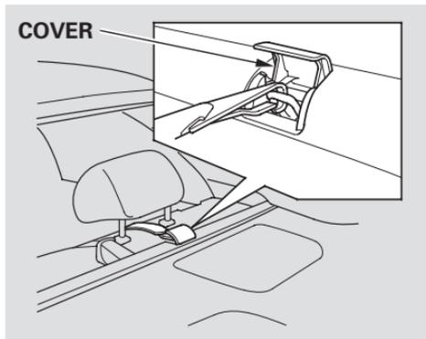
The tether anchorage points are located under plastic covers. Pivot the cover backward to access the anchorage point.
