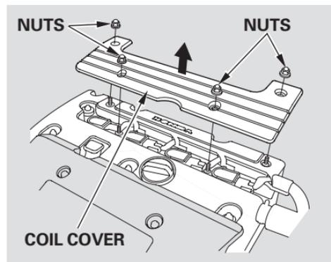
1. Remove the four nuts with a wrench, then remove the coil cover.
