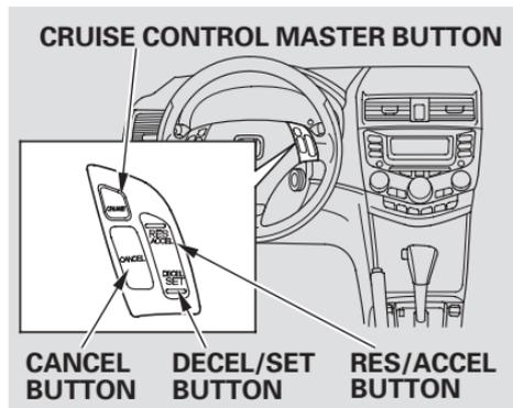
1. Push in the Cruise Control Master Button on the steering wheel. The CRUISE MAIN light on the instrument panel comes on.
