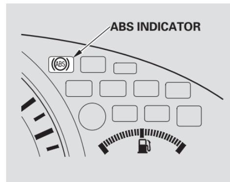
The ABS is self-checking. If anything goes wrong, the ABS indicator on the instrument panel comes on (see page 64). This means the anti-lock function of the braking system has shut down. The brakes still work like a conventional system without anti-lock, providing normal stopping ability. You should have the dealer inspect your car as soon as possible.
