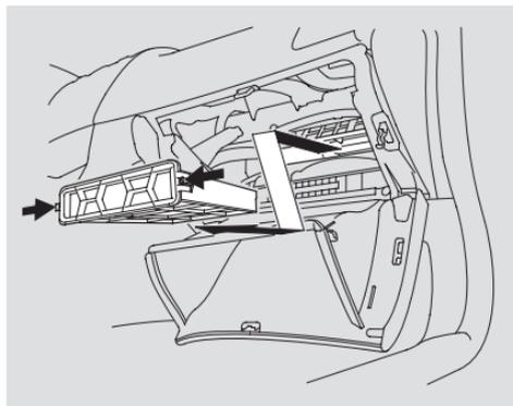
4. Push in the tabs on the corners of the dust and pollen filter case. Pull out the case.
