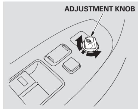
Adjust the outside mirrors with the adjustment knob on the driver's door armrest:
