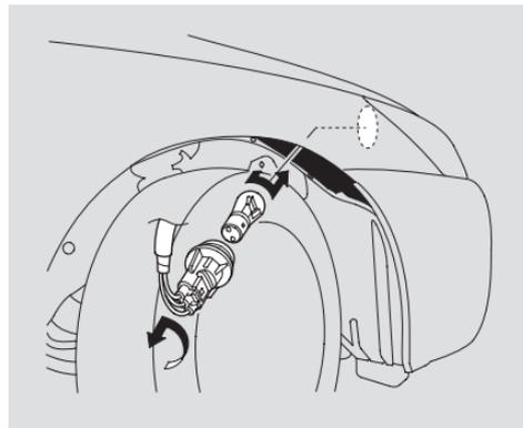
3. Pull the inner fender cover away from the fender and bumper.
