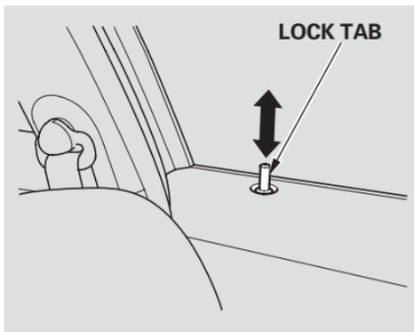
Each door has a lock tab at the top of the door. When you push down the lock tab on the driver's door, both doors lock. Pulling up the lock tab on the driver's door only unlocks that door. The lock tab on the passenger's door only locks and unlocks that door.
