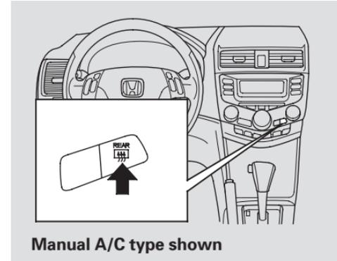
The rear window defogger will clear fog, frost, and thin ice from the window. Push the defogger button to turn it on and off. The light above/in the button lights to show the defogger is on. It also shuts off when you turn off the ignition. You have to turn it on again when you restart the car.
