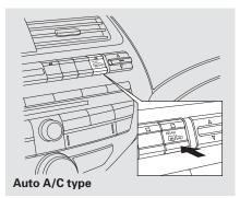
*On vehicles with automatic air conditioning system* The defogger will shut itself off within about 10 to 30 minutes according to the outside temperature (over 32°F, 0°C).
