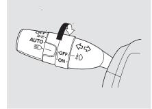
*If equipped* Turn the fog lights on and off by turning the switch next to the headlight switch. You can use the fog lights only when the headlights are on low beam. With the light switch in the AUTO position (if equipped), you can also use the fog lights when the headlights turn on automatically. They will go off when the headlights turn off, or the daytime running lights are on.
