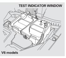
Check the terminals for corrosion (a white or yellowish powder). To remove it, cover the terminals with a solution of baking soda and water. It will bubble up and turn brown. When this stops, wash it off with plain water. Dry off the battery with a cloth or paper towel. Coat the terminals with grease to help prevent future corrosion. If additional battery maintenance is needed, see your dealer or a qualified mechanic.
