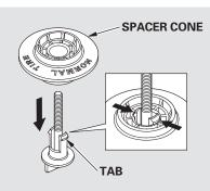
To remove the spacer cone, squeeze the tabs on the wing bolt to disengage it from the center of the spacer cone, then pull the bolt downward.
