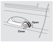
You can open and close the windows and the moonroof (if equipped) with the key in the driver's door lock.
