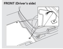
The driver's and right rear passenger's floor mats that came with your vehicle hook over the floor mat anchors. This keeps the floor mats from sliding forward and possibly interfering with the pedals (driver's floor mat) or with the seat weight sensors (right rear floor mat). REAR (Right passenger's side)
