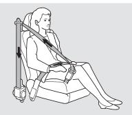
For added protection, the front seat belts are equipped with automatic seat belt tensioners. When activated, the tensioners immediately tighten the belts to help hold the driver and a front passenger in position. The tensioners are designed to activate in any collision severe enough to cause the front airbags to deploy.
