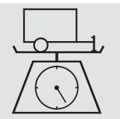
• Total Trailer Weight: The maximum allowable weight of the trailer and everything in or on it must not exceed 1,000 lbs (450 kg). Towing a load that is too heavy can seriously affect your vehicle's handling and performance. It can also damage the engine and drivetrain.
