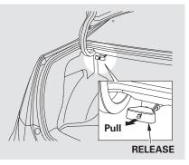
To release the seat-back from inside the trunk, pull the release under the trunk panel. Push the seat-back down from inside the trunk, or pull the seat-back down from inside the vehicle.
