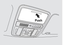
To open the sunglasses holder, push then release the indent. It will unlatch and swing down. To close it, push it until it latches. Make sure the holder is closed while you are driving.
