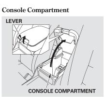
To open the console compartment, pull up on the lever and lift the armrest.
