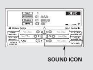
To adjust them, press the AUDIO button, push the interface selector down, and turn the interface knob to SOUND. Then press ENTER on the selector.
