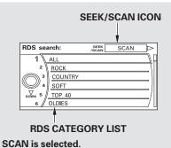
To activate RDS program scan with the interface dial, push the AUDIO button to display the FM radio information on the screen. Push the selector down, and turn the knob to select the RDS SEARCH icon. Press ENTER on the selector. The screen shows you the RDS category list. Turn the knob to the desired RDS category.
