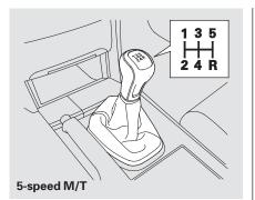
*On models with 5-speed manual transmission, or models with 6-speed manual transmission* The manual transmission is synchronized in all forward gears for smooth operation. It has a lockout so you cannot shift directly from fifth to reverse.
