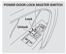
To lock both doors, push the front of the master door lock switch on either door, pull the lock tab rearward on the driver's door, or use the key on the outside lock on the driver's door.
