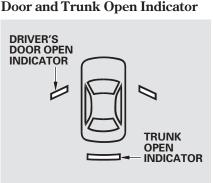
The appropriate indicator comes on if the trunk or either door is not closed tightly.
