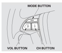
Three controls for the audio system are mounted in the steering wheel hub. These let you control basic functions without removing your hand from the wheel. The VOL button adjusts the volume up ( $\blacktriangle$ ) or down ( $\checkmark$ ). Press the top or bottom of the button, hold it until the desired volume is reached, then release it.
