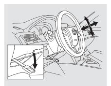
2. Move the steering wheel up or down, and in or out, so it points toward your chest, not toward your face. Make sure you can see the instrument panel gauges and indicators.
