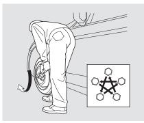
14. Tighten the wheel nuts securely in the same crisscross pattern. Have the wheel nut torque checked at the nearest automotive service facility. Tighten the wheel puts to:
