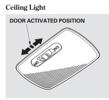
The ceiling light has a three-position switch: ON, Door Activated, and OFF. In the Door Activated (center) position, the light comes on when you:
