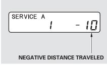
If you do not perform the indicated maintenance, negative distance traveled is displayed and begins to blink after the vehicle has been driven 10 miles (10 km) or more.
