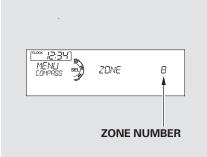
5. Once the correct zone is displayed, press the selector knob. The display then returns to normal.
