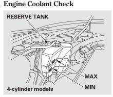
Look at the coolant level in the radiator reserve tank. Make sure it is between the MAX and MIN lines. If it is below the MIN line, see **Adding Engine Coolant** on page 304 for information on adding the proper coolant.
