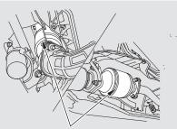
THREE WAY CATALYTIC CONVERTERS 4-cylinder models
