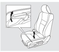
*LX, LX-S and EX models* The height of your driver's seat is adjustable. To raise the seat, repeatedly pull up the lever on the outside of the seat cushion. To lower the seat, push the lever down repeatedly.
