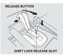
5. Push down on the key while you press the release button on the front of the shift lever and move the shift lever out of Park to neutral. 6. Remove the key from the shift lock release slot, then reinstall the cover. Make sure the notch on the cover is on the right side. Insert the key back into the ignition switch, press the brake pedal, and restart the engine.
