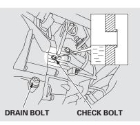
Remove the check bolt and look for transmission fluid coming out of the bolt hole. If a small amount of fluid drips out of the bolt hole, reinstall the check bolt.
