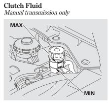
The fluid level should be between the MIN and MAX marks on the side of the reservoir. If it is not, add brake fluid to bring it up to that level. Use the same fluid specified for the brake system.
