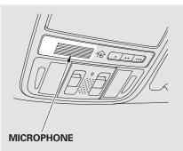
• Air or wind noise from the dashboard and side vents, windows and moonroof may interfere with the microphone. Adjust or close them as necessary.
