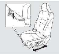
To adjust the seat forward or backward, pull up on the bar under the seat cushion's front edge. Move the seat to the desired position, and release the bar. Try to move the seat to make sure it is locked in position.
