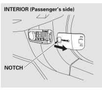
The passenger's side interior fuse box is on the lower passenger's side panel. To remove the fuse box lid, put your finger in the notch on the lid, and pull it upward slightly, then pull it toward you and take it out of its hinges.
