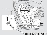
To get into the rear seat on the passenger's side, push downward on the release lever at the base of the seat-back, or pull up on the seat-back adjustment lever. The seat-back will tilt forward and the entire seat will move forward to allow easier entry to the rear seat. After a passenger gets into the rear seat, push the seat-back to the upright position and push the whole seat backwards until it latches. Make sure the seat is fully latched before sitting in it.
