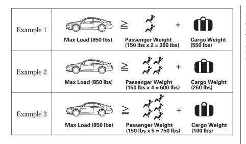
In addition, the total weight of the vehicle, all occupants, accessories, cargo, and trailer tongue load must not exceed the Gross Vehicle Weight Rating (GVWR) or the Gross Axle Weight Rating (GAWR). Both are on a label on the driver's doorjamb.
