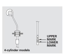
3. Insert the dipstick all the way into the transmission securely as shown in the illustration.
