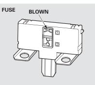
3. Check each of the large fuses in the under-hood fuse box by looking at the wire inside. Removing these fuses requires a Phillips-head screwdriver.
