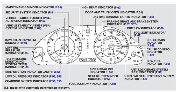
The U.S. instrument panel is shown. Differences for the Canadian models are noted in the text. **\*** : If equipped
