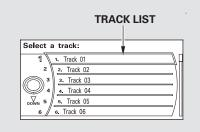
You can also choose a track directly from a track list. Press ENTER on the interface selector, and the track list screen will be shown. If there are no track names, track numbers are displayed. You will see the current track is highlighted. Turn the interface knob to select the desired track, then press ENTER on the interface selector. To exit the track list display, press the AUDIO button, or push the interface selector to the left.
