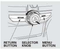
Most audio system functions can be controlled by standard buttons, bars, and knobs. In addition, you can access some functions by using the selector knob on the audio system. The knob turns left and right. Use it to scroll through lists, or to make selections or adjustments to a list or menu item on the display. When you make a selection, push the center of the selector (ENTER) to go to that selection.
