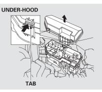
The under-hood fuse box is on the driver's side. To open it, push the tabs as shown.
