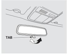
The inside mirror has day and night positions. The night position reduces glare from headlights behind you. Flip the tab on the bottom edge of the mirror to select the day or night position.
