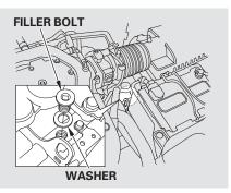
If no fluid comes out, remove the filler bolt. Slowly add Honda Manual Transmission Fluid (MTF) until it starts to run out of the check bolt hole. Pour the fluid into the filler hole slowly and carefully so you do not spill any. Clean up any spills immediately; it could damage components in the engine compartment.
