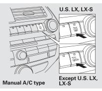
The rear window defogger will clear fog, frost, and thin ice from the window. Push the defogger button to turn it on and off. The indicator in the button comes on to show the defogger is on. It also shuts off when you turn off the ignition switch. You have to turn the defogger on again when you restart the vehicle.
