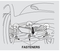
1. *Passenger's side* Remove the three fasteners with a flat-tip screwdriver.
