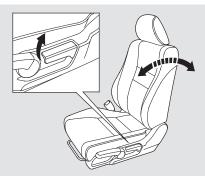
To change the seat-back angle, pull up on the lever on the outside of the seat bottom.
