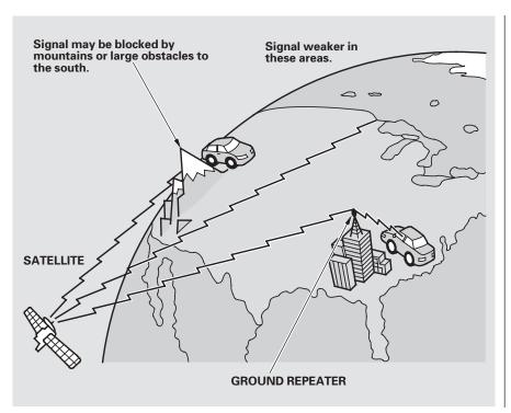
The XM satellites are in orbit over the equator; therefore, objects south of the vehicle may cause satellite reception interruptions. To help compensate for this, ground-based repeaters are placed in major metropolitan areas. Satellite signals are more likely to be blocked by tall buildings and mountains the farther north you travel from the equator.
