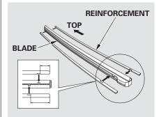
Make sure the two rubber tabs inside the blade fit to each notch of the reinforcement, as shown.
