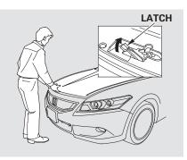
2. Reach in between the hood and the front grille with your fingers. The hood latch handle is above the "H" logo. Push this handle up until it releases the hood. Lift the hood. If the hood latch handle moves stiffly, or if you can open the hood without lifting the handle, the mechanism should be cleaned and lubricated.
