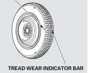
Replace the tire when you can see the tread wear indicator bars. The replacement should be the same size and design tire, mounted on the same wheel. The spare tire is not designed to be mounted on a regular wheel, and the spare wheel is not designed for mounting a regular tire. If you have a flat tire while driving, pull over safely. Drive slowly along the shoulder until you get to an area far away from traffic lanes.
