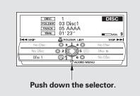
You can select any type of repeat and random modes by using the interface dial. Push the AUDIO button to display the audio information on the screen, then scroll down by pushing down the selector to select the audio menu.
