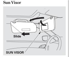
To use the sun visor, pull it down. When using the sun visor for the side window, remove the support rod from the clip, and swing it out. In this position, the sun visor can be adjusted by moving it on its slider. Do not use the extended sun visor over the inside mirror.
