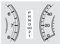
These indicators on the instrument panel show which position the shift lever is in. The "D" indicator comes on for a few seconds when you turn the ignition switch to the ON (II) position. If it flashes while driving (in any shift position), it indicates a possible problem in the transmission.
