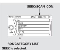
To activate RDS program search with the interface dial, push the AUDIO button to display the FM radio information on the screen. Push the selector down, and turn the knob to select the RDS SEARCH icon. Press ENTER on the selector. The screen shows you the RDS category list. Turn the knob to the desired RDS category.
