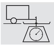
• **Tongue Load:** The weight that the tongue of a fully-loaded trailer puts on the hitch should be approximately 10% of the total trailer weight. Too much tongue load reduces front-tire traction and steering control. Too little tongue load can make the trailer unstable and cause it to sway.
