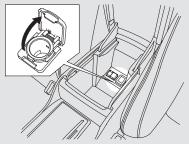
Each socket is intended to supply power for 12 volt DC accessories that are rated 120 watts or less (10 amps). None of the sockets will power an automotive type cigarette lighter element.
