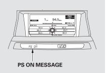
To switch the PS name display function on and off, press and release the TITLE button. With the system on, you will see the "PS ON" message on the center display. If the station you are listening to is an RDS station, the displayed frequency switches to the station name.
