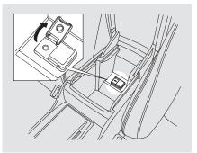
The auxiliary input jack is inside the console compartment. The system will accept auxiliary input from standard audio accessories using a 1/8 inch (3.5 mm) stereo miniplug.
