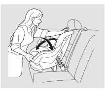
5. Push and pull the child seat forward and from side-to-side to verify that it is secure enough to stay upright during normal driving maneuvers. If the child seat is not secure, unlatch the belt, allow it to retract fully, then repeat these steps. To deactivate the lockable retractor and remove a child seat, unlatch the buckle, unroute the seat belt, and let the belt fully retract.
