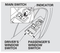
Turn the ignition switch to the ON (II) position to raise or lower either window. To open a window, push the switch down and hold it. Release the switch when you want the window to stop. Pull back on the switch and hold it to close the window.
