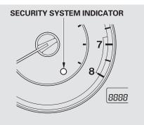
Once the security system is set, opening either door without using the key or the remote transmitter, the hood, or the trunk will cause the alarm to activate. It will also activate if the audio unit is removed from the dashboard or the wiring is cut. With the system set, you can still open the trunk with the remote transmitter without triggering the alarm. The alarm will sound if the trunk lock is forced, or the trunk is opened with the trunk release lever or the emergency trunk opener.
