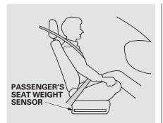
The passenger's advanced front airbag system has weight sensors under the seat. Although Honda does not encourage carrying an infant or small child in front, if the sensors detect the weight of an infant or small child (up to about 65 lbs or 29 kg), the system will automatically turn the passenger's front airbag off. Be aware that objects placed on the passenger's seat can also cause the airbag to be turned off.
