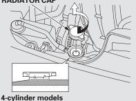
4. The coolant level should be up to the base of the filler neck. Add coolant if it is low
