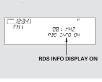
To switch the function between on and off, press and release the TITLE button. With the system on, you will see the "RDS INFO ON" message on the display. If the station you are listening to is an RDS station, the displayed frequency switches to the station name. If the station you are listening to is not an RDS station, the display continues to show the frequency with the RDS information display function on.
