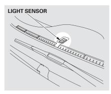
The automatic lighting feature is controlled by a sensor located on top of the dashboard. Do not cover this sensor or spill liquids on it. Instruments and Controls
