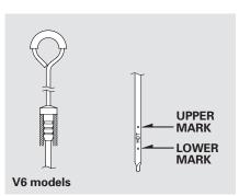
4. Remove the dipstick and check the fluid level. It should be between the upper and lower marks. 5. If the level is below the lower mark, add fluid into the dipstick hole to bring it to the level between the upper and lower marks.
