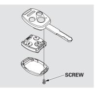
2. Separate the transmitter by prying its middle seam with your fingernail.
