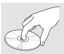
Handle a disc by its edges; never touch either surface. Do not place stabilizer rings or labels on the disc. These, along with contamination from finger prints, liquids, and felttip pens, can cause the disc to not play properly, or possibly jam in the drive.
