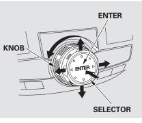
The knob turns left and right. Use it to make selections or adjustments to a list or menu on the screen.
