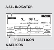
Push the interface selector down to scroll down the screen, highlight A.SEL, then press ENTER on the interface selector. You will see A.SEL on the screen, and the system goes into scan mode for several seconds.
