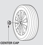
15.Remove the center cap before storing the flat tire in the trunk well.
