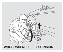
9. Use the extension and the wheel nut wrench as shown to raise the vehicle until the flat tire is off the ground. 10.Remove the wheel nuts, then remove the flat tire. Handle the wheel nuts carefully; they may be hot from driving. Place the flat tire on the ground with the outside surface facing up.
