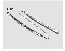
5. Place the top of the wiper blade on the end of the blade assembly, and slide the blade onto the assembly until the tabs are fitted onto the wiper blade.
