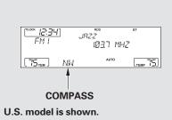
The compass may need to be manually calibrated after exposure to a strong magnetic field. If the compass seems to be continually showing the wrong direction and is not self-calibrating, or the compass display is blinking with the CAL indicator on, do the following.
