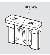
5. Look for a blown wire inside the fuse. If it is blown, replace it with one of the spare fuses of the same rating or lower.
