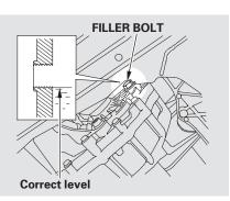
Remove the transmission filler bolt, and carefully feel inside the bolt hole with your finger.
