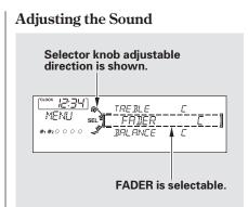
Press the MENU button to display the sound settings. Turn the selector knob to select an appropriate setting: bass, treble, fader, balance, SUBW\* (subwoofer) and SVC (speedsensitive volume compensation). Press the selector knob (ENTER) to enter the setting, then turn the selector knob to adjust the setting.
