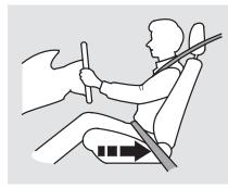
Adjust the driver's seat as far to the rear as possible while allowing you to maintain full control of the vehicle. Have a front passenger adjust their seat as far to the rear as possible.
