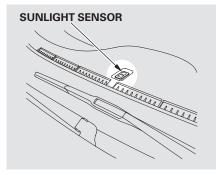
The climate control system has two sensors: a sunlight sensor on top of the dashboard, and a temperature sensor next to the steering column. Do not cover the sensors or spill any liquid on them.
