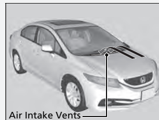
Air Intake Vents
