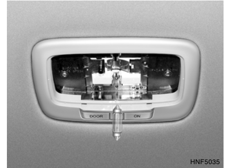
2. Replace with a new bulb.
