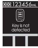
If the smart key is not in the vehicle or is not detected and you push the engine start/stop button, the warning illuminates on the LCD screen for 10 seconds.
