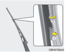
4. Press the button and pull the blade assembly upward.
