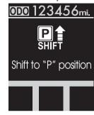
If you push the engine start/stop button with the engine start/stop button ON and the shift lever not in P(Park), the warning illuminates on the LCD screen for 10 seconds to indicate that you should press the engine start/stop button with the shift lever in P(Park) to turn off the engine.
