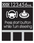
When the steering wheel does not unlock, the warning illuminates for 10 seconds on the LCD screen.
