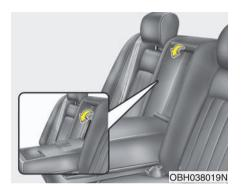
Carrying long/narrow cargo (if equipped) Pull the armrest down using the strap provided on the armrest. Pull the cover down while pushing the release lever down. Additional cargo space is provided to accommodate long/narrow cargo (skis, poles, lumber, etc.) not able to fit properly in the trunk when closed.
