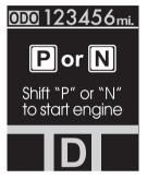
If you try to start the engine with the shift lever not in P(Park) or N(Neutral), the warning illuminates for 10 seconds on the LCD screen.
