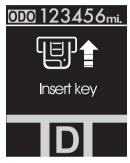
If you push the engine start/stop button while the "Key is not detected" illuminates on the LCD screen, the warning illuminates for 10 seconds.
