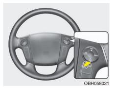
3. Push the SET- switch, and release it at the desired speed. The SET indicator light in the instrument cluster will illuminate. Release the accelerator pedal. The desired speed will automatically be maintained.
