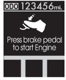
If the engine start/stop button turns to the ACC position twice by pushing the engine start/stop button repeatedly without pressing the brake pedal, the warning illuminates on the LCD screen for 10 seconds to indicate that you should press the brake pedal to start the engine.
