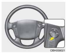
Push the SET- switch, and release it at the desired speed. The SET indicator light, set speed and vehicle to vehicle distance on the LCD screen will illuminate. Release the accelerator pedal. The desired speed will automatically be maintained.
