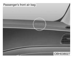
The purpose of the SRS is to provide the vehicle's driver and/or the front passenger with additional protection than that offered by the seat belt system alone in case of a frontal impact of sufficient severity. The SRS uses sensors to gather information about the driver's and front passenger's seat belt usage and impact severity.
