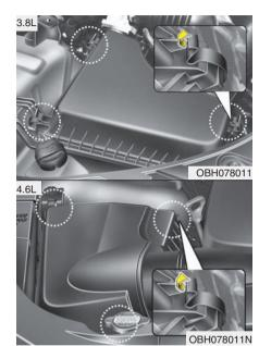
1. Loosen the air cleaner cover attaching clips and open the cover.
