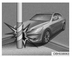
Air bags may not inflate if the vehicle collides with objects such as utility poles or trees, where the point of impact is concentrated to one area and the full force of the impact is not delivered to the sensors. C041100BBH
