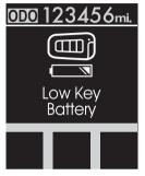
When the smart key in the vehicle discharges, the warning illuminates on the LCD screen for 10 seconds.
