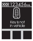
If the smart key is not in the vehicle and if any door is opened or closed with the engine start/stop button in ACC, ON, or START, the warning illuminates on the LCD screen. The chime also sounds for 5 seconds when the smart key is not in the vehicle and any door is closed.
