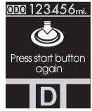
If there is a problem with the engine start/stop button system, the warning illuminates for 10 seconds to indicate that you could start the engine by pressing the engine start/stop button while pressing the brake pedal.
