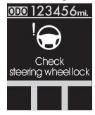
When the steering wheel does not lock, the warning illuminates for 10 seconds on the LCD screen.
