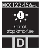
When the stop lamp fuse is disconnected, the warning illuminates for 10 seconds on the LCD screen.
