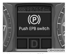
8. After using the EPB emergency release, a warning message will come on. You should operate the EPB switch for the vehicle to return to its normal condition. If the vehicle does not return to normal condition, take your vehicle to an authorized HYUNDAI dealer and have the system checked.
