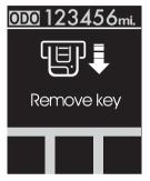
When you turn off the engine with the smart key in the smart key holder, the warning illuminates on the LCD screen for 10 seconds.
