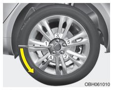
Loosen the wheel lug nuts counterclockwise one turn each in sequence of number, but do not remove any nut until the tire has been raised off the ground.
