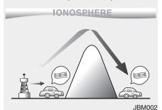
AM broadcasts can be received at greater distances than FM broadcasts. This is because AM radio waves are transmitted at low frequencies. These long, low frequency radio waves can follow the curvature of the earth rather than travelling straight out into the atmosphere. In addition, they curve around obstructions so that they can provide better signal coverage.
