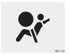
The SRS air bag warning light " on the instrument panel will illuminate for about 6 seconds after the ignition switch is turned to the ON position, after which the SRS air bag warning light " " should go out.
