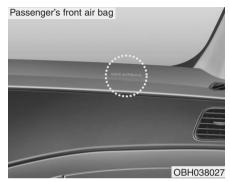
The purpose of the SRS is to provide the vehicle's driver and/or the front passenger with additional protection than that offered by the seat belt system alone in case of a frontal impact of sufficient severity. The SRS uses sensors to gather information about the driver's and front passenger's seat belt usage and impact severity.
