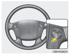
Push the SET- switch, and release it at the desired speed. The SET indicator light in the instrument cluster will illuminate. Release the accelerator pedal. The desired speed will automatically be maintained.
