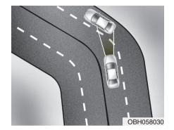
Your vehicle speed can be reduced due to a vehicle in the adjacent lane. Apply the accelerator pedal and select the appropriate set speed. Check to be sure that the road conditions permit safe operation of the smart cruise control.
