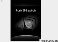
8. After using the EPB emergency release, a warning message will come on. You should operate the EPB switch for the vehicle to return to its normal condition. If the vehicle does not return to normal condition, take your vehicle to an authorized HYUNDAI dealer and have the system checked.
