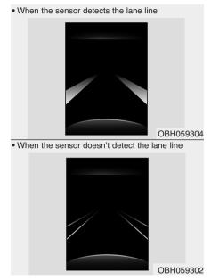
If your vehicle leaves the lane when the LDWS is operating and vehicle speed exceeds 43 mph (70 km/h), the warning operates as follows:
