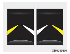
1. Visual warning If you leave the lane, the lane you leave on the LCD display blinks yellow with an 0.8 second interval.
