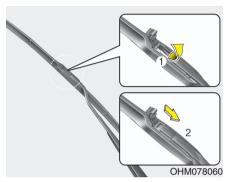
4. Open the cover of the blade. Press the clip behind the wiper arm and remove the blade assembly downward.
