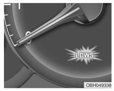
To operate the LDWS, press the switch with the ignition in the ON position. The indicator illuminates on the cluster. To cancel the LDWS, press the switch again.
