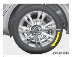
Then position the wrench as shown in the drawing and tighten the wheel nuts. Be sure the socket is seated completely over the nut. Do not stand on the wrench handle or use an extension pipe over the wrench handle. Go around the wheel tightening every other nut until they are all tight. Then double-check each nut for tightness. After changing wheels, have an authorized HYUNDAI dealer tighten the wheel nuts to their proper torque as soon as possible.
