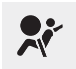
SRS warning light
