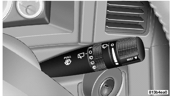
Rear Wiper/Washer Switch
