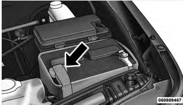
Positive Battery Post
