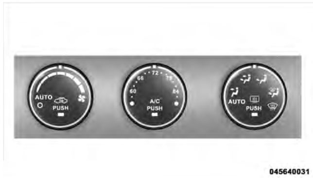
Automatic Temperature Control
