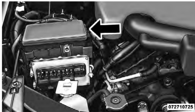
Totally Integrated Power Module
