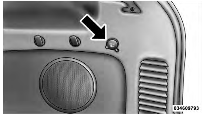
Rear Power Outlet
