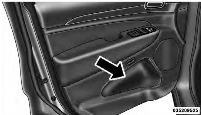
Door Panel Storage
