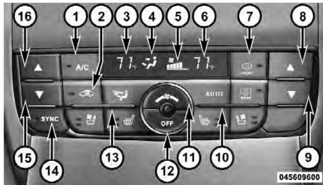
Automatic Temperature Control (ATC) Panel
