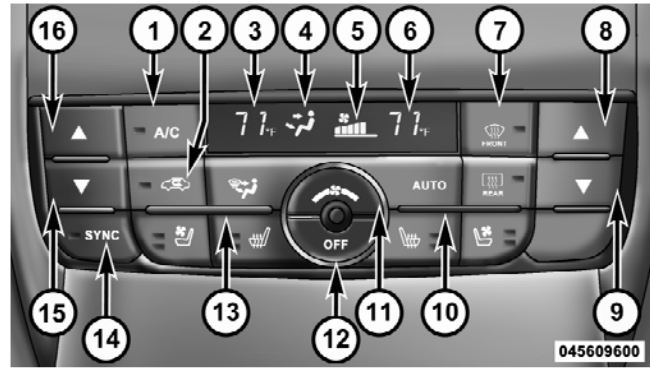
Automatic Temperature Control (ATC) Panel
