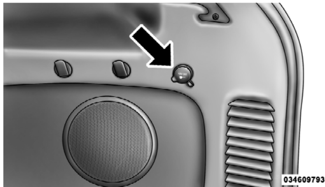
Rear Power Outlet
