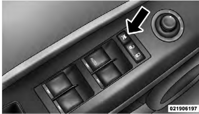
Window Lockout Switch
