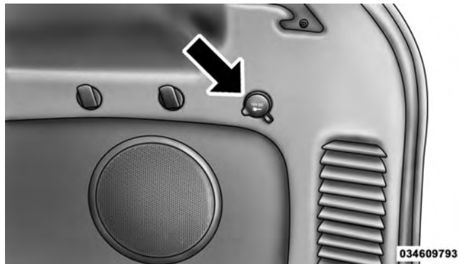
Rear Power Outlet
