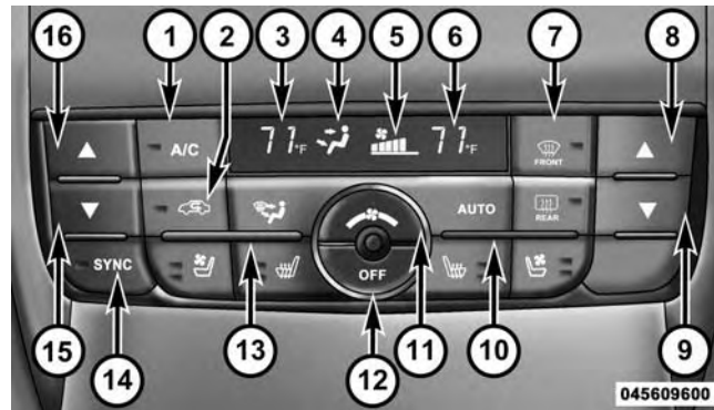
Automatic Temperature Control (ATC) Panel
