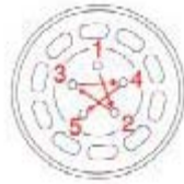
Correct tightening order for wheel bolts
