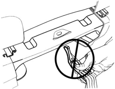
**If the tether strap is clipped incorrectly (as shown) the child safety seat may not be retained properly in the event of a collision.**
