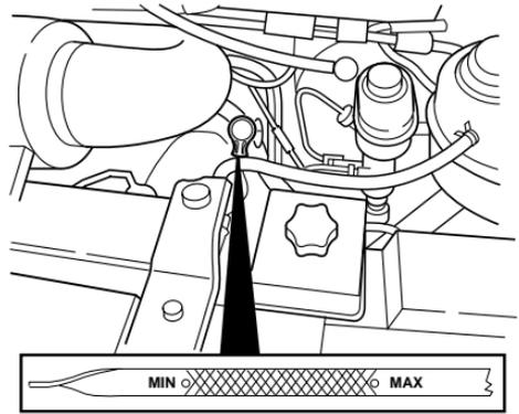
6. Wipe the indicator clean. Insert the indicator fully, then remove it again.
