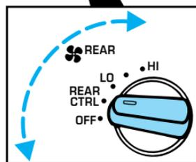
The fan speed of the auxiliary unit can be controlled either by the front seat using the front auxiliary control or by the rear seat passengers using the rear auxiliary control, but not both. To control the auxiliary unit using the rear control, the front control must be in the REAR position.
