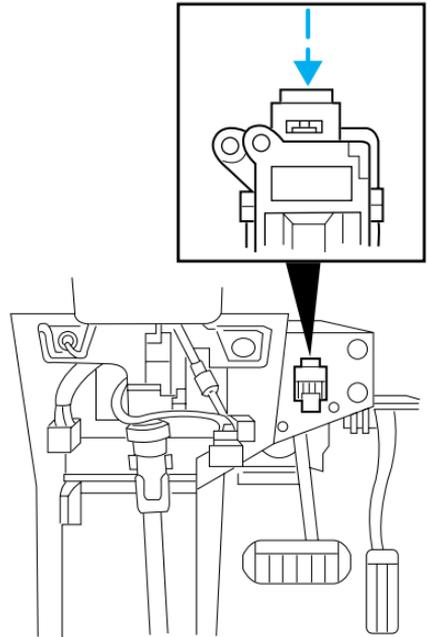
Use the following procedure to reset the fuel pump shut-off switch.
