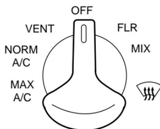
The air conditioning compressor will operate in all modes except VENT and FLR. However, the air conditioning will only function if the outside temperature is about 10°C (50°F) or higher.
