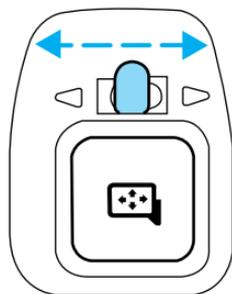
2. Move the control in the direction you wish to tilt the mirror.
