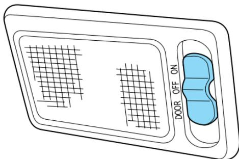
When the control is in the OFF position, it will not illuminate when you open the doors or fully rotate the headlamp control.
