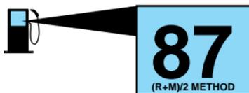
Do not be concerned if your engine sometimes knocks lightly. However, if it knocks heavily under most driving conditions while you are using fuel with the recommended octane rating, see your dealer or a qualified service technician to prevent any engine damage.
