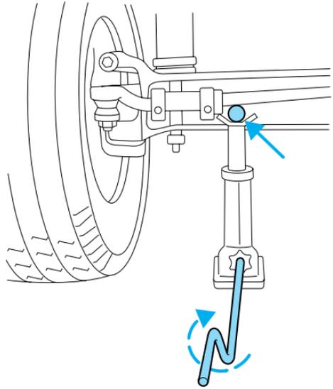
3. Turn the jack handle clockwise until the wheel is completely off the ground.
