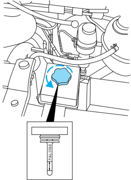
Check the fluid level when it is at ambient temperature, 20° – 80° F (-7° – 25° C):
