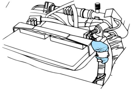
3. Disconnect the primary battery ground cable.
