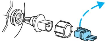
6. Remove the bulb retaining ring by rotating it counterclockwise (when viewed from the rear) to free it from the bulb socket, and slide the ring off the plastic base. Keep the ring to retain the new bulb.
