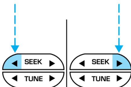
To set the minute, press and hold the CLK control and press TUNE:
