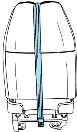
4. Grasp the tether strap and position it to the seat pedestal as shown.
