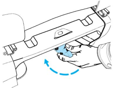
6. Clip the tether strap to the seat pedestal as shown.
