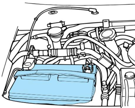
However, for severe usage or in high temperature climates, check the battery electrolyte level. Refer to the Scheduled Maintenance Guide for the service interval schedules.
