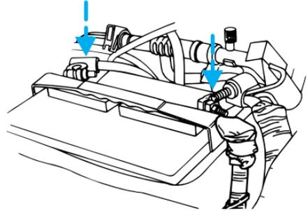
3. Unwrap the secondary positive cable and reconnect to the primary battery terminal.
