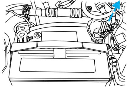
2. Wrap the secondary positive cable with a non-conductive material to insulate.
