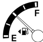
the gauge first indicates empty, there is a small amount of reserve fuel in the tank. When refueling the vehicle from an empty indication, the amount of fuel that can be added will be less than the advertised capacity due to the reserve fuel.
