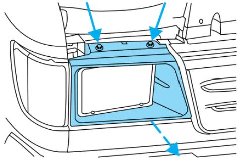
4. Remove the four headlamp bulb retaining screws.
