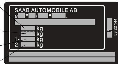
Permissible load (in addition to driver) = GVW minus curb weight
