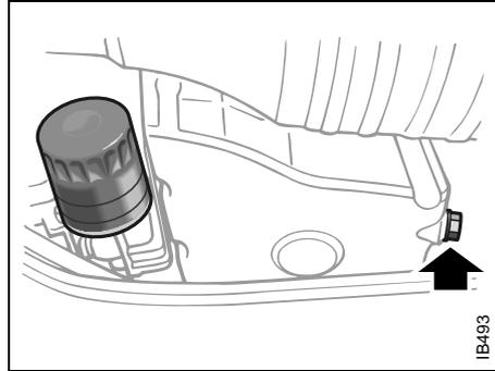
*Drain plug and oil filter*
