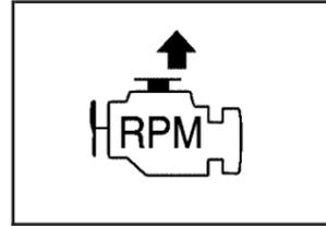
If your vehicle has this feature, the manual high idle switch is located on the instrument panel.
