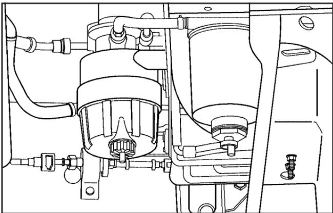
5. For van models, in order to drain the water from the system, you will have to repeat the operation for the primary and secondary fuel filters.
