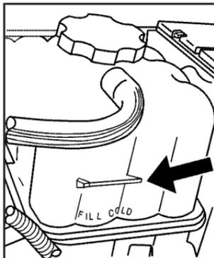
The coolant surge tank is located in the engine compartment on the passenger's side of the vehicle. See *Engine Compartment Overview* on page 5-18 for more information on its location.
