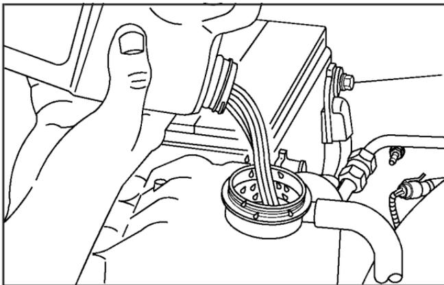
6. Then fill the coolant surge tank with the proper mixture, to slightly above the fill mark.
