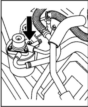
5. Open the fuel filter vent valve by turning the screw counterclockwise several full turns. The vent valve is located on top of the fuel filter housing.
