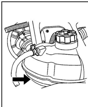
The coolant recovery tank is located near the center of the engine compartment. See *Engine Compartment Overview* on page 5-18 for more information on its location.
