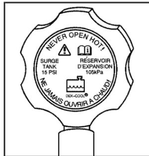
The surge tank pressure cap must be tightly installed.
