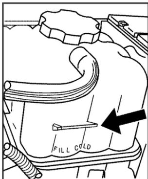
The coolant level should be at or above the FULL COLD mark. If it isn't, you may have a leak at the pressure cap or in the radiator hoses, heater hoses, radiator, water pump or somewhere else in the cooling system.
