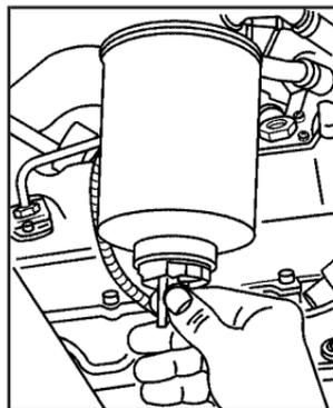
4. For pickup models, open the drain valve by turning it two to three turns. When fuel empties from the valve, all the water has been drained. Close the valve hand tight. To help remove all the water, press the priming pump several times.
