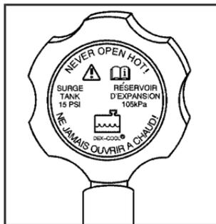
Park the vehicle on a level surface. You can remove the coolant surge tank pressure cap when the cooling system, including the coolant surge tank pressure cap and upper radiator hose, is no longer hot.
