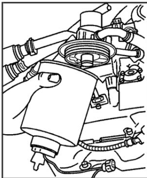
2. Unplug the water sensor wire connected to the fuel filter and unscrew the filter element.
