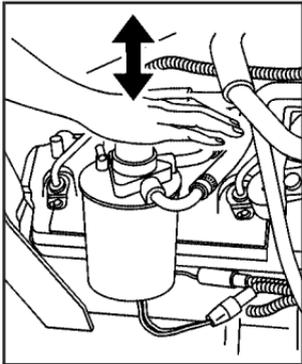
6. Repeatedly push down on the fuel filter priming pump with the palm of your hand. The pump is located on top of the fuel filter housing. Let the pump return upward between pushes.
