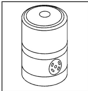
The air cleaner/filter assembly may have an air cleaner/filter restriction indicator that lets you know when the engine air cleaner/filter is dirty and needs to be serviced.
