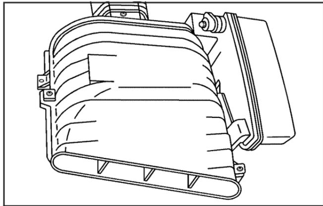
The air cleaner/filter assembly is located at the front of the engine compartment.
