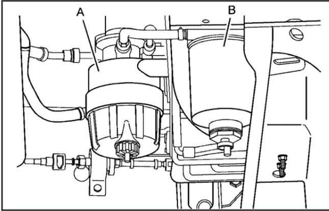
2. Unplug the water sensor wire connected to the fuel filter (lowest wire) and unscrew the filter's cap.
