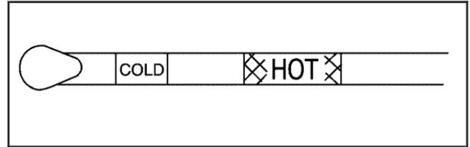
Check both sides of the dipstick, and read the lower level. The fluid level must be in the COLD area for a cold check or in the HOT or cross-hatched area for a hot check. Be sure to keep the dipstick pointed down to get an accurate reading.
