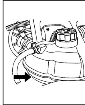
When the engine is cold, the coolant level should be at or above the COLD FILL mark.
